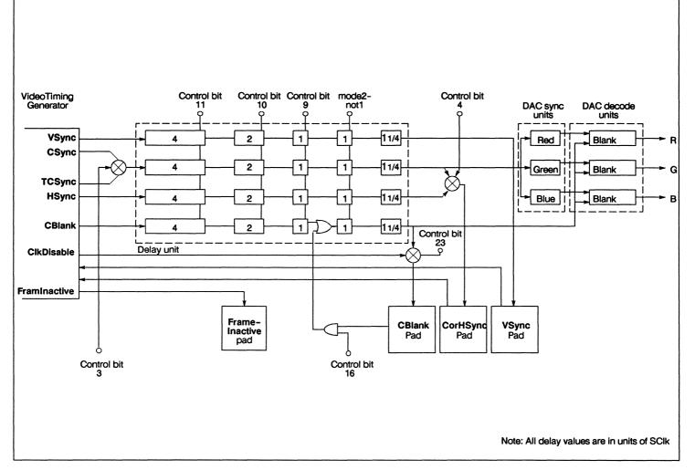
Figure 6.18 Digital and analogue syncing and blanking system 110
