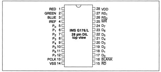
Figure 4.20 IMS G176/L 28 pin dual-in line package pinout
