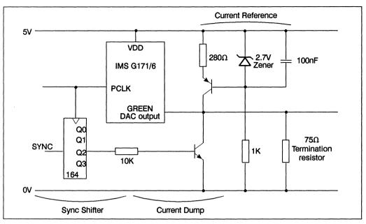
Figure 10.9 Adding an external sync pulse circuit to the G171/6.
