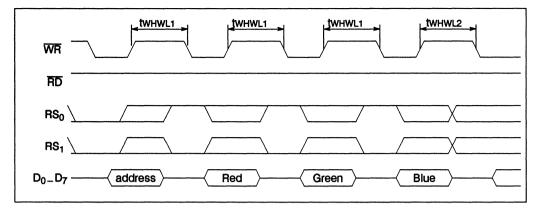
Figure 5.12 Colour value write followed by any write
