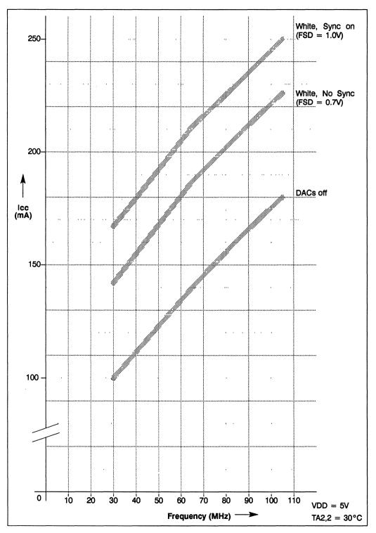
Figure 6.11 Icc (typical) versus pixel frequency
