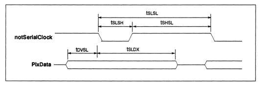
Figure 6.7 Pixel port signals in mode 1
