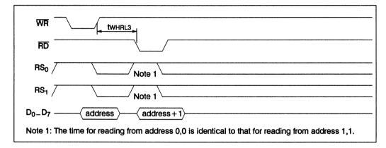
Figure 3.12 Write and read back address register (read mode)
