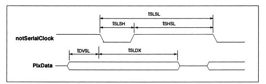
Figure 8.5 Pixel port timing diagram
