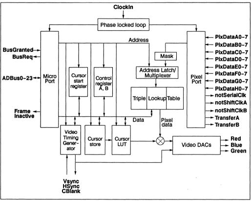
Figure 8.1 IMS G364 Block Diagram
