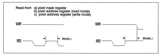
Figure 3.7 Read from register followed by any access
