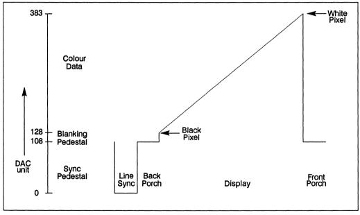
Figure 8.15 DAC output levels
