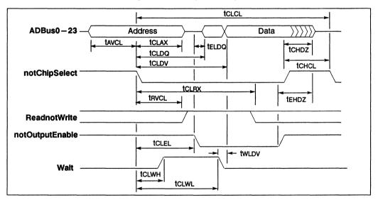
Figure 7.3 Micro port read cycle
