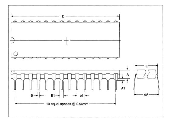
Figure 3.21 28 pin plastic dual-in-line package dimensions
