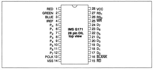
Figure 3.20 IMS G171 28 pin dual-in line package pinout
