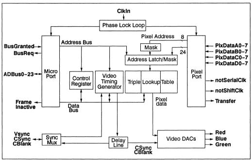
Figure 6.1 IMS G300 Block Diagram
