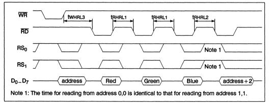
Figure 5.14 Read colour value then the address register (read mode)
