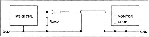
Figure 4.16 Buffered signal
