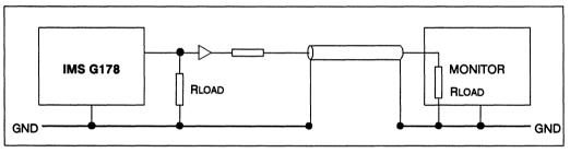
Figure 5.16 Buffered signal
