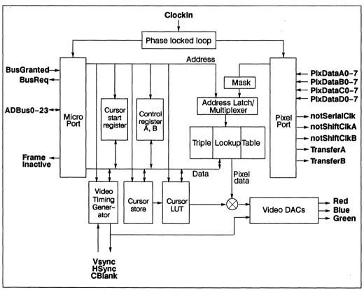
Figure 7.1 IMS G332 Block Diagram
