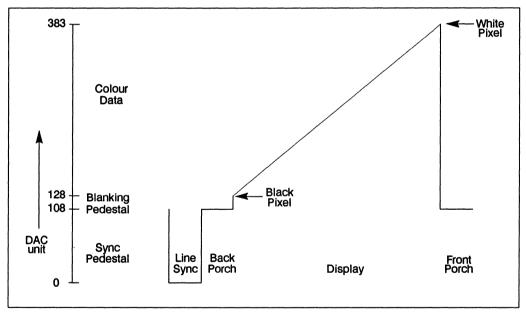
Figure 7.15 DAC output levels
