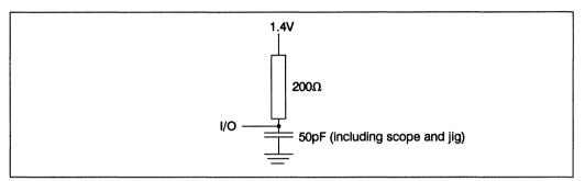
Figure 5.3 Digital output load
