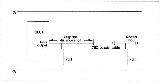
Figure 10.2 Double termination of DAC output.
