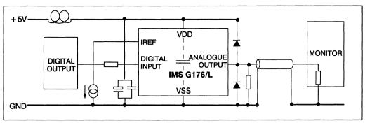
Figure 4.19 Suggested circuit using DIL package
