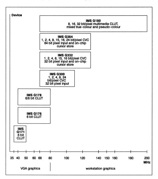
The INMOS family of colour look-up tables provide the analogue output stages for colour graphic systems. The device consists of a high-speed random access store or look-up table, three DACs, a pixel word mask and a microprocessor interface.
