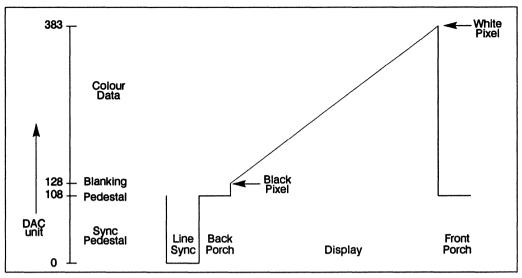
Figure 6.27 DAC output levels
