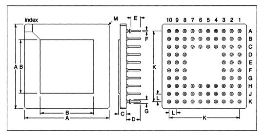
Figure 6.33 84 pin grid array package dimensions
