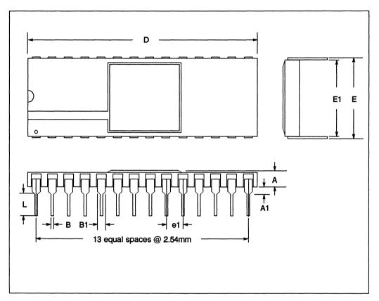
Figure 3.22 28 pin ceramic dual-in-line package dimensions
