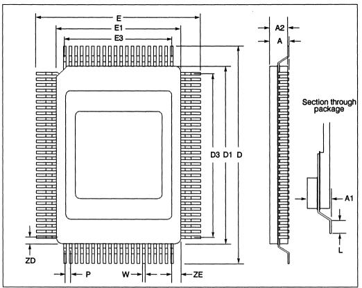
Figure 6.35 100 pin ceramic quad flatpack package dimensions
