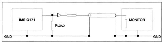
Figure 3.15 Buffered signal
