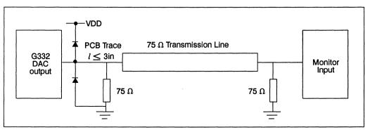
Figure 7.17 DAC output loading
