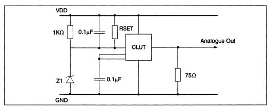
A typical recommended circuit for the voltage reference is shown in figure 10.8.
