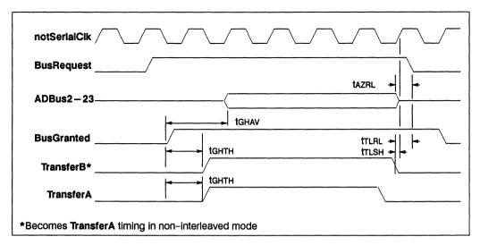
Figure 7.4 Micro port DMA and data transfer timings
