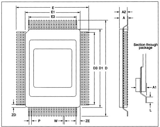
Figure 7.19 100 pin ceramic quad flatpack package dimensions
