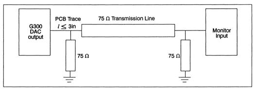
Figure 6.29 DAC output loading
