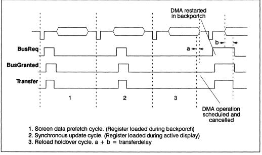
Figure 6.21 Data transfer operational behaviour
