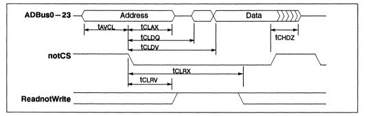
Figure 6.4 Micro port read cycle
