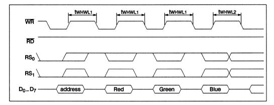
Figure 3.11 Colour value write followed by any write
