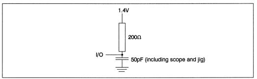
Figure 3.3 Digital output load
