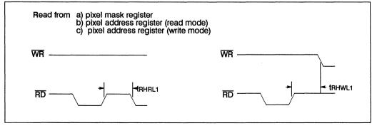
Figure 5.8 Read from register followed by any access
