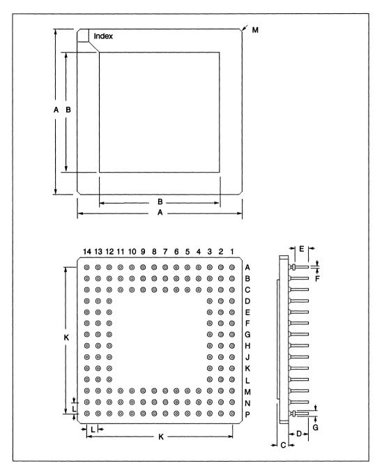
Figure 8.19 132 pin grid array package dimensions
