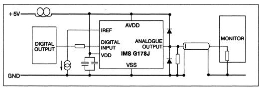
Figure 5.18 Suggested circuit using PLCC package
