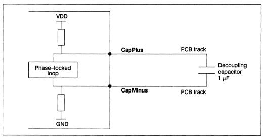
Figure 6.30 Recommended PLL decoupling
