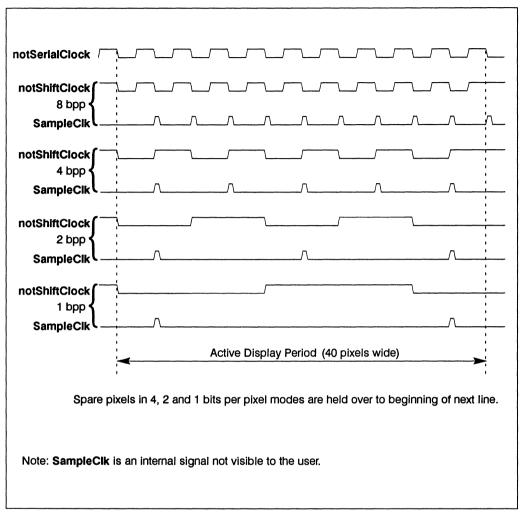
Figure 6.24 Relationship between Serial and Shift Clocks to pixel data in various bits per pixel modes
