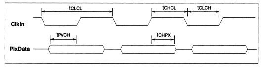
Figure 6.8 Pixel port signals in mode 2
