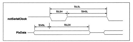
Figure 7.5 Pixel port timing diagram
