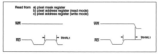
Figure 4.8 Read from register followed by any access
