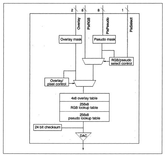
Figure 9.1 Colour Channel Architecture
