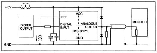
Figure 3.17 Circuit incorporating suggested design features
