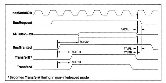
Figure 8.4 Micro port DMA and data transfer timings
