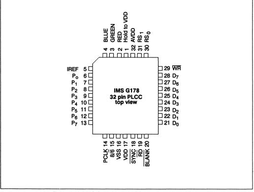
Figure 5.19 IMS G178 32 pin PLCC J-bend package pinout
