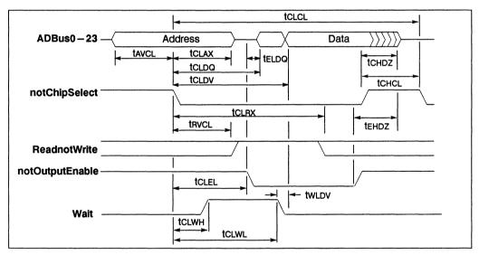
Figure 8.3 Micro port read cycle
