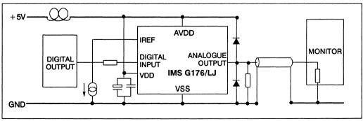
Figure 4.18 Suggested circuit using PLCC package
