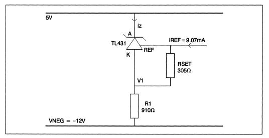
Figure 10.5 Current reference based on the TL431 voltage reference.
