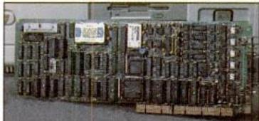
National Instruments' EISA-A2000 data-acquisition card accepts four inputs.
