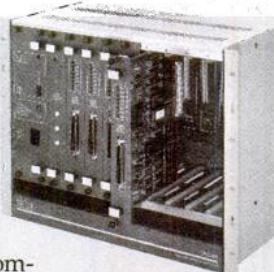
DB-25, RJ-11, or telephone punch down block. We even provide optional INCS-64 compatible line drivers and multiplexers, which extend your transmission distances up to 3,000 feet and beyond.
