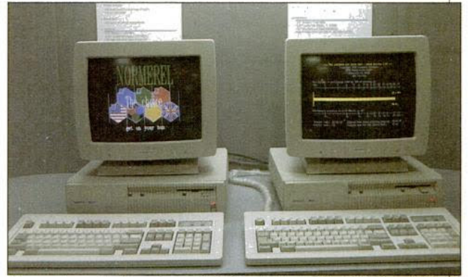
Normerel unveiled a series of MCA PCs, including the NS 50 and NS 70. The high-end NS 70 comes with a 70-megabyte hard disk.
