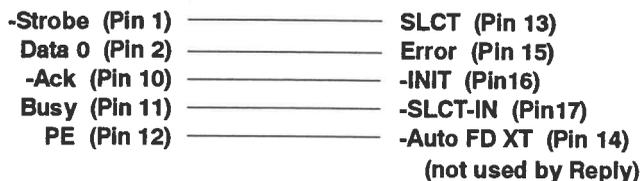
Figure 5-10 Parallel Loop Back Connector
