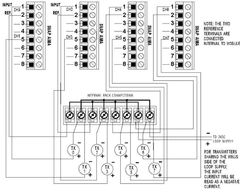
**Typical Analog Input (Current: Positive) Using Terminal Strip**
