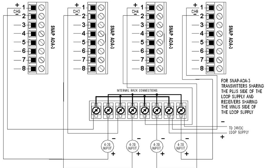
**Typical Analog Output (4-20 mA Current: Sinking) Using Terminal Strip**
