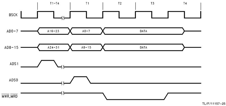
**Note:** In 32-bit address mode, ADS1 is at TRI-STATE after the first T1-T4 states; thus, a 4.7k pull-down resistor is required for 32-bit address.
