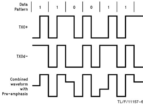
The signal with pre-emphasis shown above is generated by resistively combining TXO+ and TXOd-. This signal along with its complement is passed to the transmit filter.
