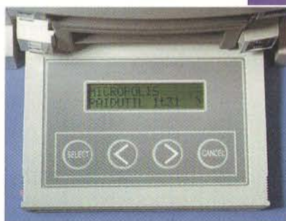
The Raidion LTX stacks up to eight high-capacity SCSI drives into a RAID tower that the host system considers to be a single SCSI device. The four-drive stack shown at right stores 5.2 GB of data in a RAID 5 configuration. The fifth module on the stack bottom holds the Gandiva controller, which has a slide-out control panel (above).
