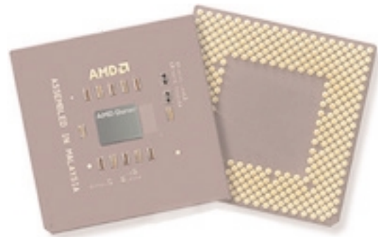
Figure 1. This photograph shows Duron in flip-chip packaging. The top of the ceramic package has a number of small jumper pads, which select default operating parameters such as processor core voltage and clock frequency multiplier.
