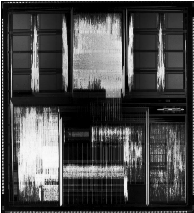
Figure 4. The Nx586 die includes 3.5 million transistors and is built using 0.5-micron CMOS. In a fit of paranoia, NexGen would not reveal the die size or provide a die overlay.
