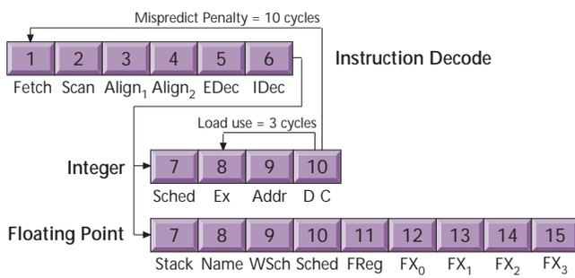
Figure 2. K7's deep 10-stage pipeline enables a high clock rate, but it pays a serious penalty on mispredicted branches.
