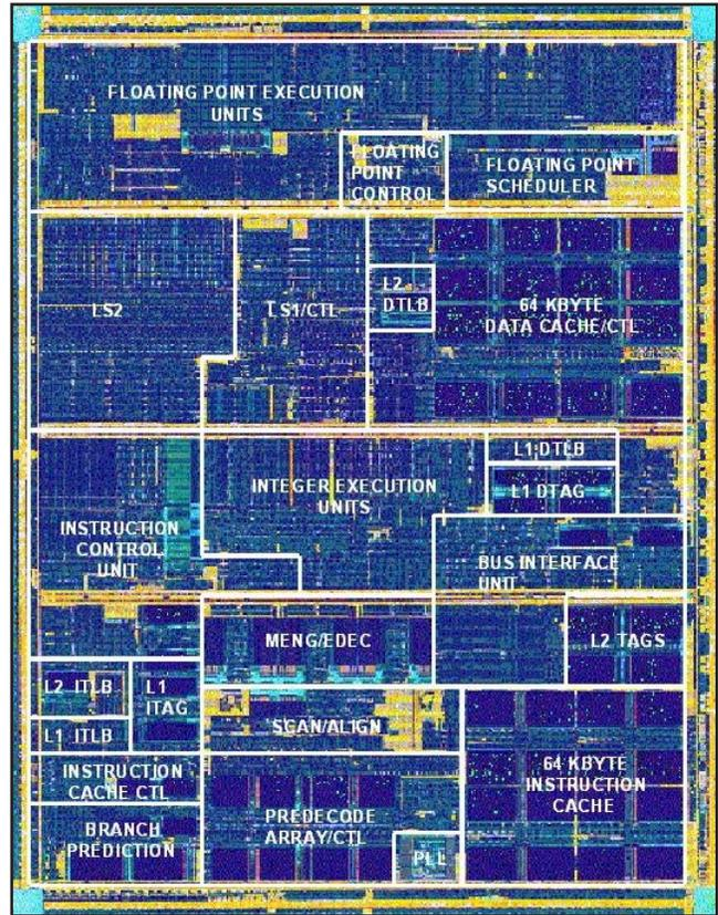
Figure 7. K7's 22 million transistors occupy 184 mm<sup>2</sup> in a slightly enhanced version of AMD's 0.25-micron 6-layer-metal CS44E process. (Source: AMD)
