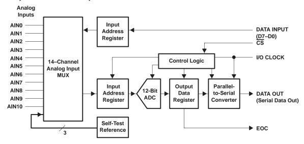
Figure 1. TLC2543 Block Diagram
