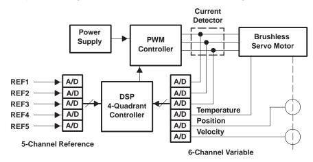
Figure 7. Brushless DC Servomotor Feedback System
