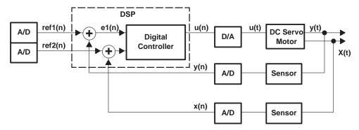
Figure 6. Compensator Block Diagram
