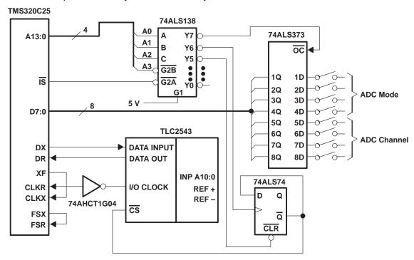
Figure 2. TLC2543/TMS320C25 Interface Circuit
