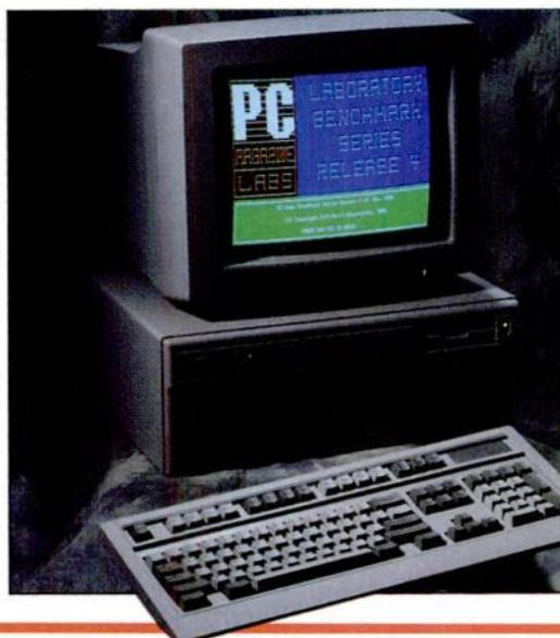
*The Tandy 5000 MC ships standard with a full assortment of I/O ports, including a connection for a VGA monitor. Tandy put the microprocessor and static-RAM controller on a proprietary 32-bit board.*
