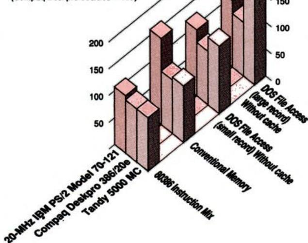
The DOS File Access benchmark test measures the throughput rate of the disk being tested. In this case, throughput times are measured in terms of how long the disk takes to perform common DOS file-management functions. Five tasks—file creation, sequential file write, sequential file read, random file write, and random file read—are timed and the results summed.
