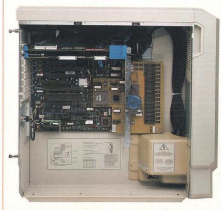
external cache is vital for multiuser performance; it unloads a good chunk of bus traffic and enables the 80486's burst mode. The BYTE benchmarks bear this out. IBM's 80486 Power Platform uses no external cache and suffers the consequences. For example, the VX FT Server was about 1.6 times faster than the IBM product on the string-move portion of the BYTE CPU tests. On the matrix, Sieve, and sort portions, there was virtually a tie. The string-move tests make extensive use of cache memory.
