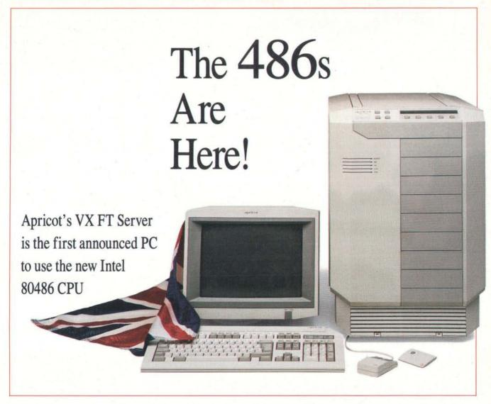
hile IBM and Compaq have been loudly engaged in a one-upmanship battle over who leads the market, Britain's Apricot has quietly introduced the first PC based on Intel's 80486 CPU. Unlike IBM's recently announced 80486 Power Platform upgrade for the PS/2 Model 70, the Apricot VX FT Server, based on the Micro Channel architecture (MCA), is an entirely new system with an external RAM cache. This cache memory provides a significant performance advantage over IBM's product.
