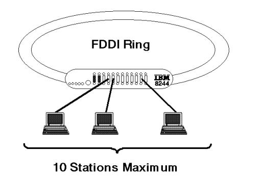
Figure 78. 8244 Standard Mode: Integrating Single Attachment Stations
