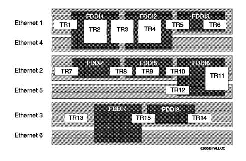
Figure 88. TriChannel Backplane Network Allocation
