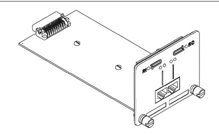
Figure 44. RJ-45 Ring In/Ring Out Module
