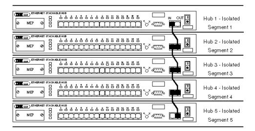
Figure 30. An IBM 8224 Stack - Fully Segmented. This example shows a stack of five hubs. Each hub has been segmented out of the network with an SNMP command to the IBM 8224 MIB. Thus, there are five segments and five collision domains now in the stack.
