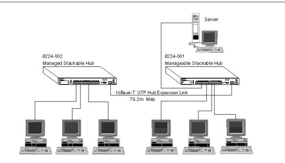
Figure 26. Interconnecting 8224 Hubs via the Hub Expansion Ports
