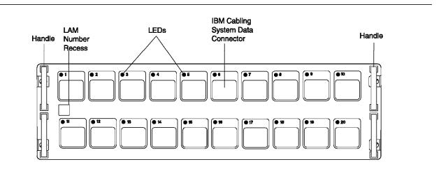
Figure 52. Front View, ICS Lobe Attachment Module (LAM)
