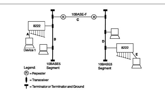
Figure 20. 8222 Hubs in a 10Base5 and Fiber Network
