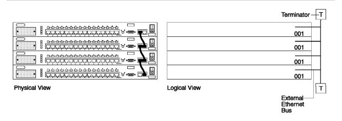
Figure 25. A Stack of Four 8224 Model 001s
