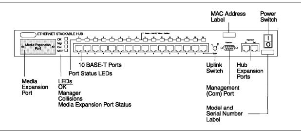
Figure 22. IBM 8224 Model 001 and 002 Front Panel
