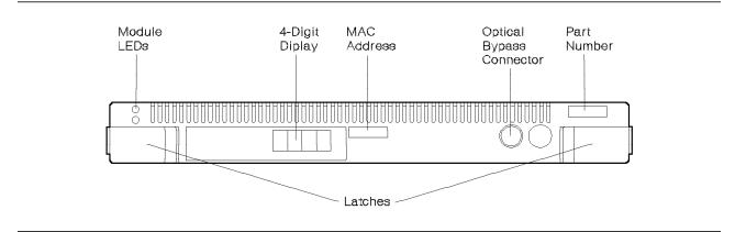
Figure 70. IBM 8240 Concentrator Control Module
