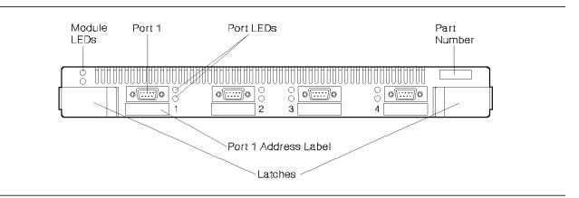
Figure 73. IBM 8240 Device Attachment Module for Copper
