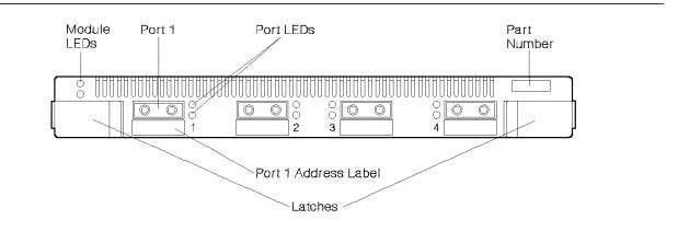
Figure 72. IBM 8240 Device Attachment Module for Optical Fiber
