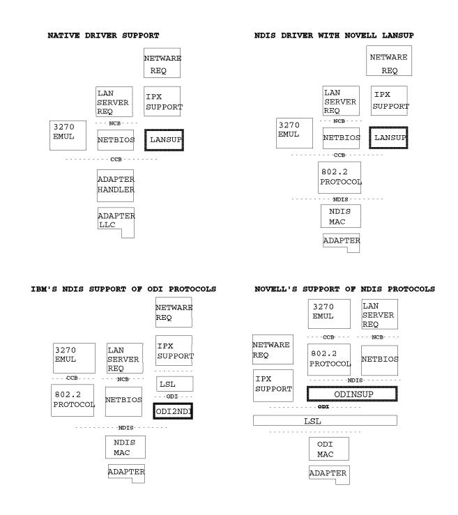
Figure 8. Mixed IBM and Novell Workstation Environments
