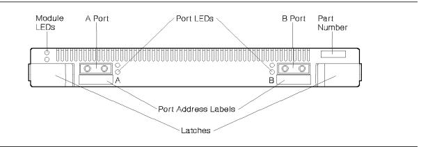
Figure 71. IBM 8240 Ring Attachment Module
