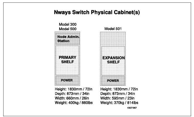
Figure 109. 2220 Nways Switch Rack Configuration
