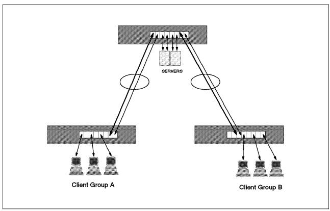
In Figure 99 you can see a connection between two switches using EtherPipe.
