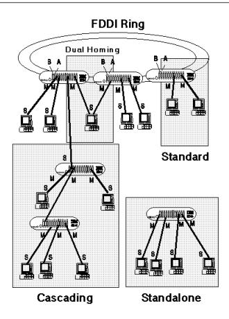
Figure 83. Keying 8244 Cable Plugs in Different Operating Modes
