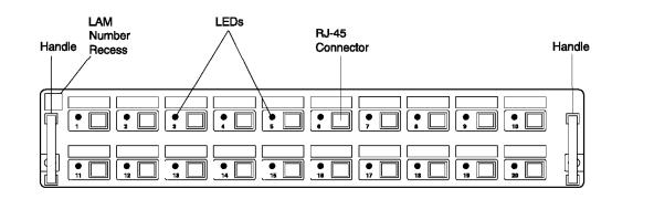
Figure 54. Front View, Shielded RJ-45 Lobe Attachment Module (LAM)
