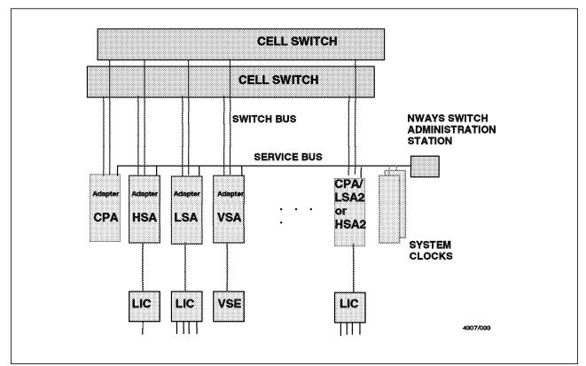
Figure 110. 2220 Nways Switch Hardware Components
