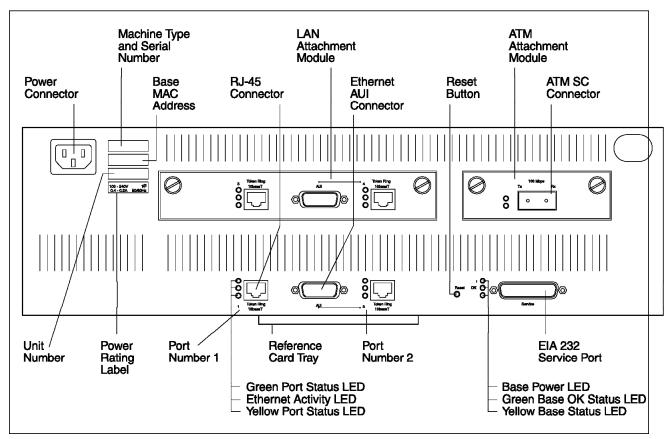
Figure 114. The 8281 Front Panel. The attachment modules are optional.
