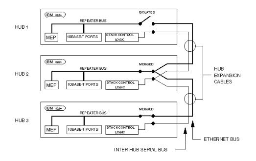
Figure 28. IBM 8224 Hub Expansion Port Interconnection. This example shows a stack of three hubs, one of which is segmented. Hub 1 is isolated (segmented) from the Ethernet bus in the hub expansion port cables via an SNMP command. Note that after segmentation the inter-hub serial control bus remains connected to the stack control logic in each of the hubs.
