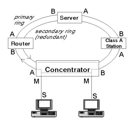
Figure 82. Optical Fiber Connections in 8244 Standard Mode
