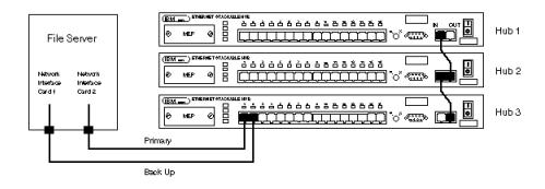
Figure 36. An IBM 8224 Stack - With Backup Port Enabled - Server Application. This example shows a hub stack connected to a server with 2 NICs. Port 1 is the primary connection. Port 2 is the secondary connection or backup port. The server must be rebooted after the transfer to the backup port to reset to the new node address in the backup server NIC.
