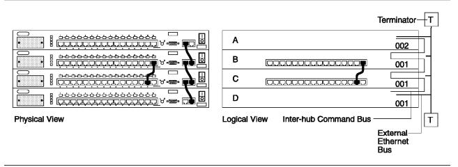
Figure 34. 8224 Hub C - Cascaded from Hub B
