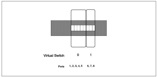
Figure 98. Example of Virtual Switch Configuration
