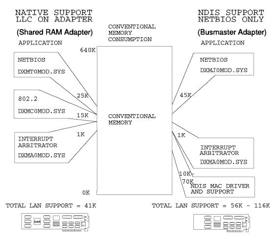
Figure 12. LSP DOS Memory Consumption with J0 Module
