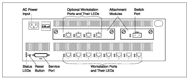
The following figure shows the front panel of the 8282 ATM Workgroup Concentrator:
