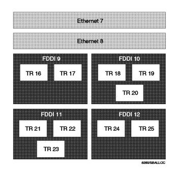
Figure 89. ShuntBus Backplane Network Allocation
