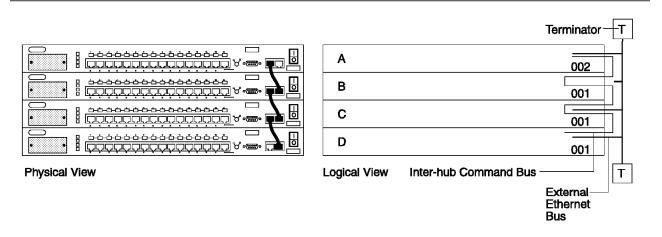
Figure 33. 8224 Hub B - Segmented from the External Ethernet Bus
