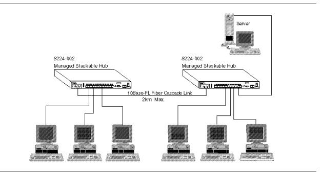
Figure 27. Cascading 8224 Hubs via Fiber Media Expansion Ports
