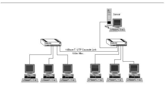
Figure 17. 8222 in a Typical IEEE 802.3 Network
