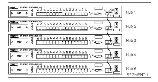
Figure 29. An IBM 8224 Stack - Unsegmented. This example shows a stack of five hubs, none of which are segmented. Thus, all are connected together in one segment or collision domain through the Ethernet bus in the hub expansion port cables.
