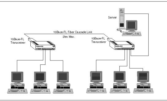
Figure 21. 8222 Hubs Connected with Fiber
