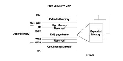
Figure 9. Memory MAP for DOS PS/2 Environments
