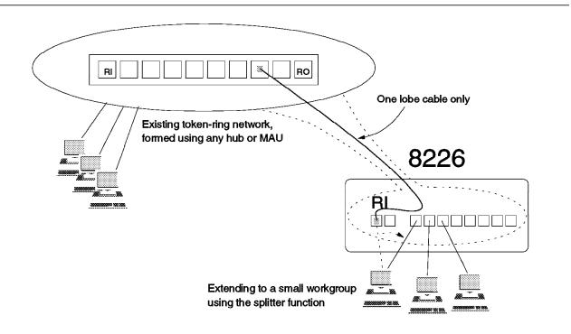
Figure 39. 8226 Splitter Mode. Instead of attaching to a workstation, the lobe cable can go into the RI port of an 8226 set in splitter mode. You then have eight ports to tie a small workgroup to the main ring.
