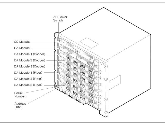
Figure 69. IBM 8240 FDDI Concentrator
