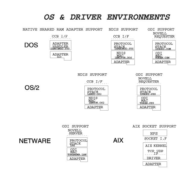
Figure 4. OS and Driver Environments with Module Name Examples
