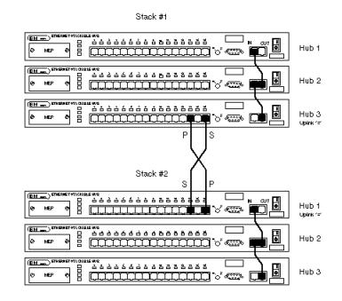
Figure 37. Two IBM 8224 Stacks - With Backup Ports Enabled - Cascading Application. This example shows multiple hub stacks connected via cascading over a backed-up 10Base-T link. The link between port 14 on hub 3 on stack 1 to port 16 on hub 1 of stack 2 is the primary (P) connection. The link between port 16 on hub 3 on stack 1 to port 14 on hub 1 of stack 2 is the secondary (S) or backup connection.
