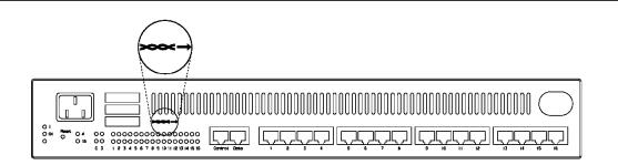
Figure 56. Front View, Remote LAM. Note that the magnified symbol in the diagram (of a piece twisted wire) appears only on the active RLAM.
