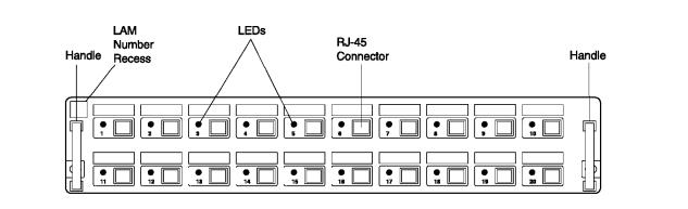
Figure 53. Front View, RJ-45 Lobe Attachment Module (LAM)
