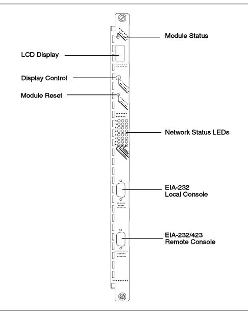
Figure 93. EC-DMM Front Panel
