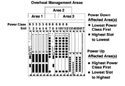
Figure 91. 8260 Cooling Zones and Power Classes
