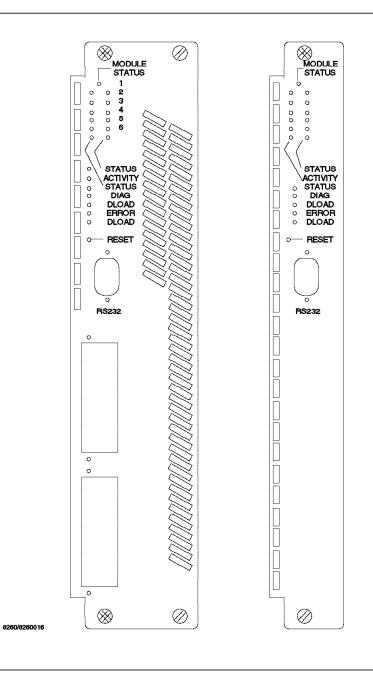
Figure 96. Front View of the Multiprotocol Interconnect Modules
