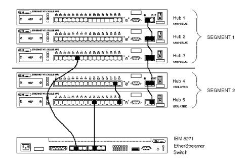
Figure 32. A Stack of IBM 8224 Hubs - Configured for Two Segments Joined with an IBM 8271 Switch. This example shows a segmented stack of 8224 hubs. Connectivity between the two collision domains is provided by an IBM 8271 EtherStreamer Switch.
