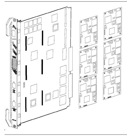
Figure 94. EC-DMM with Up to 6 E-MACs
