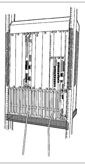
Figure 85. IBM 8260 Model 017. The 8260 has the 4-slot 8250 feature and a second power supply installed.
