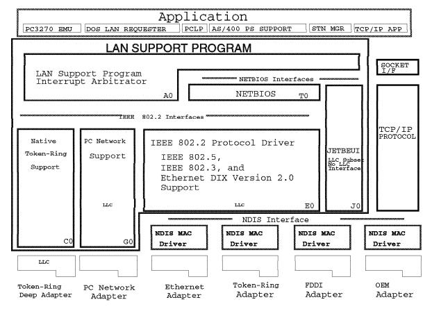
Figure 7. DOS Transport for IBM LAN Adapters
