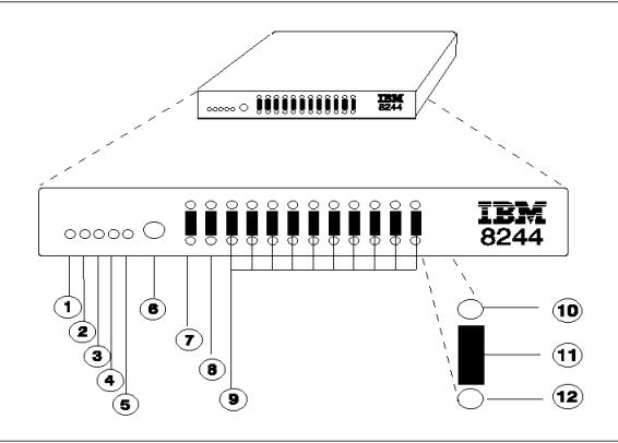
Figure 74. Front View of the 8244 Concentrator
