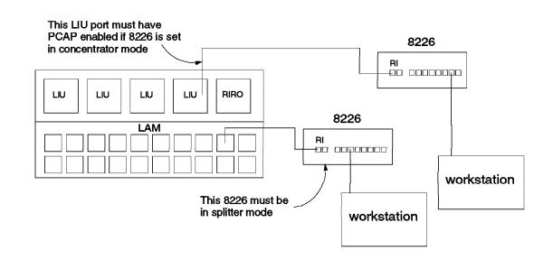
Figure 65. Fan-Out Using 8226s
