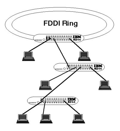
Figure 79. 8244 Cascading Mode: Using Cascaded Concentrators
