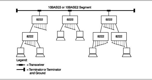
Figure 19. 8222 Hubs in a Network with Coaxial Segments
