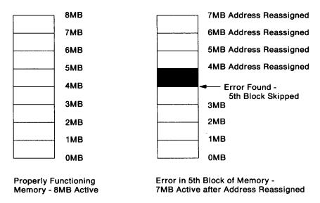
Figure 3-7. Memory Error Address Reassignment
