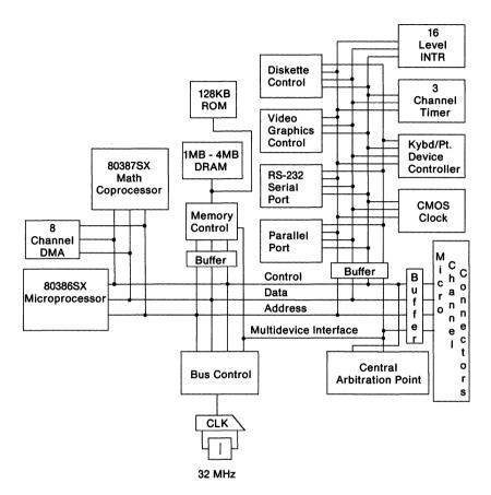
Figure 1-1. System Board Block Diagram
