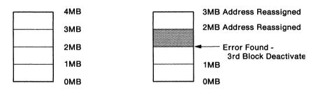
Properly Functioning Memory - 4MB Active Error in 3rd Block of Memory -3MB Active after Address Reassigned
