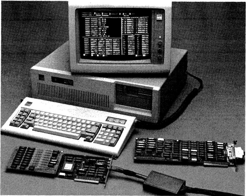
**Figure 5-16. TMS320C30 XDS1000 Algorithm Development Configuration**
