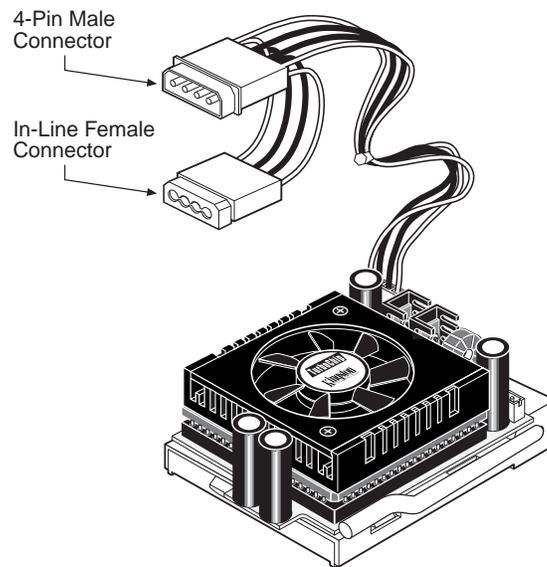
*Figure 7: Attaching the Power Cable*
