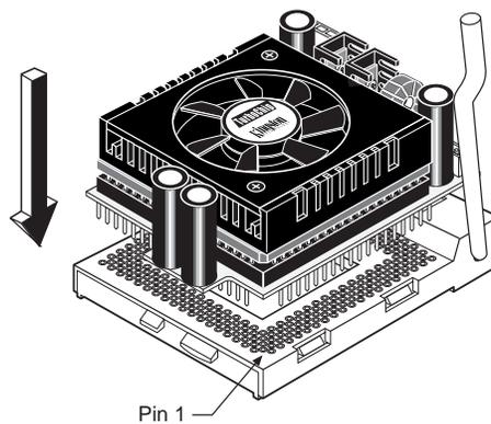
*Figure 5: Orienting the TurboChip*
