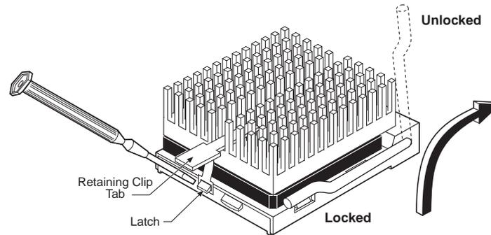
*Figure 4: Removing the CPU Chip*
