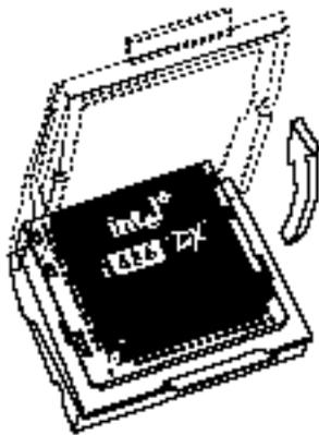
*Fig. 2-4 ZIF socket with Overhead Bar*
