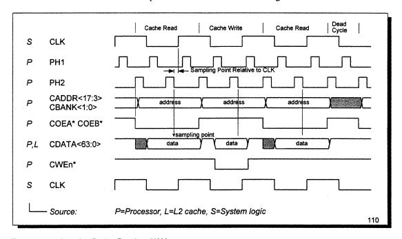
Figure 28 Level-2 Cache Read and Write
