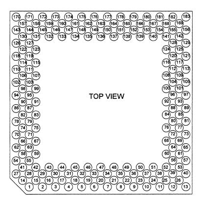
Figure 15 Nx587 Pinout Diagram (Top View)
