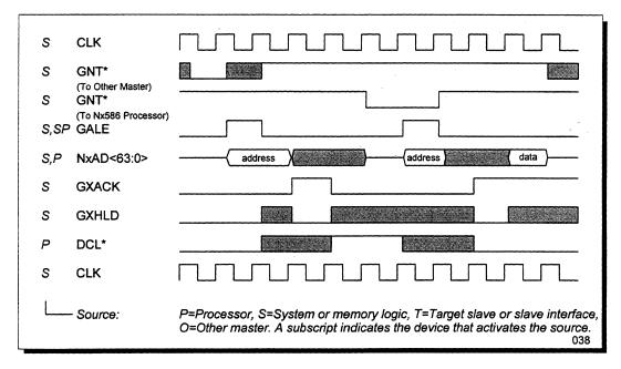
Figure 37 Single-Qword Read Hits Modified Cache Block
