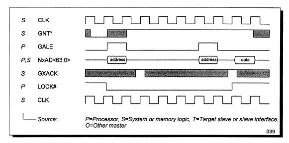
Figure 35 Interrupt-Acknowledge Cycle
