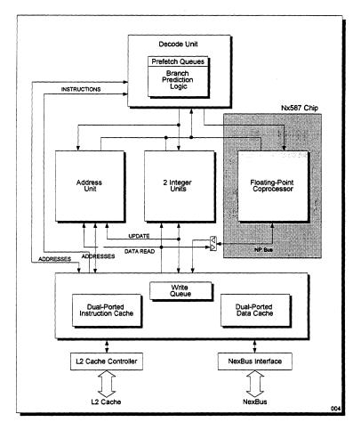
Figure 20 Nx586 Internal Architecture
