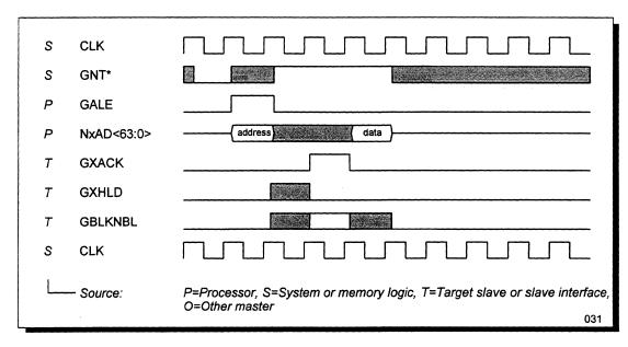
Figure 33 Fastest Single-Qword Write
