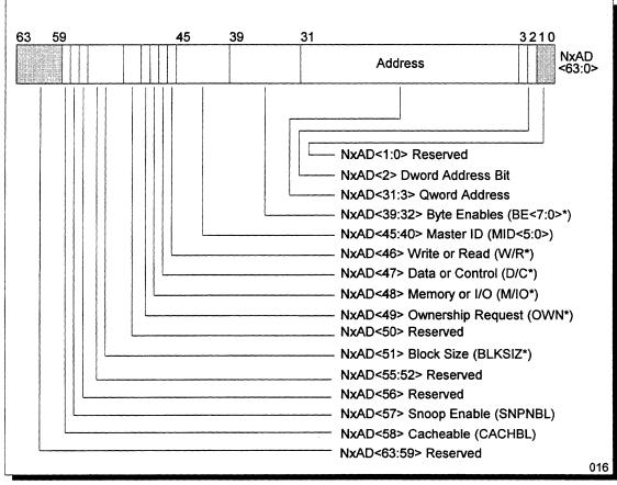
Figure 8 NexBus Address and Status Phase
