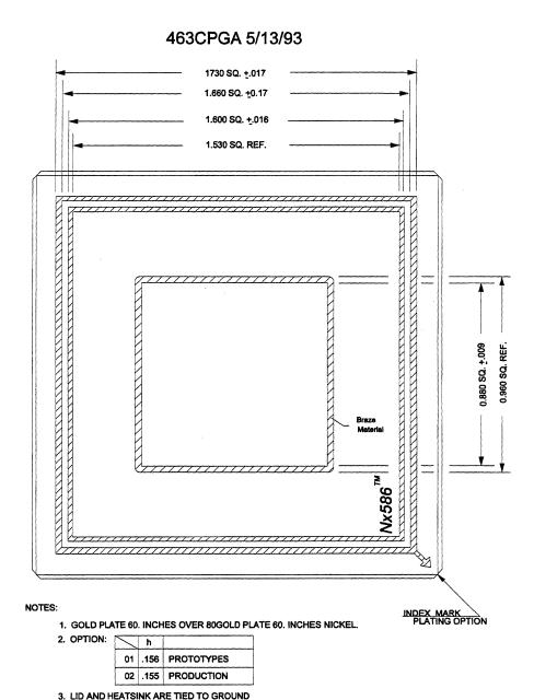
Figure 38 Nx586 Package Diagram (top)
