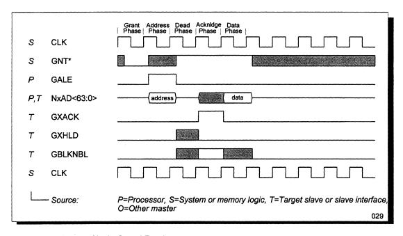
Figure 29 Fastest Single-Qword Read
