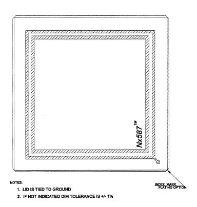
Figure 40 Nx587 Package Diagram (top)
