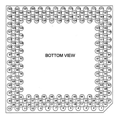
Figure 16 Nx587 Pinout Diagram (Bottom View)
