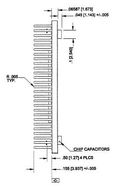
Figure 41 Nx587 Package Diagram (side)
