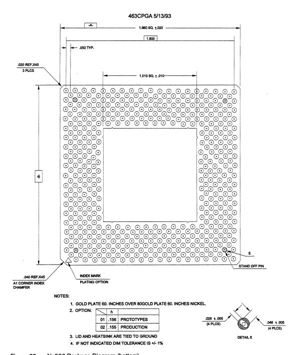
Figure 39 Nx586 Package Diagram (bottom)
