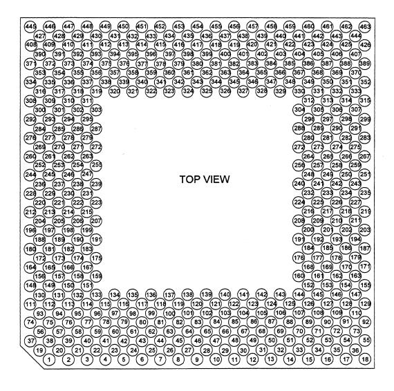
Figure 6 Nx586 Pinout Diagram (Top View)
