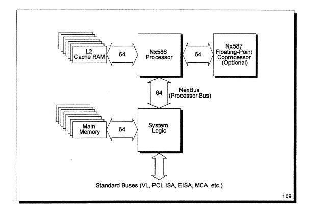
Figure 17 Nx586 based System Diagram
