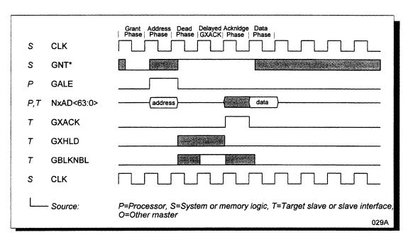
Figure 30 Fast Single-Qword Read with a delayed GXACK
