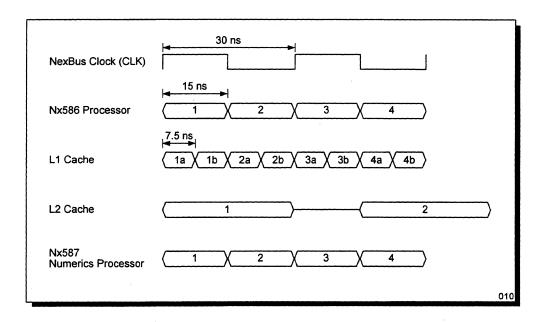
Figure 19 Operating Frequencies (66MHz Processor)
