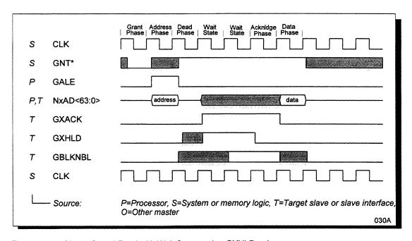
Figure 32 Single-Qword Read with Wait States using GXHLD only
