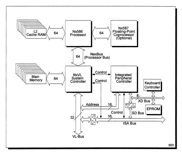
Figure 18 Nx586 based System using the NxVL Diagram
