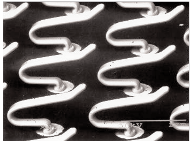
Figure 1. MicroSpring contacts are small and strong. The shape and size of the spring and the contact at the spring's tip vary according to the intended application. These springs are used in an LGA socket.
