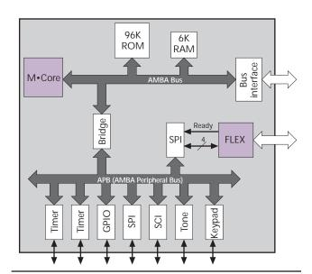
Figure 1. The MMC2080 combines a 10-MHz M•Core processor with assorted peripherals and a complete Flex paging-protocol decoder, for a self-contained 32-bit paging controller.
