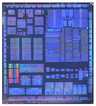
Figure 1. Motorola's MPC8260 PowerQUICC II processor measures  $11 \times 12$  mm in the company's 0.29-micron HIP 3 process and contains approximately five million transistors.
