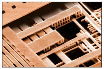
Figure 1. This photomicrograph shows all six copper interconnect layers from Motorola's upcoming 0.18-micron HiPerMOS 6 process. (Source: Motorola)
