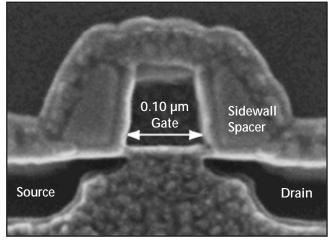
Figure 3. Transistor gate length is often pushed well below a process's typical minimum feature size, as shown in this photomicrograph of a transistor from Motorola's 0.18-micron HiPer-MOS 6 process. (Source: Motorola)
