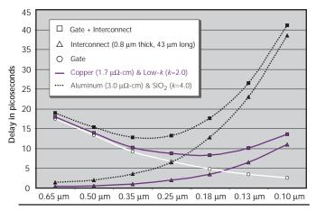
Figure 2. Gate speed continues to improve as geometries shrink, but interconnects slow down. As this example shows, copper and low-k dielectrics will become mandatory in future generations. (Source: Mark Bohr, Intel, IEDM 95)
