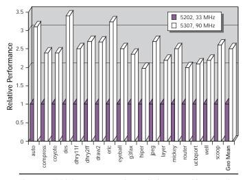
**Figure 1.** With its newer core, faster clock rate, and larger cache, the 90-MHz 5307 runs 2–3 times faster than a 33-MHz 5202 ColdFire part. (Source: Motorola)
