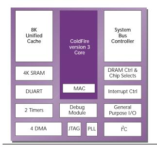
Figure 2: The 5307 has a large, unified 8K cache, 2K of SRAM, and a built-in DRAM controller, making it a single-chip controller.
