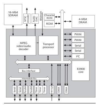
**Figure 1.** Toshiba's TC81220F satellite television decoder includes several autonomous units, including an R3900 MIPS core and a programmable transport processor. With 512K of DRAM, 2M of synchronous DRAM, and some analog components, the chip can implement a complete DSS system.
