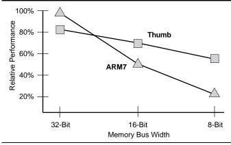
Figure 2. Comparing ARM7 cores with and without Thumb shows the effects of memory bus width on performance. The 16-bit Thumb instruction set surpasses ARM in low-cost systems. (Source: ARM).
