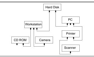
Figure 1. FireWire's point-to-point connections allow combined daisy-chain and tree topologies with a maximum of 16 hops. Current performance levels limit node-to-node distance to 4.5 meters.
