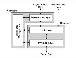
Figure 3. The TI chip set implements layers of the protocol stack partially in hardware, partially in firmware.
