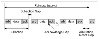
Figure 4. Nodes acknowledging transactions receive higher priority and are allowed to transmit immediately after any data packet. Other nodes must wait longer to arbitrate for bus ownership, creating the subaction gap.
