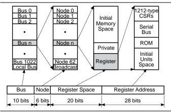
Figure 2. P1394 draws upon the IEEE 1212 standard for its definition of 64-bit fixed addressing. Sixty-three nodes on 1024 buses are each assigned 256 terabytes of address space.
