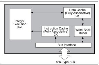
Figure 1. The W89K's fully associative caches deliver hit rates similar to larger direct-mapped caches but use less space.
