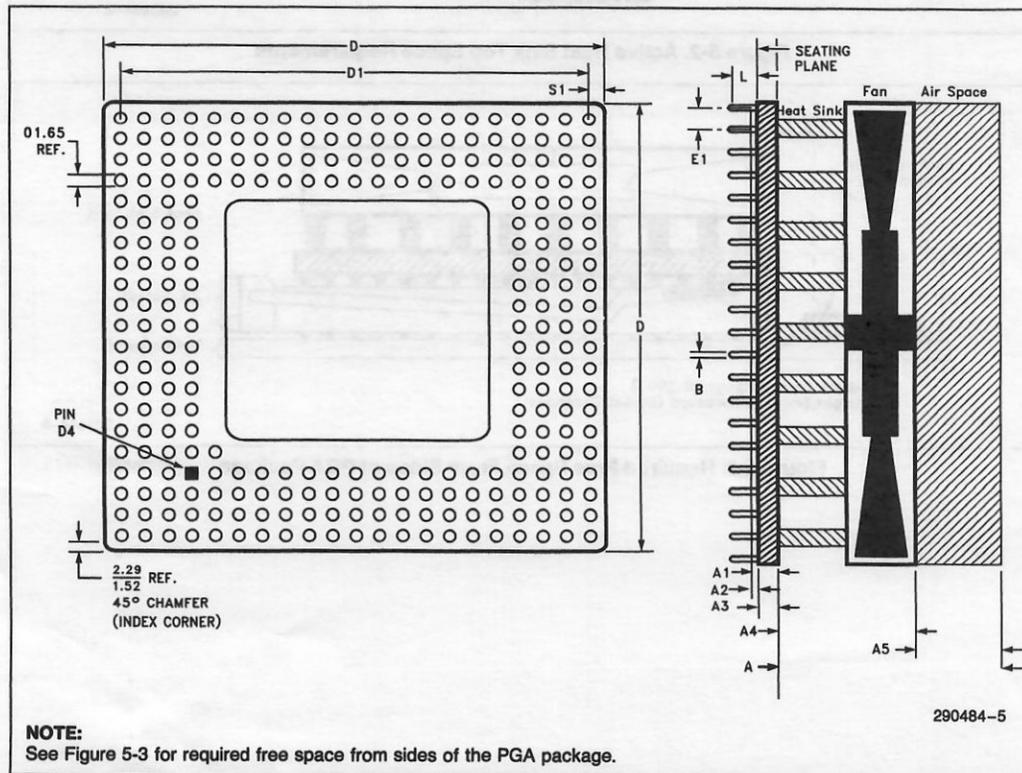
Figure 5-1. OverDrive™ Processor Package Dimensions
