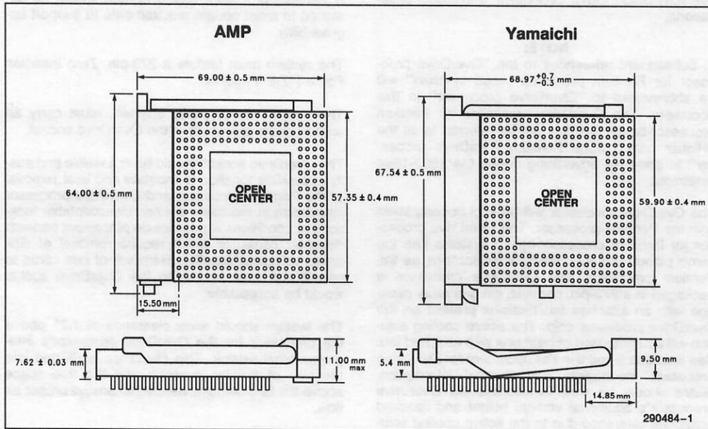
Figure 2-1. OverDrive™ Socket Footprint Dimensions
