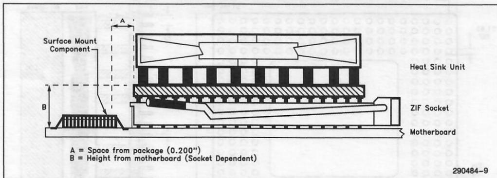
Figure 5-3. Required Free Space From Sides of PGA Package
