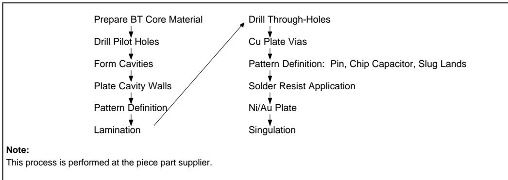
Figure 4. Piece Part Substrate Manufacturing and Lamination Process
