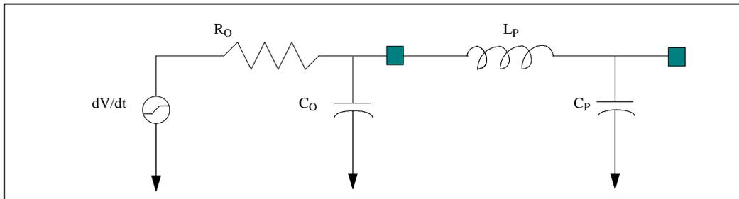
Figure 8. First Order I/O Buffer Model for PPGA
