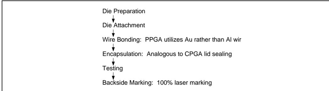
Figure 5. Intel PPGA Assembly Process
