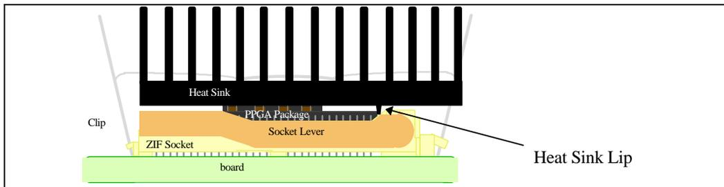
Figure 10. A Heat Sink Design With a Lip
