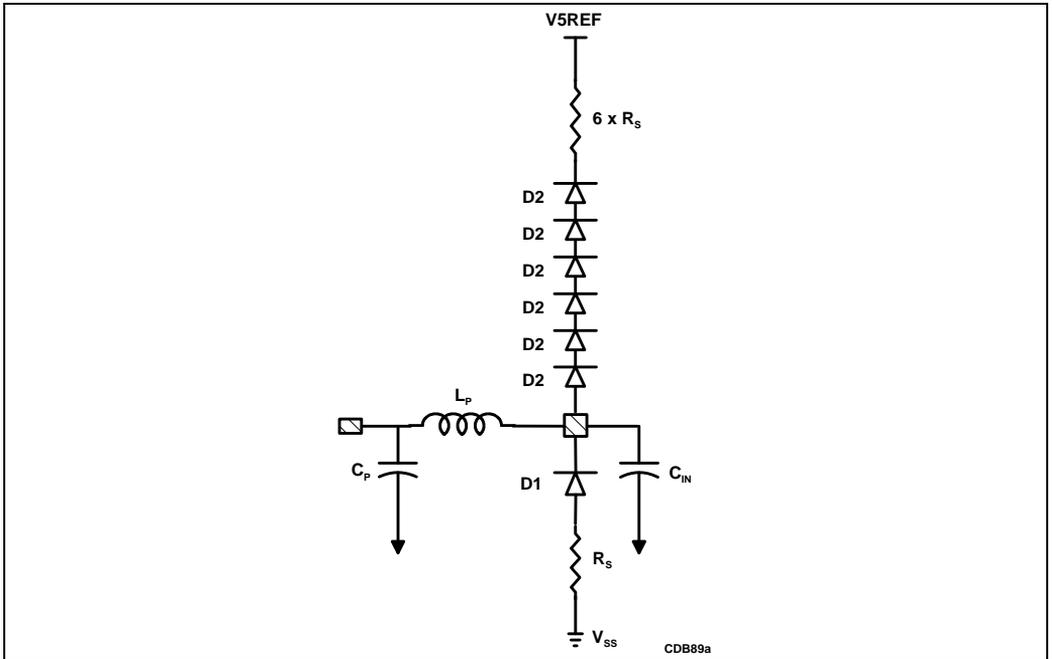
**Figure 24-6. Complete 5V Tolerant Input Model Including 6 Diodes**
