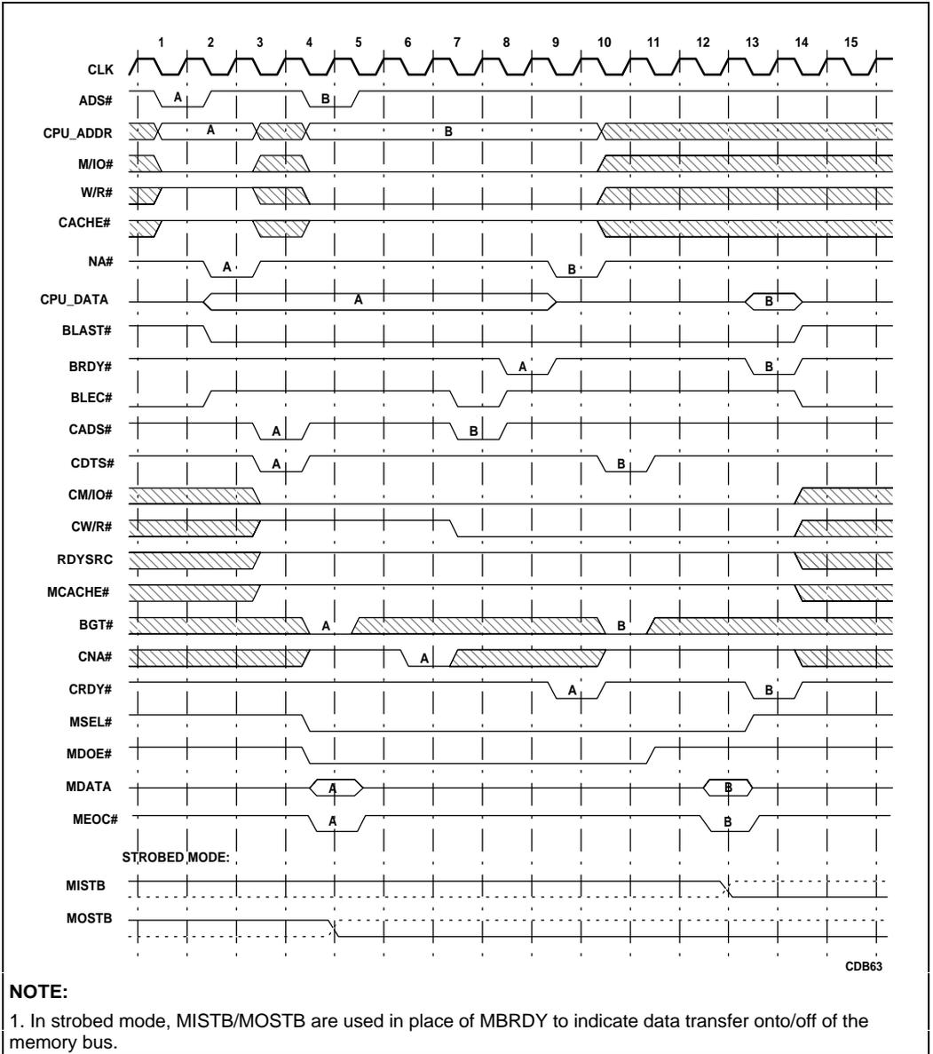
Figure 6-10. I/O Cycles
