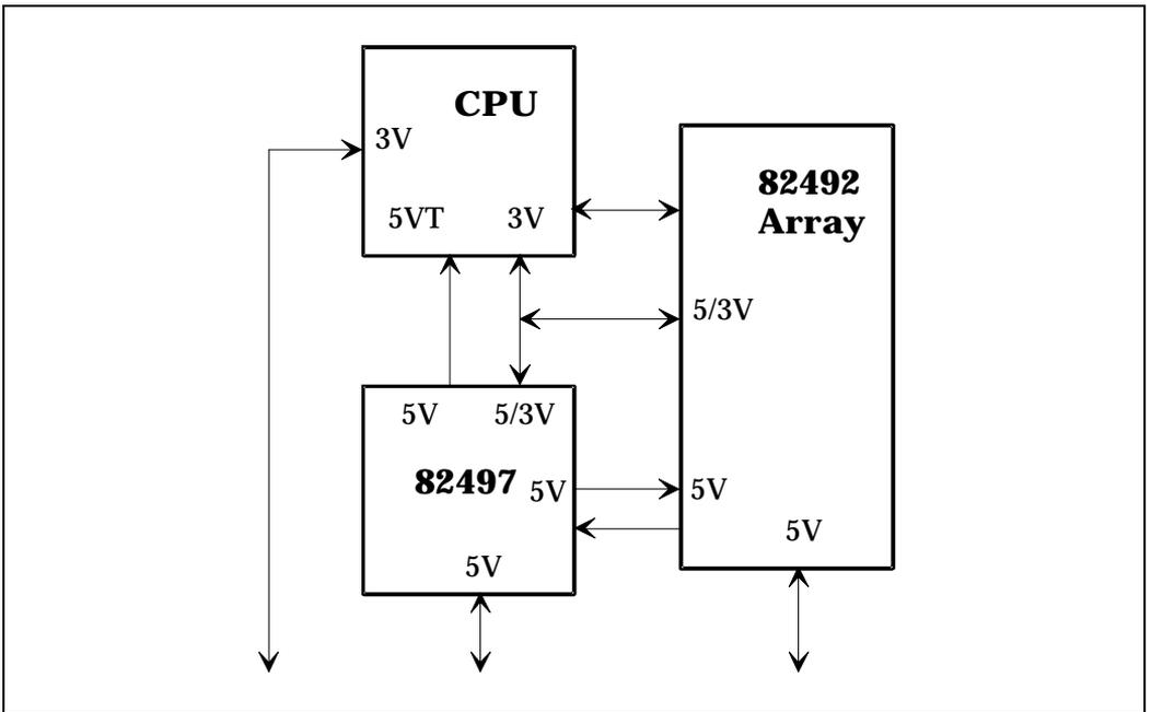
**Figure 13-2. Interface Buffer Types**
