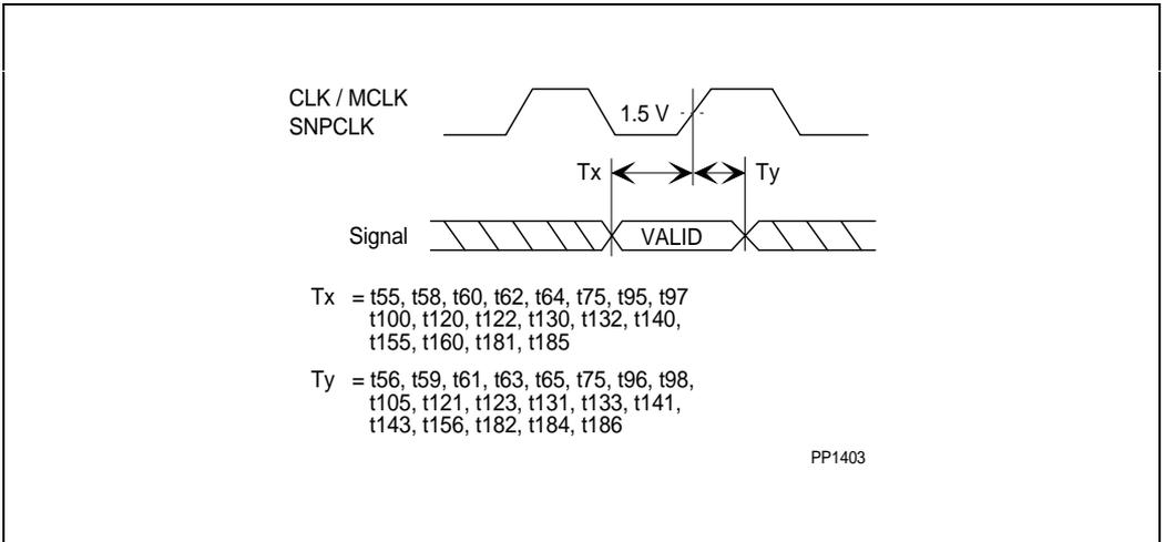
Figure 14-5. Setup and Hold Timings
