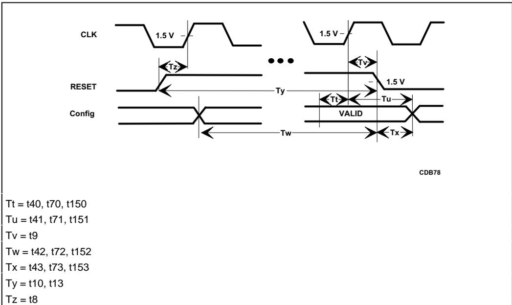
Figure 23-9. Reset and Configuration Timings
