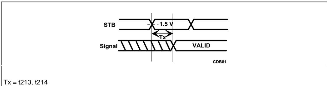
Figure 23-13. Valid Delay Timings from Strobes
