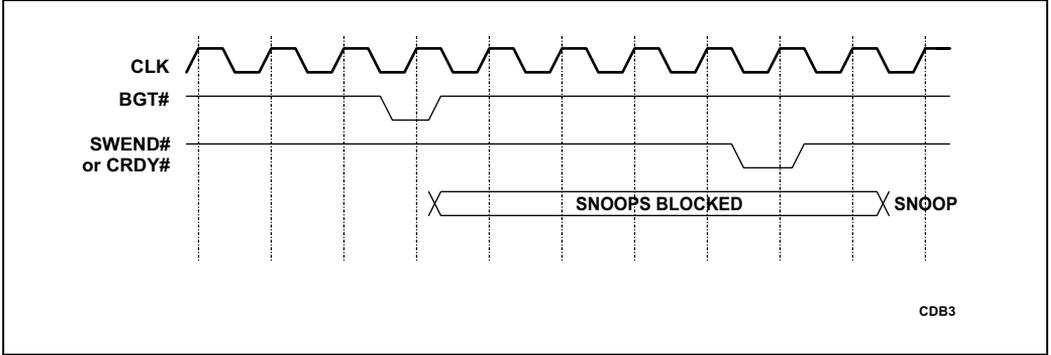
**Figure 22-12. Snoop Response Blocking Using BGT#**
