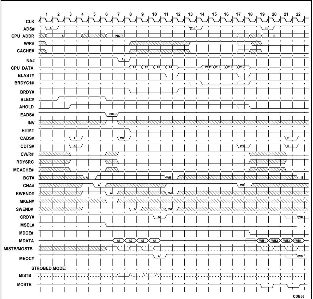
Figure 6-3. Read Miss with Replacement of Modified Line
