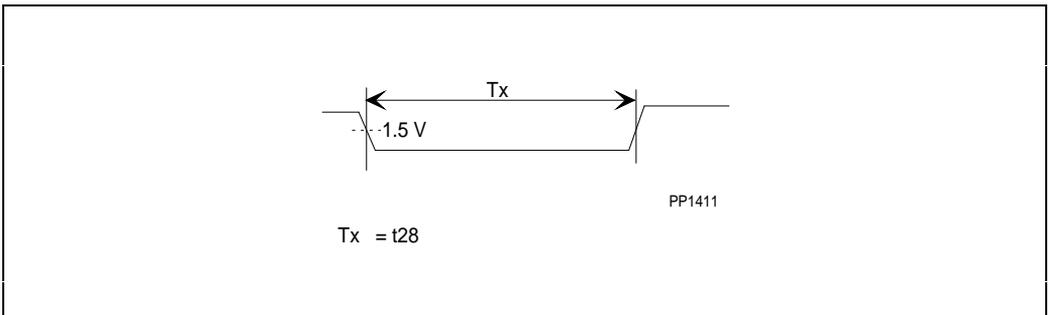
Figure 14-13. Test Reset Timings
