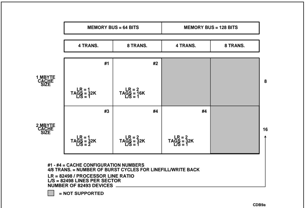
Figure 21-1. 82498 Cache Controller/82493 Cache SRAM Configurations with the Pentium® Processor (735\90, 815\100, 1000\120, 1110\133)
