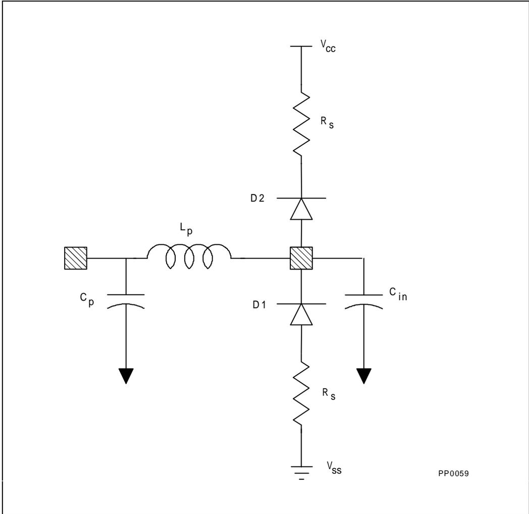
Figure 15-1. Input Buffer Model, Except for Group CPU-CCTL5T
