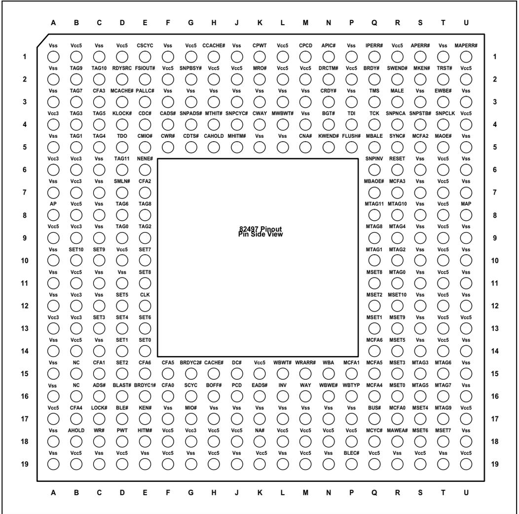
Figure 12-2. 82497 Cache Controller Pinout Pin Side View
