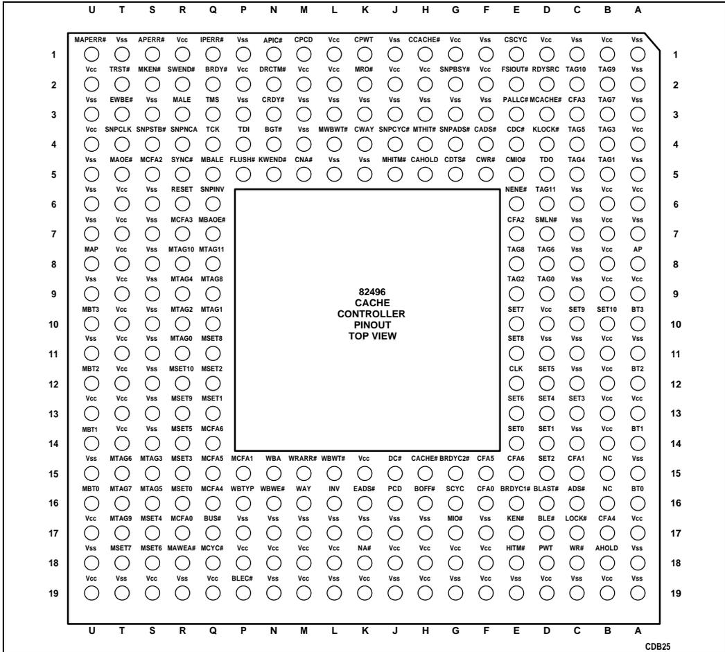
Figure 1-3. 82496 Cache Controller Pinout (Top View)
