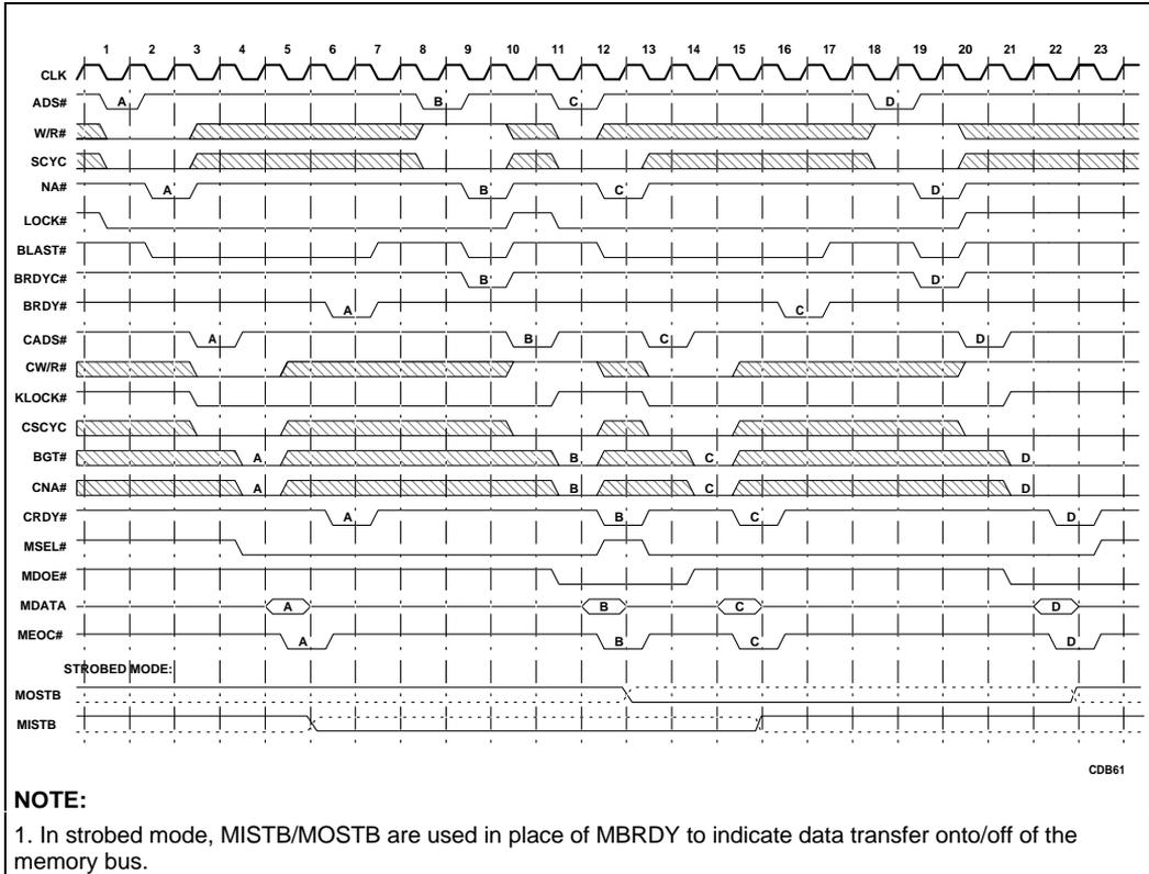
Figure 6-8. Locked Read Modify Write Cycles
