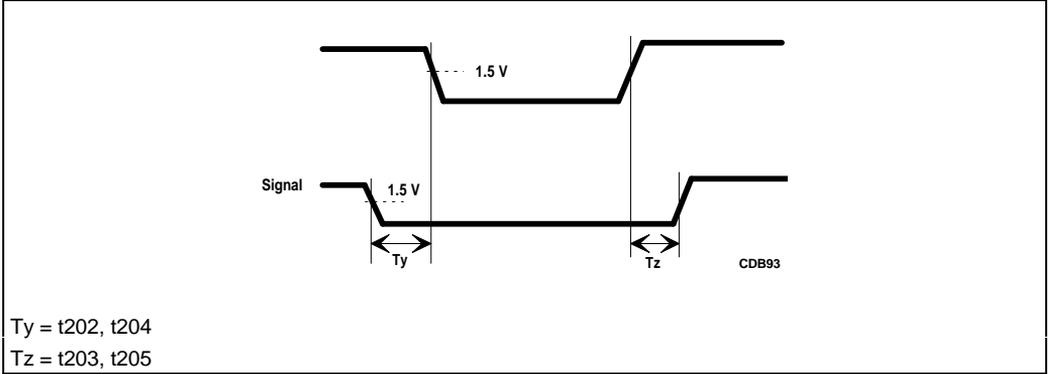
Figure 7-12. Setup and Hold Timings  $M_xST$
