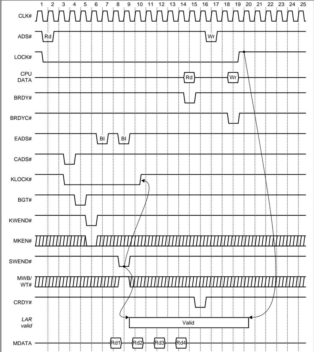
Figure 22-4. Non-Split LOCKed Read Miss - Line Fill to E/M
