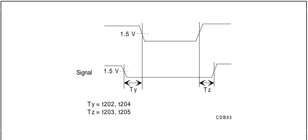
Figure 14-9. Setup and Hold Timings to Strobes
