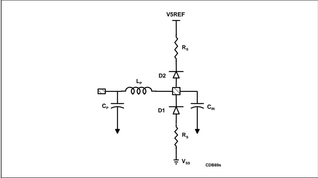
Figure 24-5. Complete 5V Tolerant Input Model Including Diode
