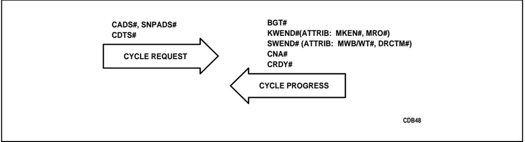
Figure 5-2. Memory Bus Cycle Progress and Attribute Signals
