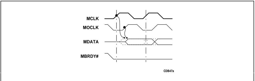
**Figure 5-29. Increasing Hold Time of Output Burst Data**
