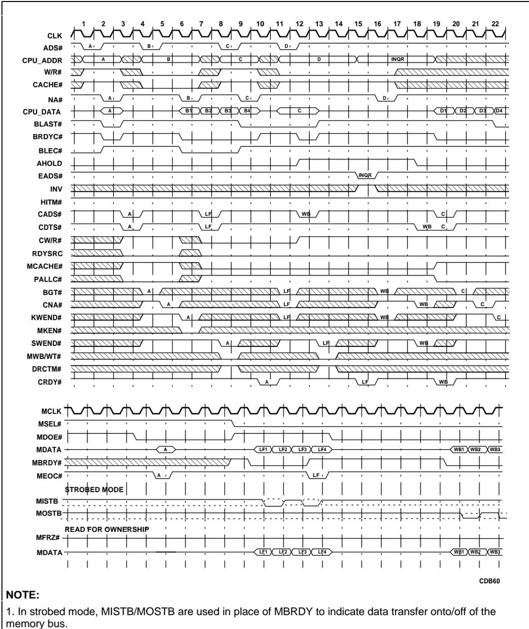
Figure 6-7. Write Miss with Allocation to Modified Line
