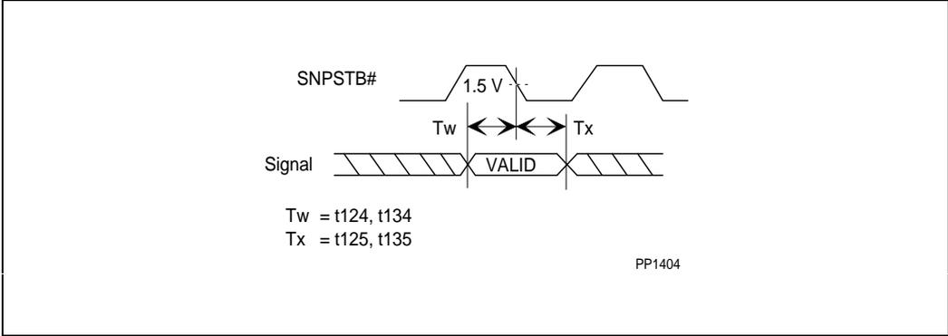
Figure 14-6. Setup and Hold Timings in Strobed Snooping Mode
