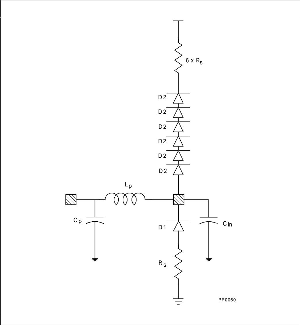
Figure 15-2. Input Buffer Model for Group CPU-CCTL5T
