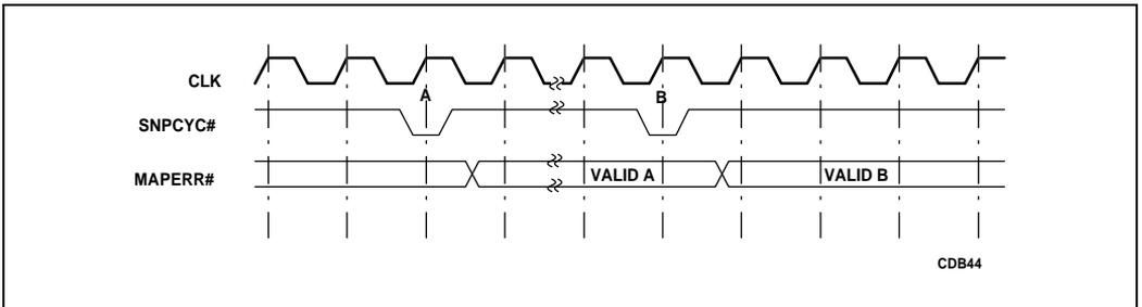
Figure 5-18. MAPERR# Timing for Asynchronous Snoop Modes
