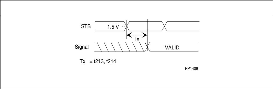
Figure 14-11. Valid Delay Timings From Strobes
