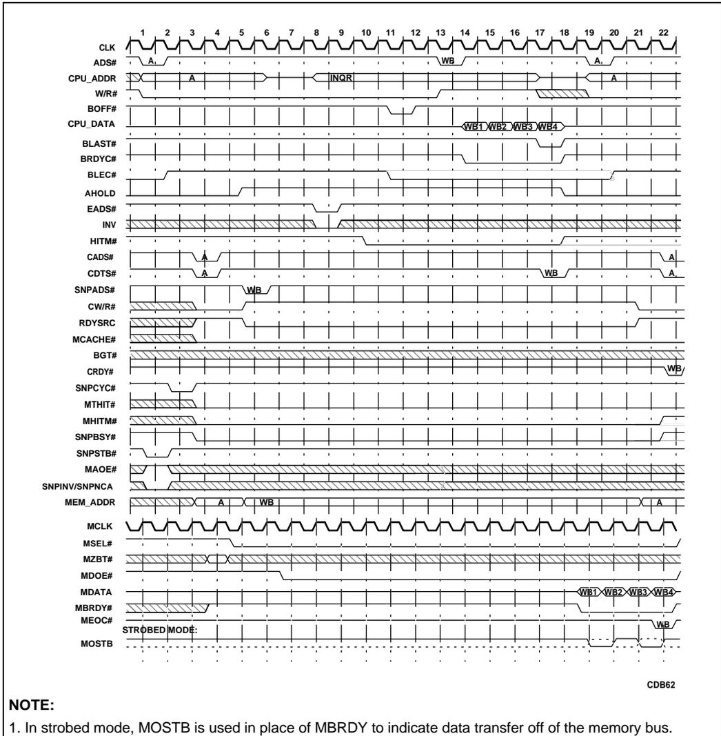
**Figure 6-9. Snoop Hit to [M] State — Synchronous Snoop Mode**
