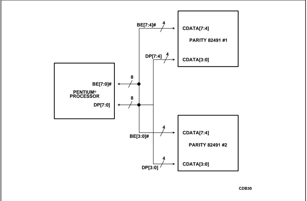
Figure 5-21. Pentium® Processor/82491 Cache SRAM Data Parity Connections
