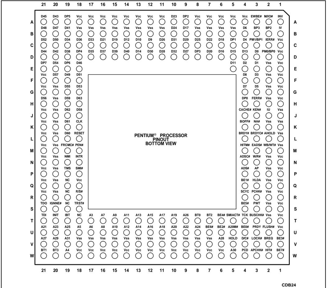
Figure 1-2. Pentium® Processor Pinout (Bottom View)
