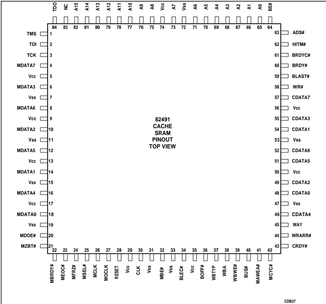
Figure 1-5. 82491 Cache SRAM Memory Pinout (Top View)
