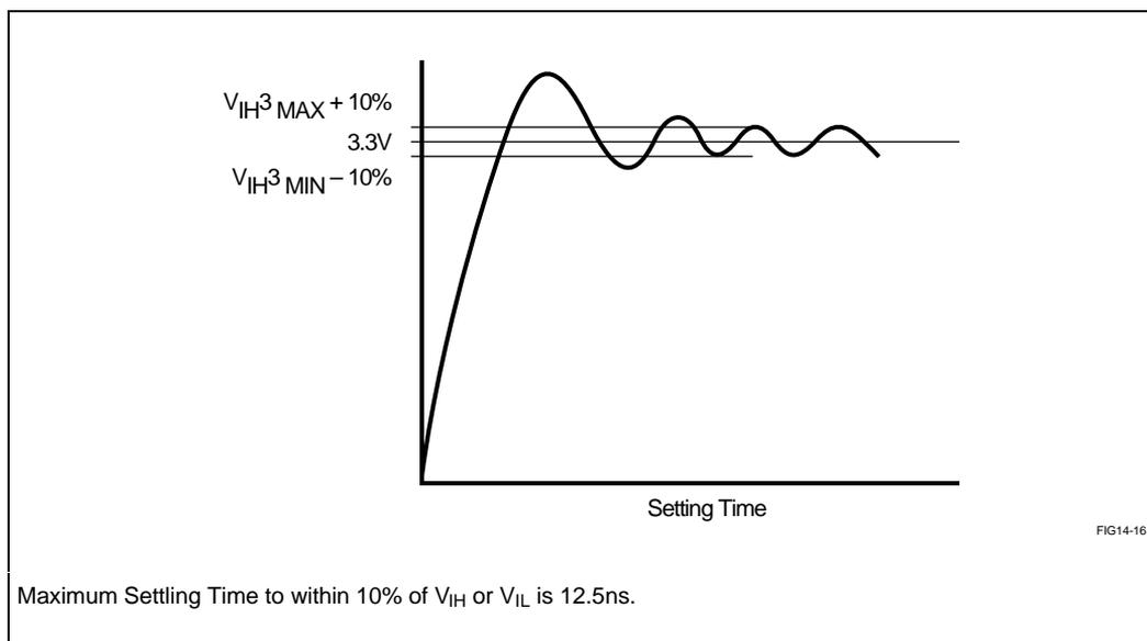
Figure 14-16. Settling Time
