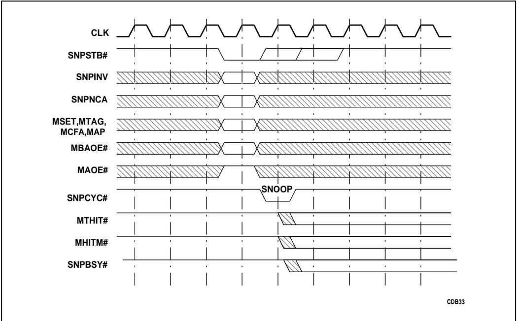
Figure 5-4. Synchronous Snoop Mode
