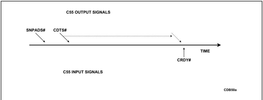
**Figure 22-15. Cycle Progress for Snoop Write Back Cycles**
