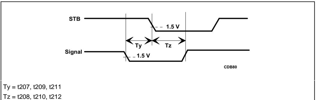
Figure 23-11. Setup and Hold Timings to Strobes
