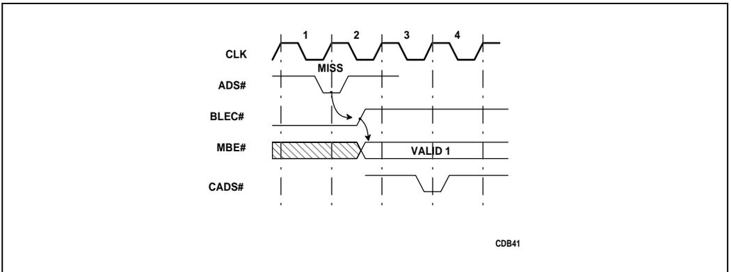
Figure 5-23. BLEC# Deassertion Due to ADS# Assertion
