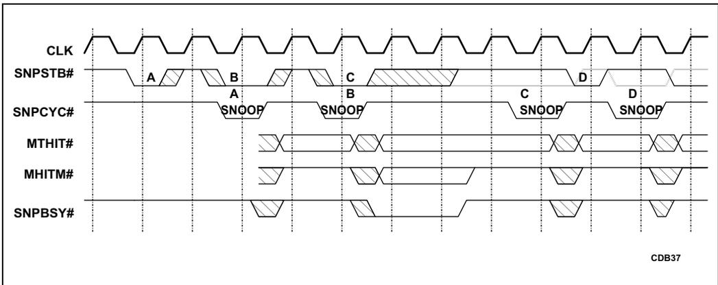
Figure 22-8. Fastest Asynchronous Snooping
