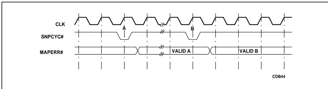
**Figure 5-27. MAPERR# Timing**
