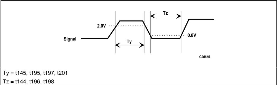
**Figure 7-16. Active/Inactive Timings**
