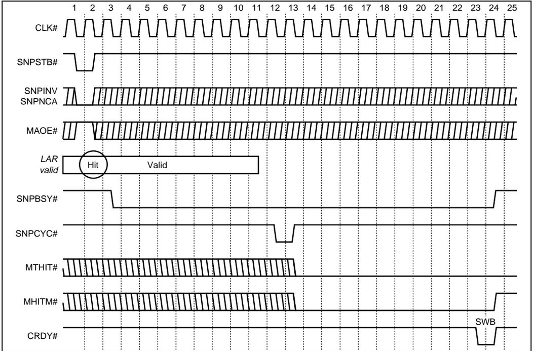
Figure 22-17. Snoop Hit to LOCKed Address Register
