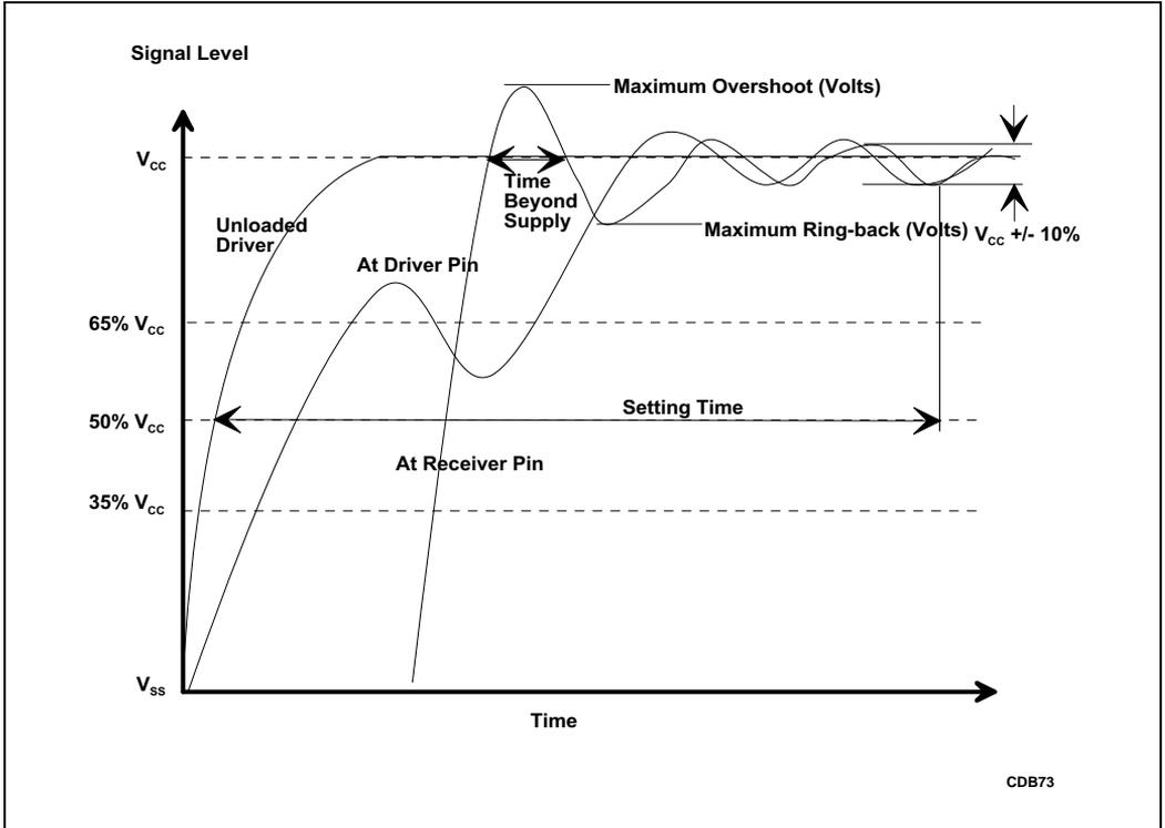
Figure 23-4. Driver and Receiver Signal Waveforms Showing Signal Quality Parameters
