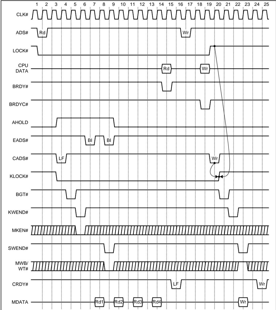
Figure 22-3. Non-Split LOCKed Read Miss with Clean Replacement
