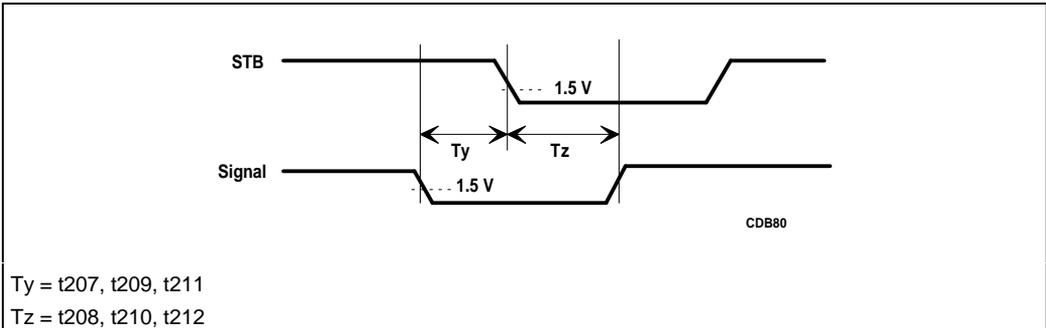
Figure 7-11. Setup and Hold Timings to Strobes
