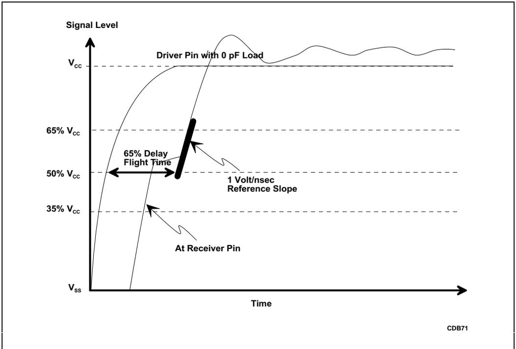
Figure 23-2. Derating the Flight Time
