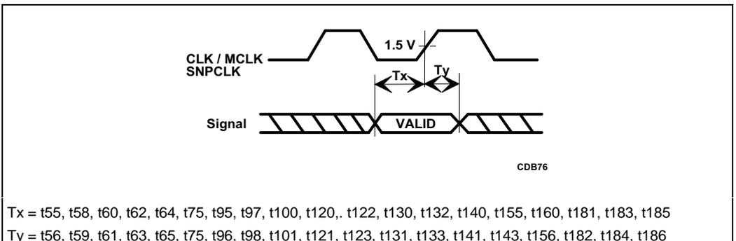
Figure 23-7. Setup and Hold Timings
