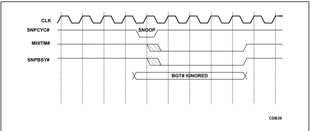
**Figure 22-13. Snoop Executing before BGT# Is Asserted**
