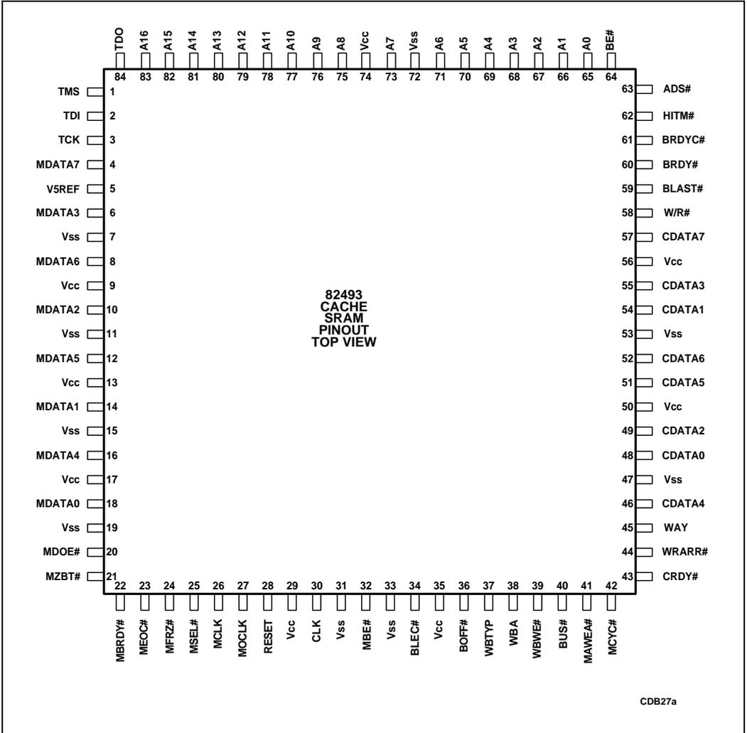
Figure 20-3. 82493 Cache SRAM Memory Pinout (Top View)
