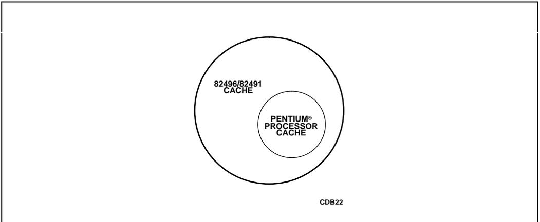
**Figure 3-2. Pentium® Processor Cache Chip Set Cache Inclusion**
