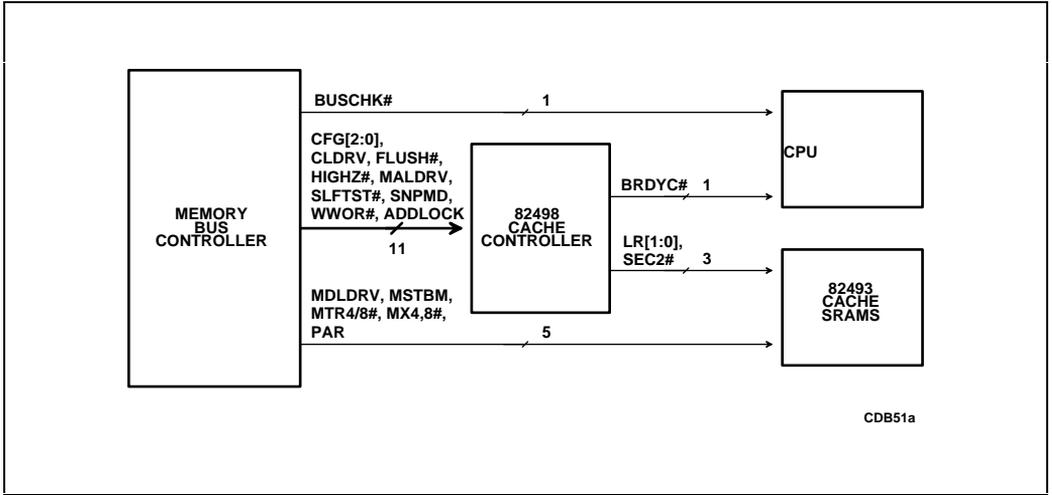
**Figure 21-3. CPU-Cache Chip Set Configuration Inputs**
