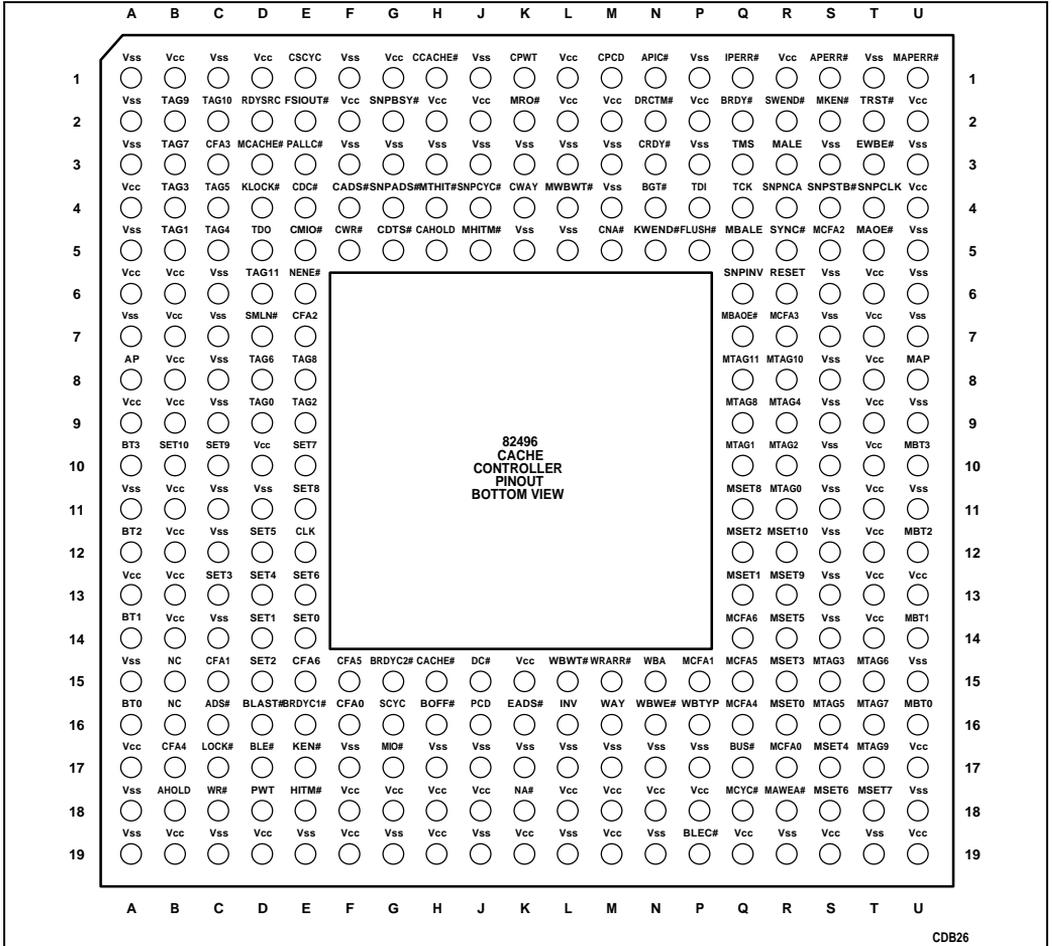
Figure 1-4. 82496 Cache Controller Pinout (Bottom View)
