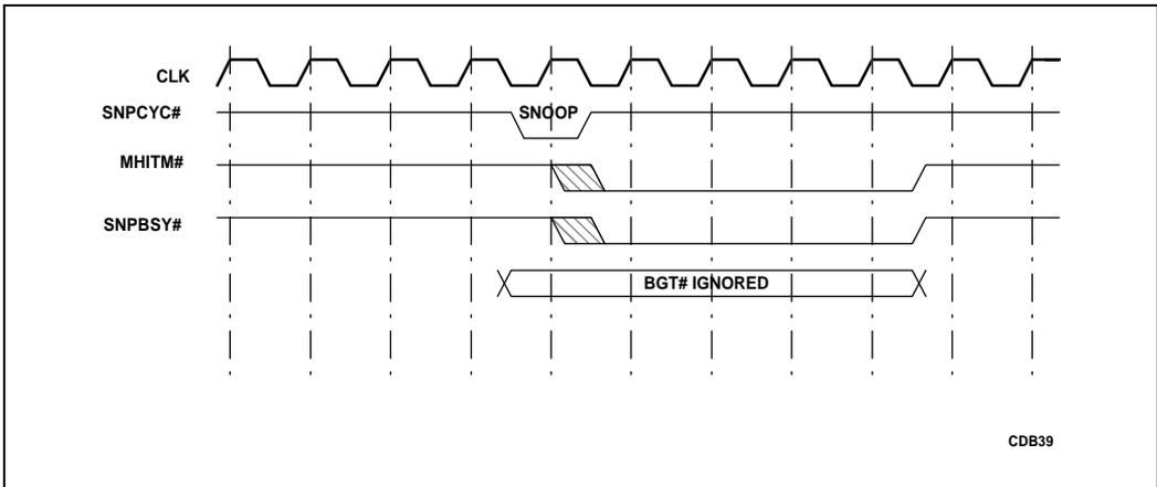
Figure 5-14. Snoop Executing before BGT# is Asserted
