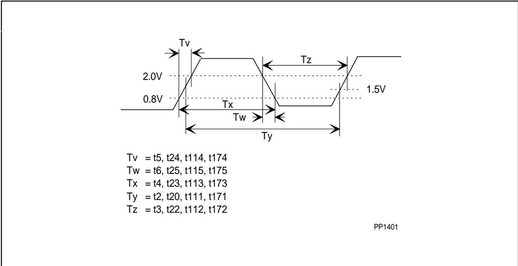
**Figure 14-3. Clock Waveform**
