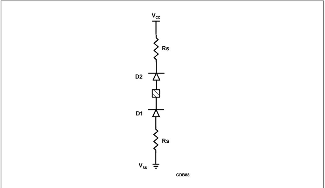
Figure 8-3. Input Diode Model
