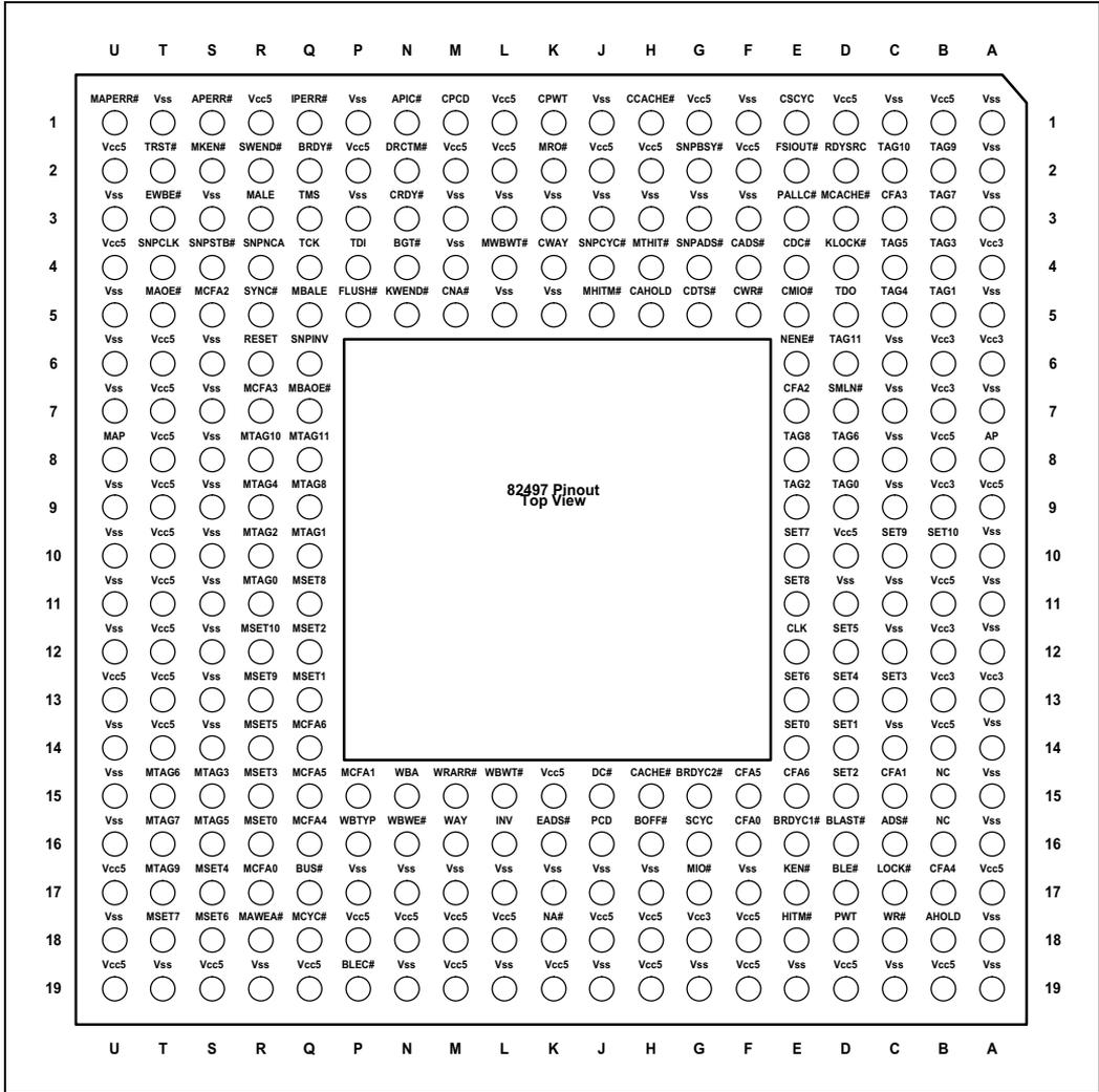
Figure 12-1. 82497 Cache Controller Pinout Top Side View
