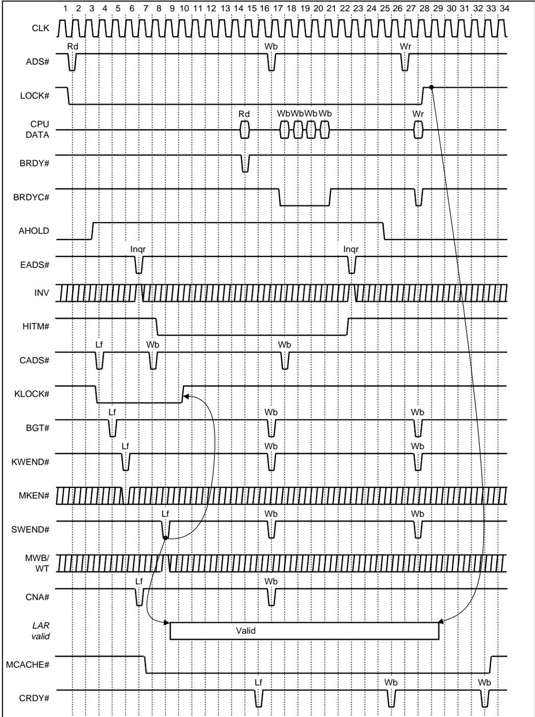
Figure 22-5. Non-Split LOCKed Read Miss - Replacement of Modified Line
