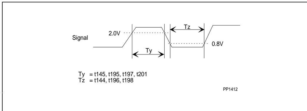
Figure 14-14. Active/Inactive Timings
