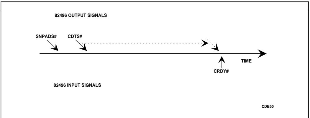
Figure 5-16. Cycle Progress for Snoop Writeback Cycles
