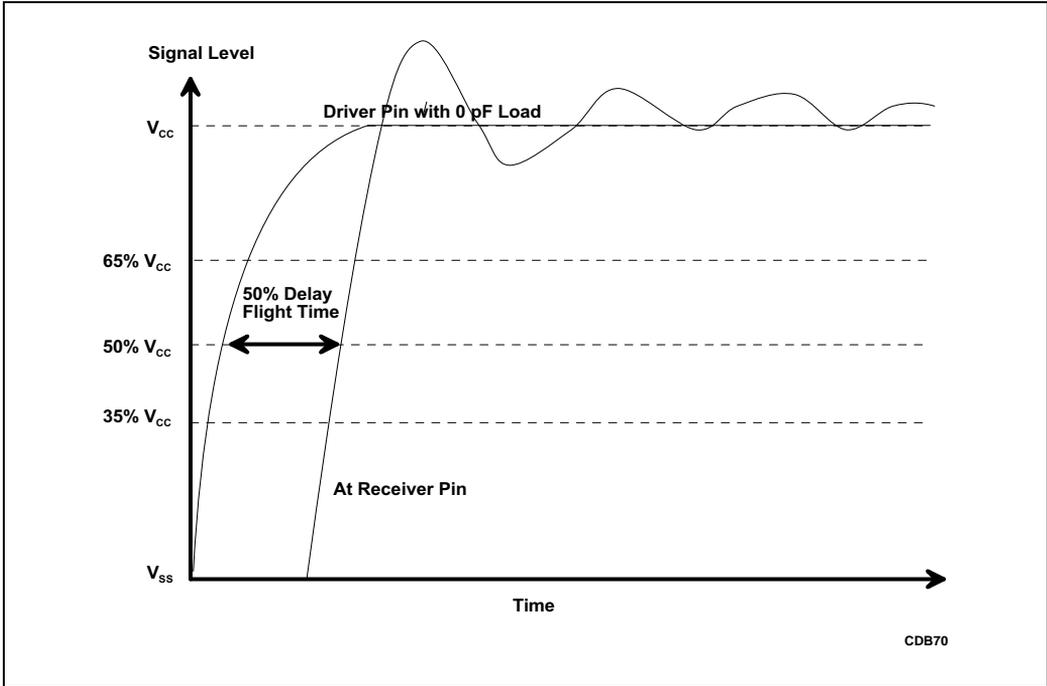
**Figure 7-1. Determination of Flight Time**
