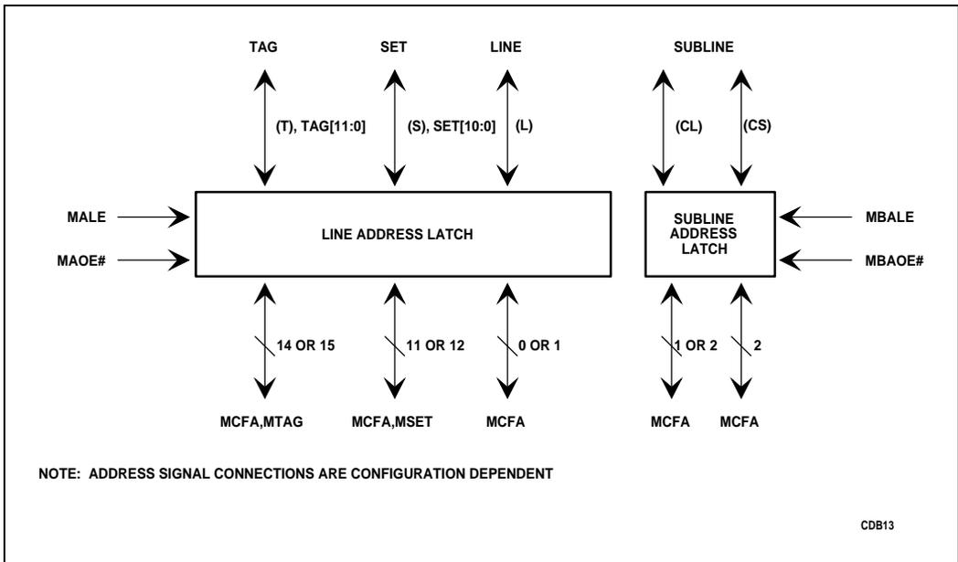
**Figure 4-5. Address Latching**
