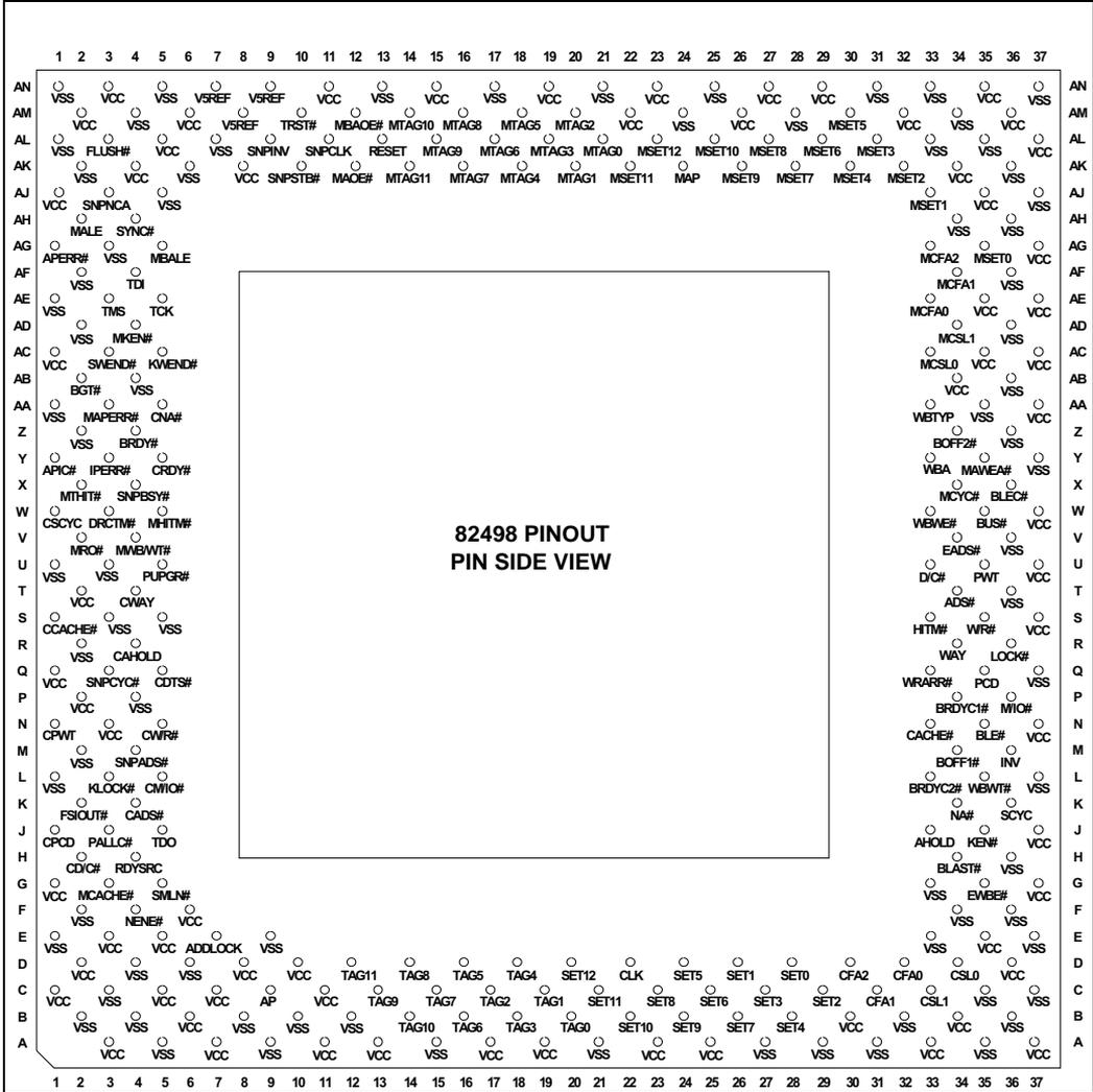
Figure 20-2. 82498 Cache Controller Pinout (Pin View)
