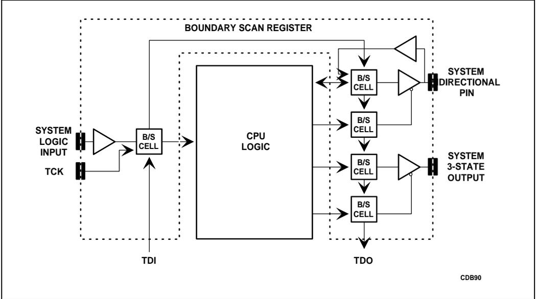
Figure 11-1. Boundary Scan Register Structure of a Component
