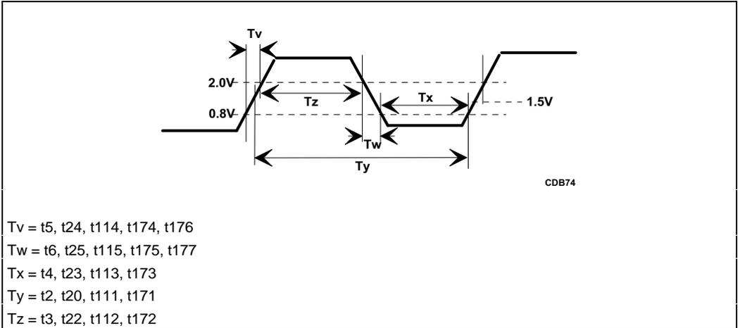
Figure 23-5. Clock Waveform
