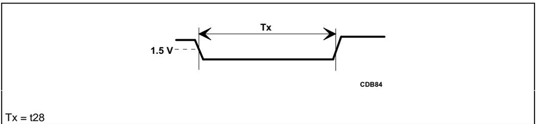
Figure 23-15. Test Reset Timings
