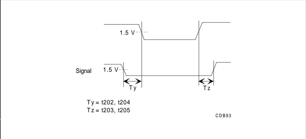
Figure 14-10. Setup and Hold Timings MxST
