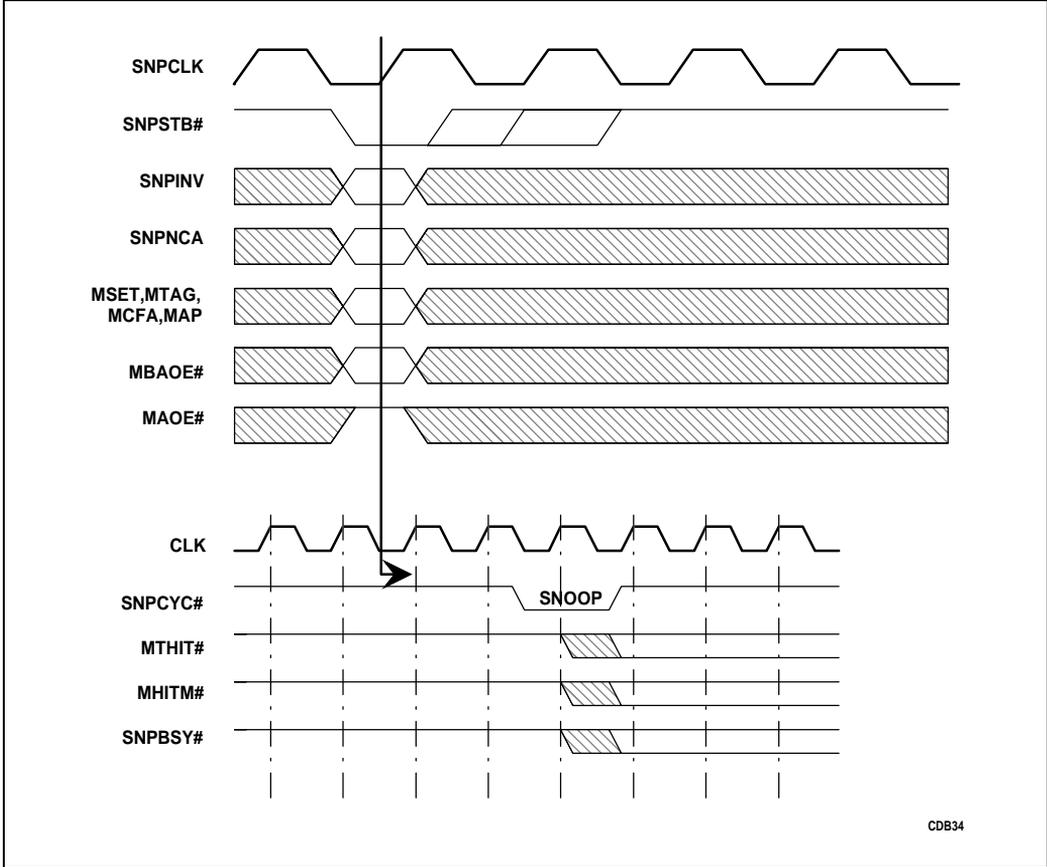
Figure 5-5. Clocked Snoop Mode
