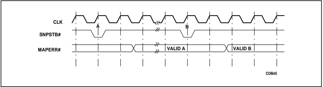
Figure 5-17. MAPERR# Timing for Synchronous Snoop Mode
