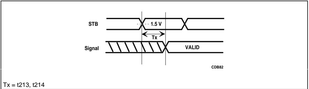
Figure 7-13. Valid Delay Timings from Strobes
