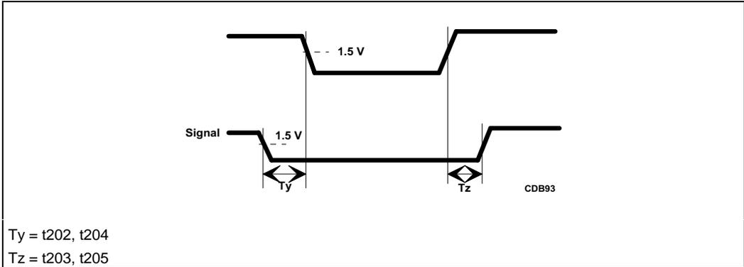
Figure 23-12. Setup and Hold Timings M<sub>x</sub>ST
