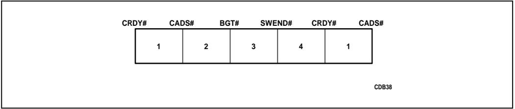
**Figure 5-12. Snoop Response During Cycles**
