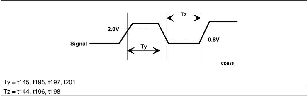
**Figure 23-16. Active/Inactive Timings**
