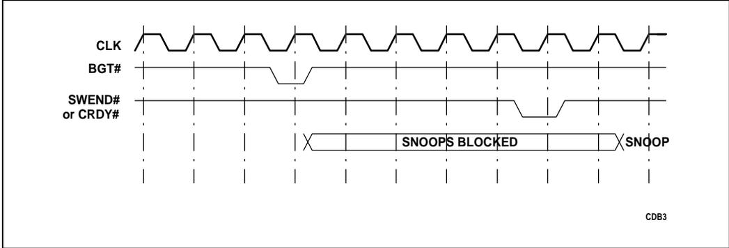
Figure 5-13. Snoop Response Blocking Using BGT#
