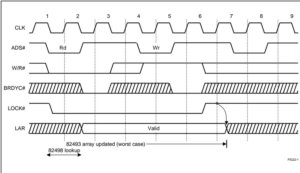
Figure 22-1. Non-Split LOCKed Sequence - Hit to E/M State
