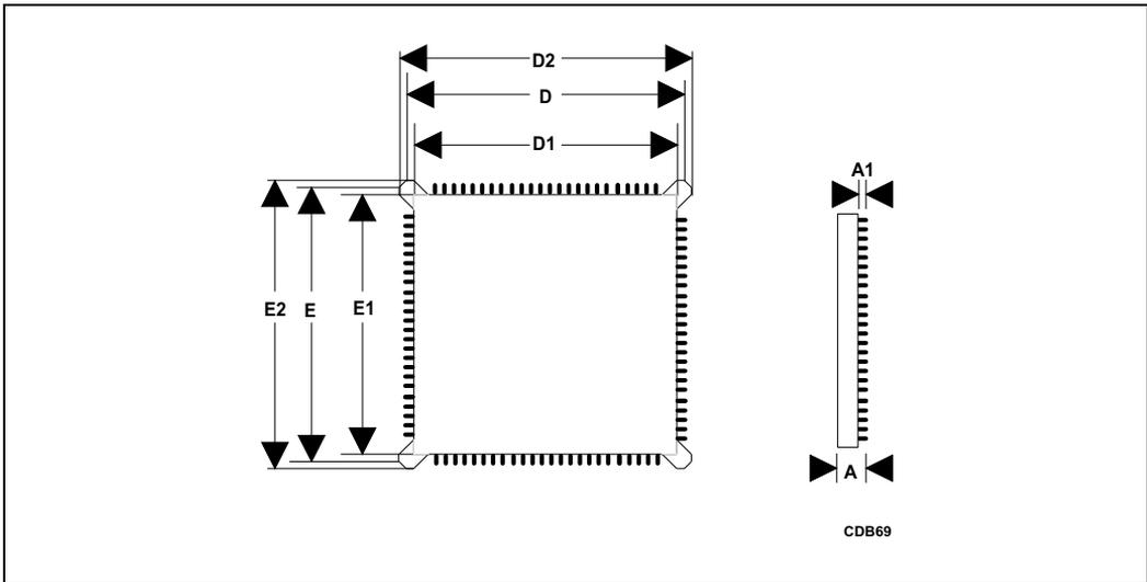
**Figure 25-2. 82493 Cache SRAM Mechanical Specifications**
