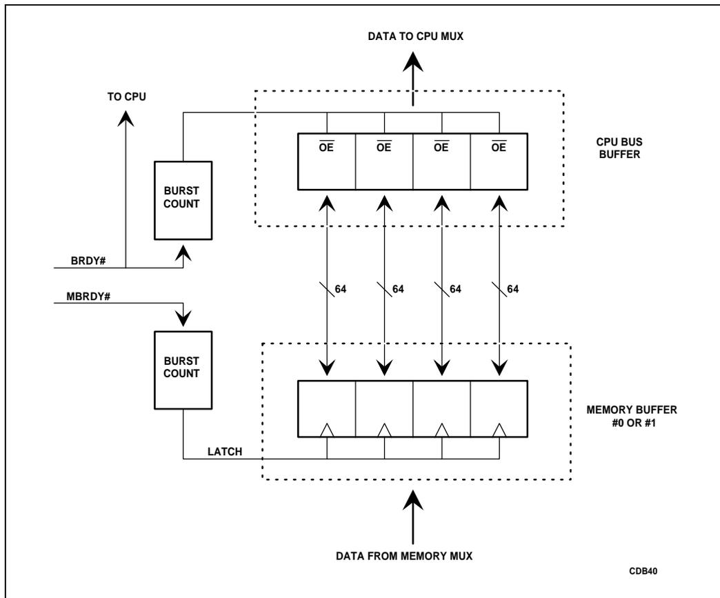
Figure 5-20. 82491 Cache SRAM Read Data Path
