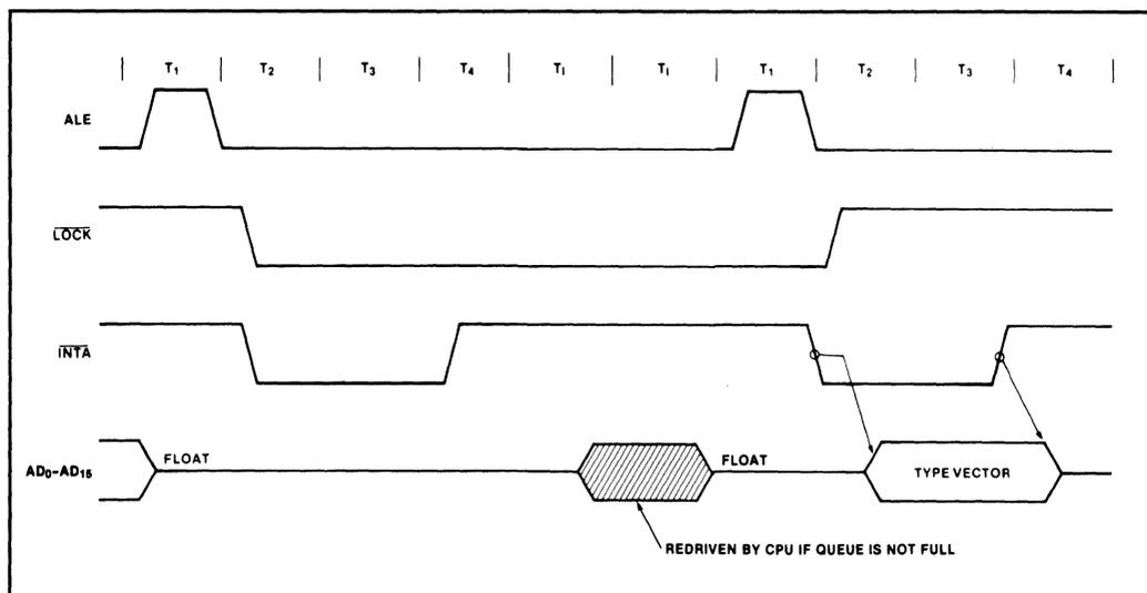
Figure 1-106 Interrupt Acknowledge Timing
