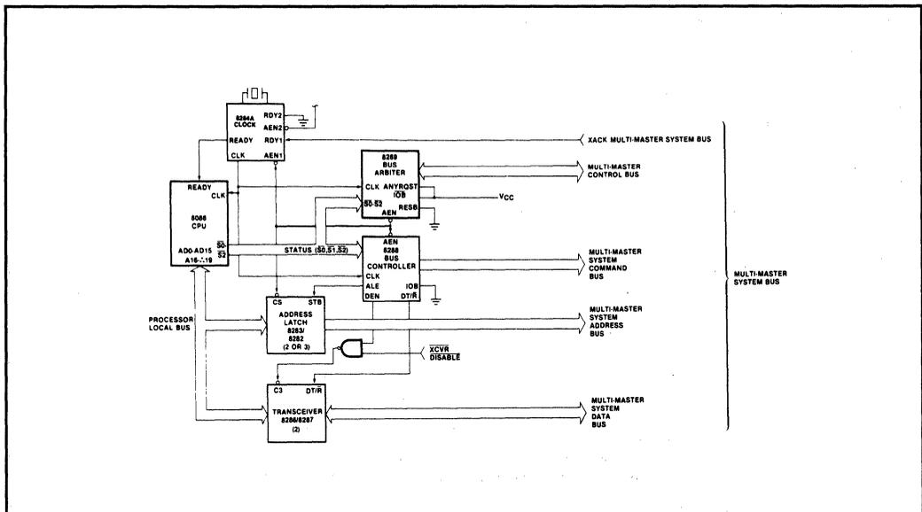
Figure 1-131 Typical Medium Complexity CPU Circuit
