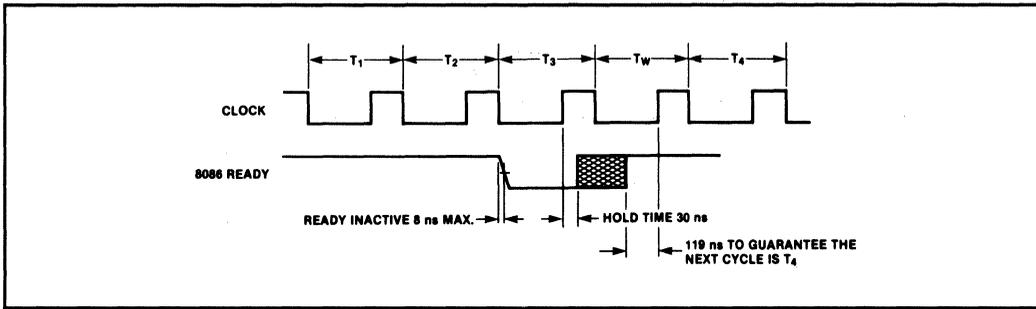
Figure 1-86 Normally Ready System Inserting a Wait State
