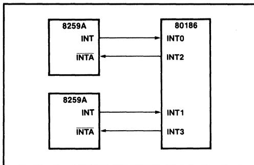
**Figure 2-60 Cascade and Special Fully Nested Mode Interface**
