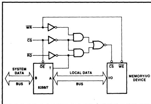
Figure 1-79 Buffering Devices Without OE\*/RD\* and With Common or Separate Input/Output
