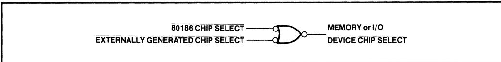
Figure 2-18 80186/External Chip Select/Device Chip Select Generation
