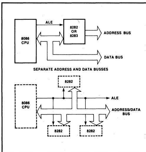
**Figure 1-75 Multiplexed Bus With Local Address Demultiplexing**
