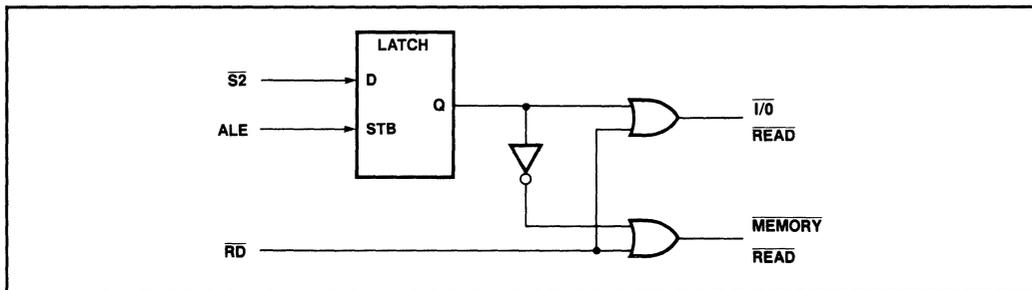
Figure 2-10 Generating I/O and Memory Read Signals
