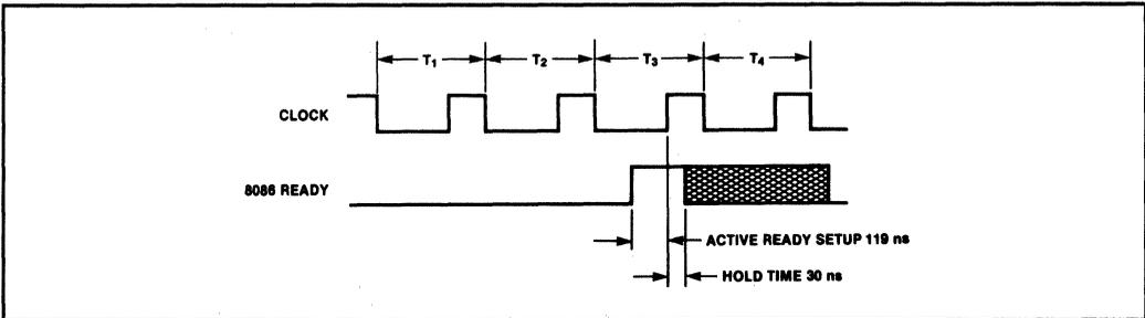
Figure 1-87 Normally Not Ready System Avoiding a Wait State
