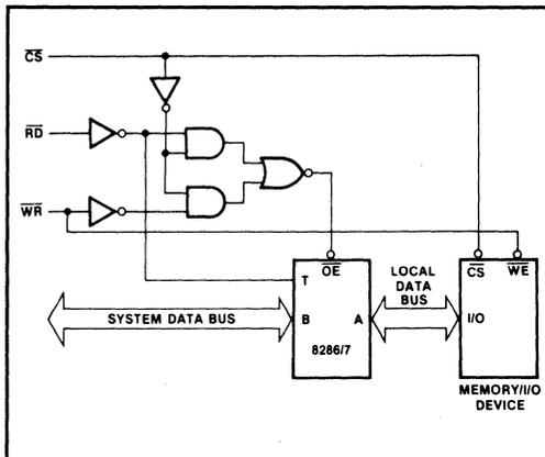
Figure 1-80 Buffering Devices Without OE\*/RD\* and With Common or Separate Input/Output
