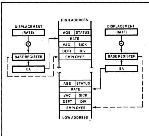
Figure 1-21 Accessing A Structure With Based Addressing
