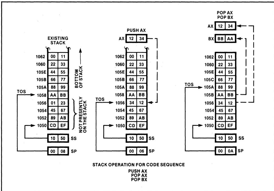
Figure 1-14 Stack Operation
