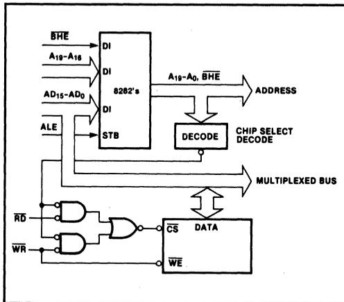
Figure 1-68 Devices Without Output Enable on the Multiplexed Bus
