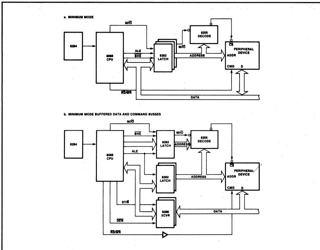
Figure 1-58 8086 System Configurations
