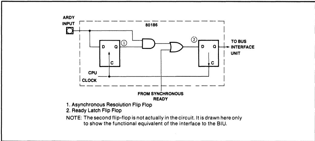
Figure 2-31 Asynchronous Ready Circuits for the 80186
