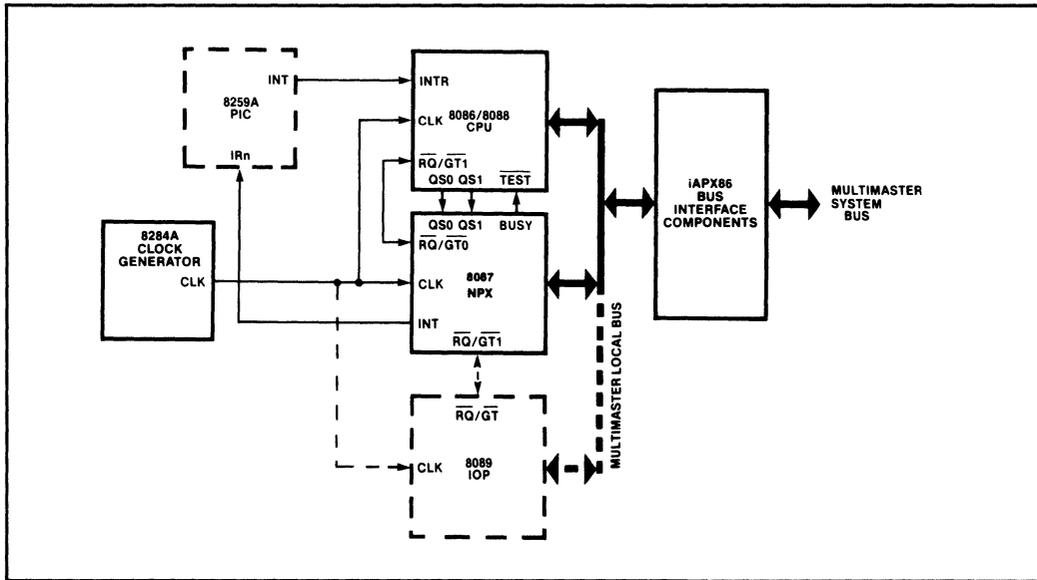
Figure 3-11 8087 NPX — 8086/88 CPU System Configuration
