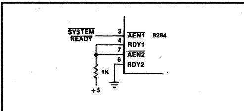
Figure 1-91 Using AEN1\*/AEN2\* to Generate Ready
