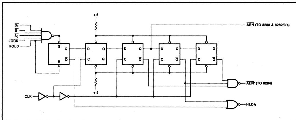
Figure 1-101 Circuit to Translate HOLD into AEN Disable for Maximum Mode 8086/88
