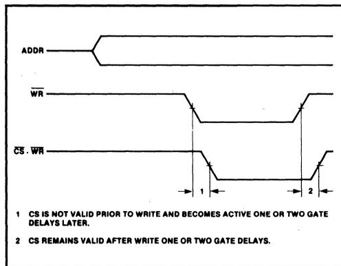
Figure 1-70 CE to WR\* Setup and Hold
