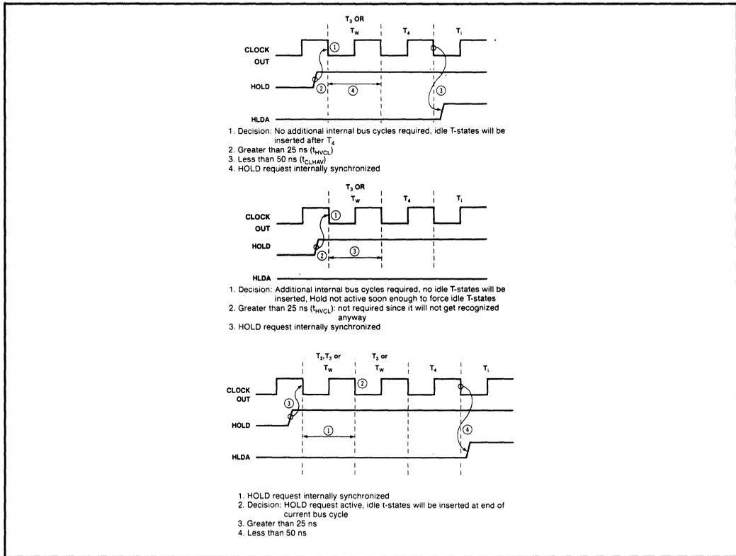
Figure 2-36 HOLD/HLDA Timing
