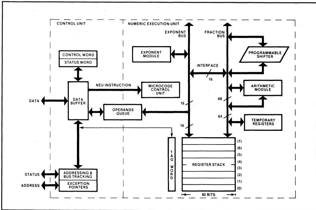
**Figure 3-7 8087 Numeric Processor Extension Block Diagram**
