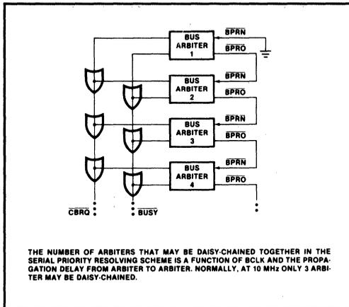
Figure 1-130 Serial Priority Resolving.
