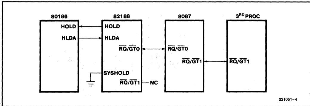
Figure 3-12 8087 NPX — 80186/188 CPU System Configuration
