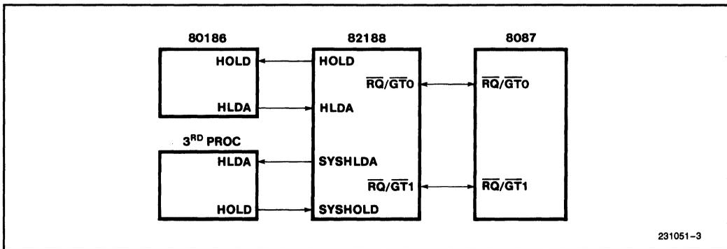
Figure 3-14 Three Processor System Bus Signal Connections
