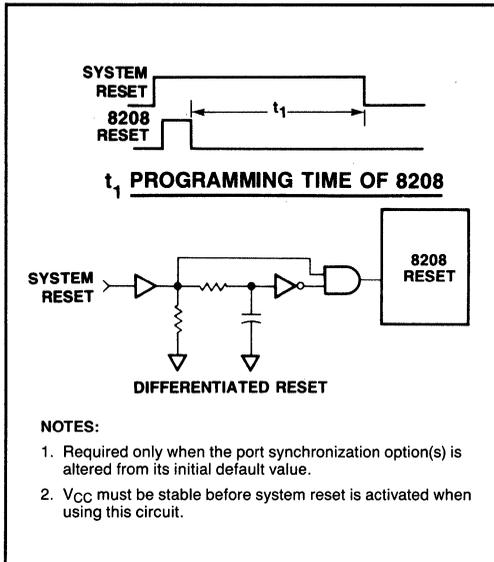
Figure 2-25 8208 Differentiated Reset Circuit
