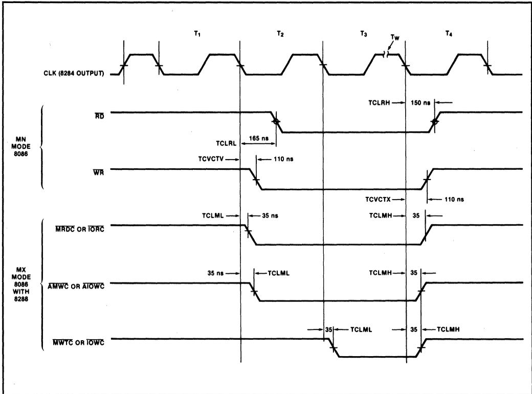
Figure 1-126 Maximum and Minimum Mode Command Timing
