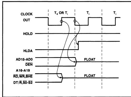
**Figure 2-34 Signal Float/HLDA Timing**
