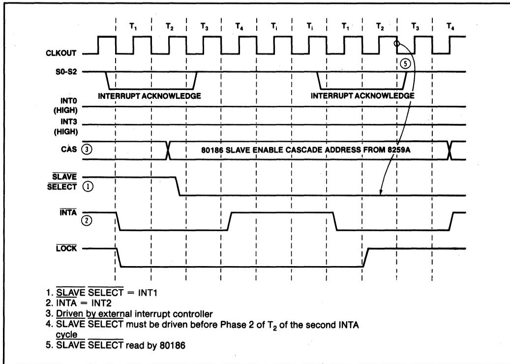
Figure 2-65 80186 iRMX™ 86 Mode Interrupt Acknowledge Timing
