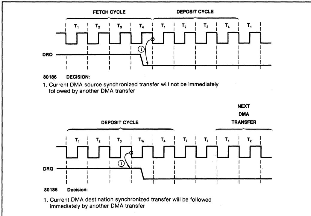
Figure 2-45 Source & Destination Synchronized DMA Request Timing
