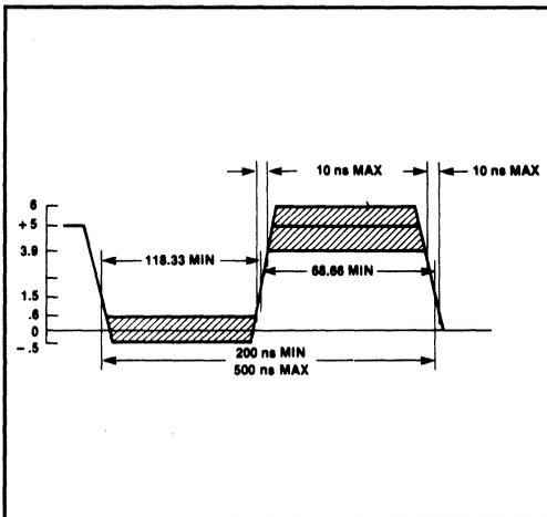
Figure 1-110 8086/88 Clock Waveform
