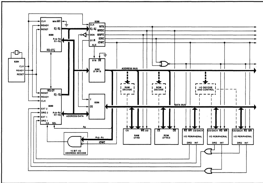
Figure 4-10 iAPX 86/11, 88/11 Configuration with 8089 in Local Mode
