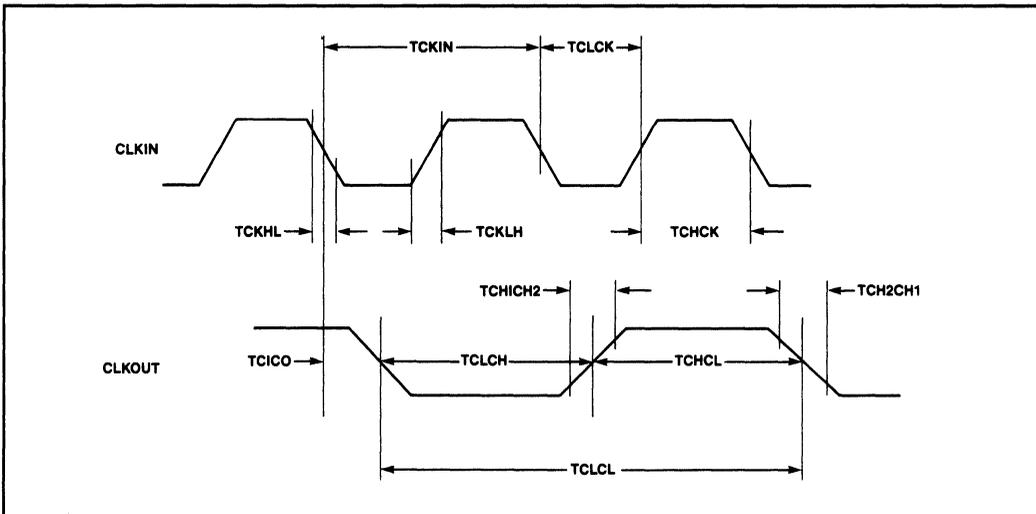
Figure 2-73 Clock In/Clock Out Timing
