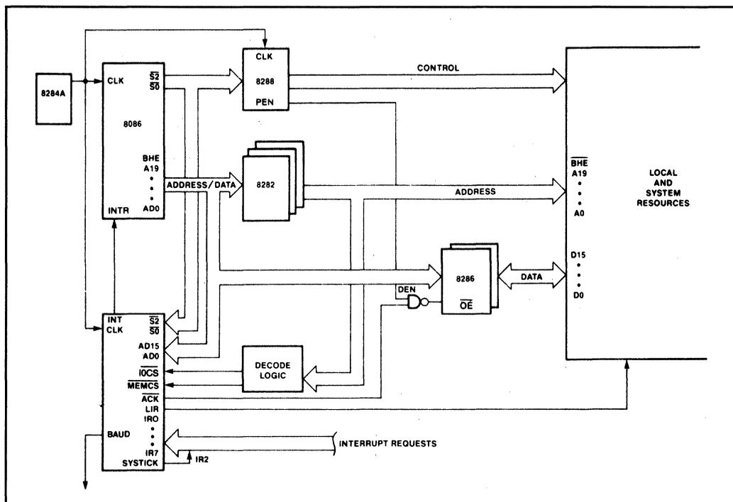
Figure 5-3 OSP Typical Configuration With An 8086
