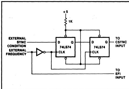
**Figure 1-115 Synchronizing CSYNC With EFI**
