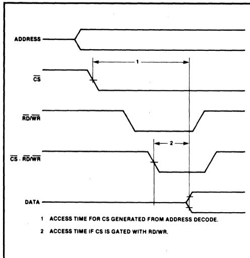
Figure 1-69 Access Time: CS Gated with AD\*/WR\*
