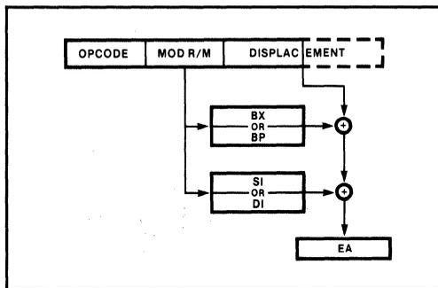
Figure 1-24 Based Index Addressing
