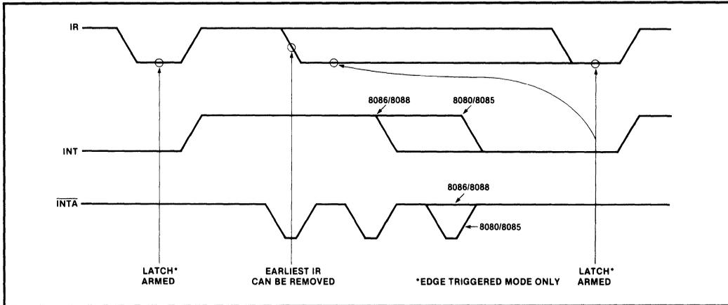
Figure 1-137 IR Triggering Timing Requirements
