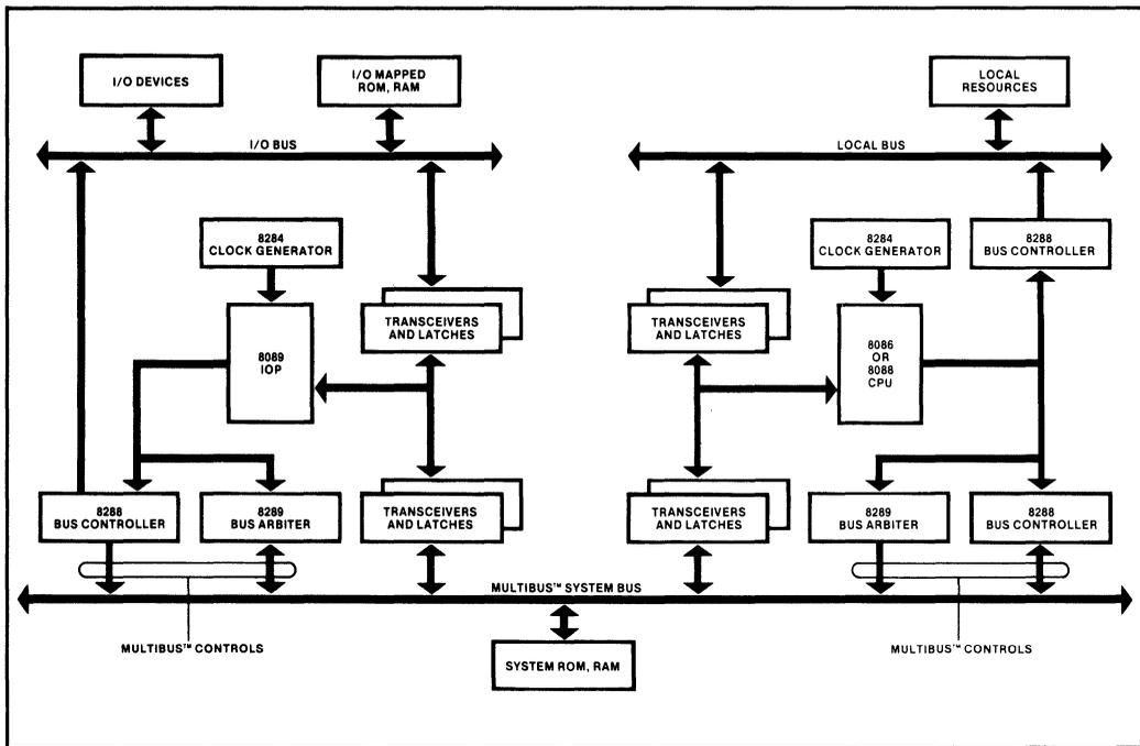
Figure 1-2 8086/8088/8089 Multiprocessing System
