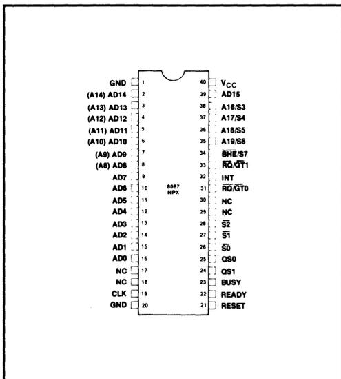
Figure 3-2 8087 Numeric Data Processor Pin Diagram
