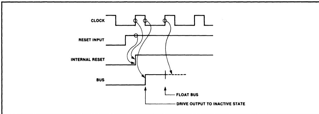
Figure 1-102 8086/88 Bus Conditioning on Reset Timing Diagram
