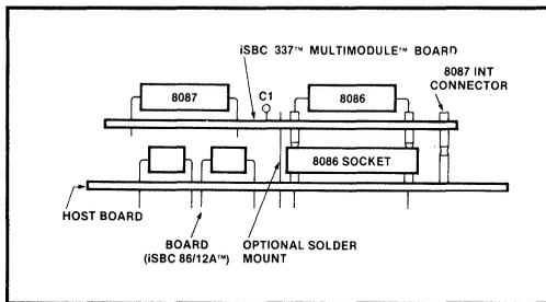
**Figure 3-6 iSBC® 337 MULTIMODULE Mounting Scheme**
