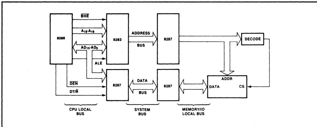
Figure 1-76 Fully Buffered System
