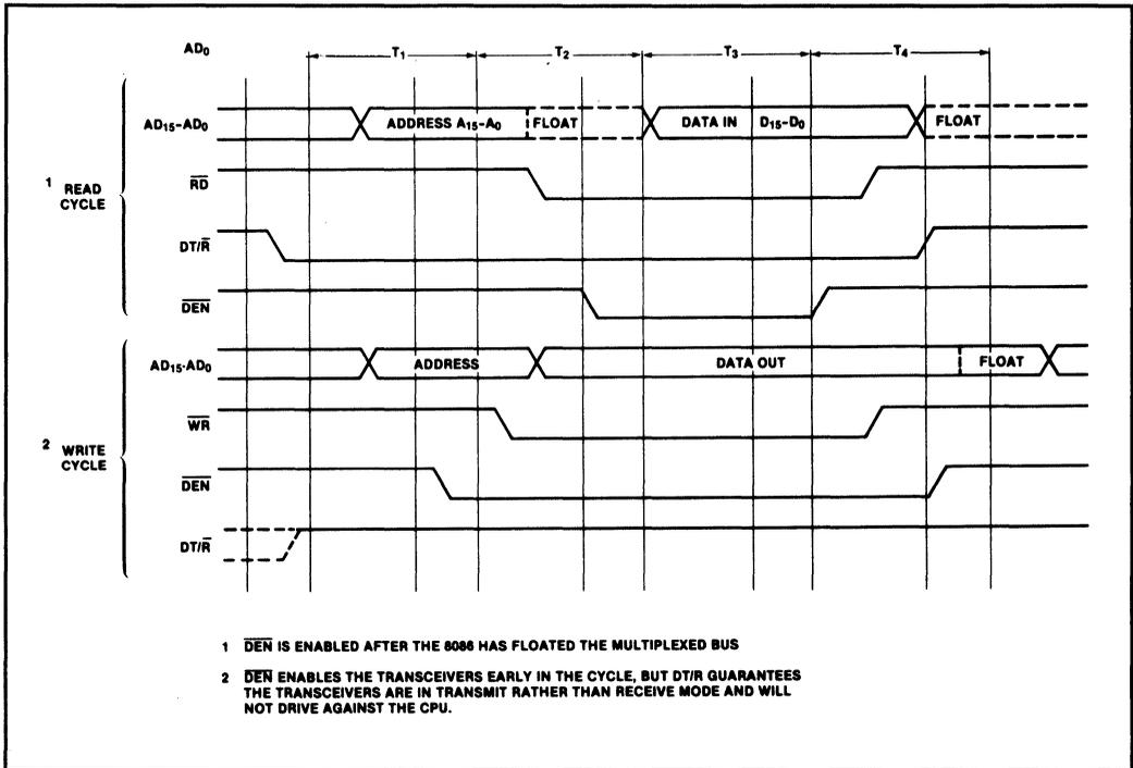
Figure 1-71 Bus Transceiver Control
