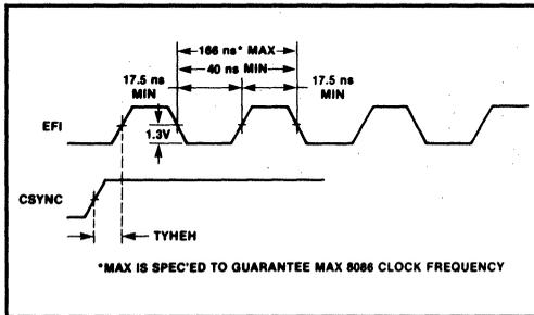
**Figure 1-116 CSYNC Setup and Hold to EFI**
