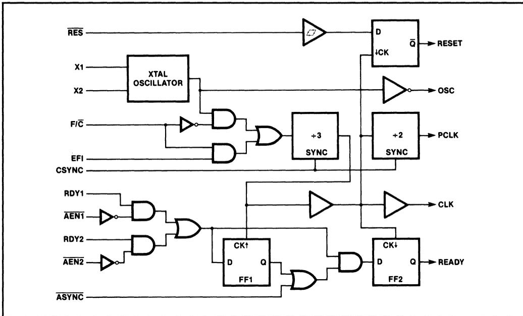
Figure 1-109 8284A Clock Generator/Driver Block Diagram
