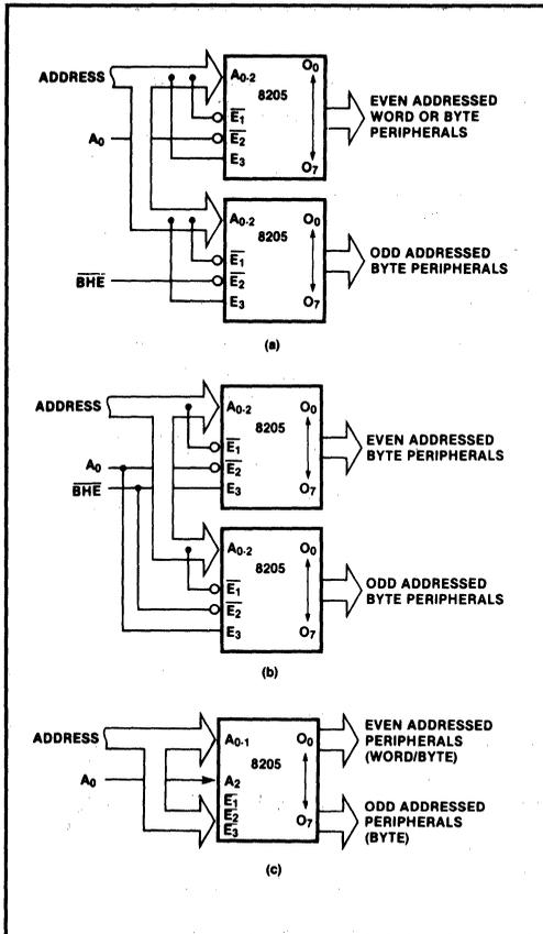
Figure 1-54 I/O Device Chip Select Techniques
