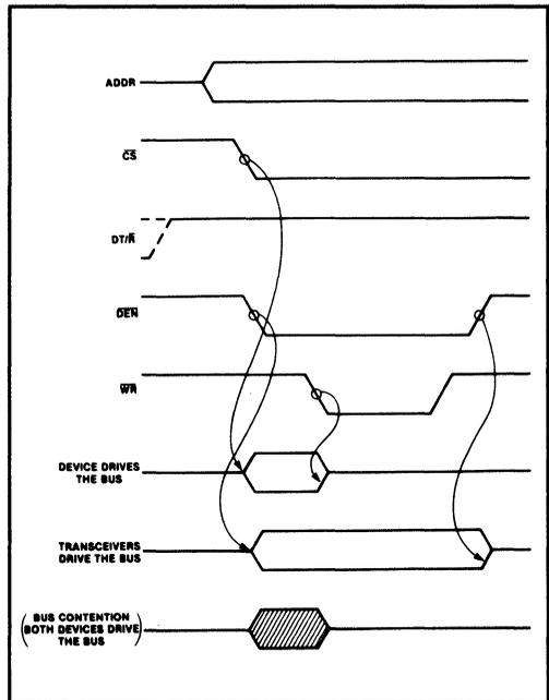
Figure 1-73 CS\*/Bus Driving Device Timing
