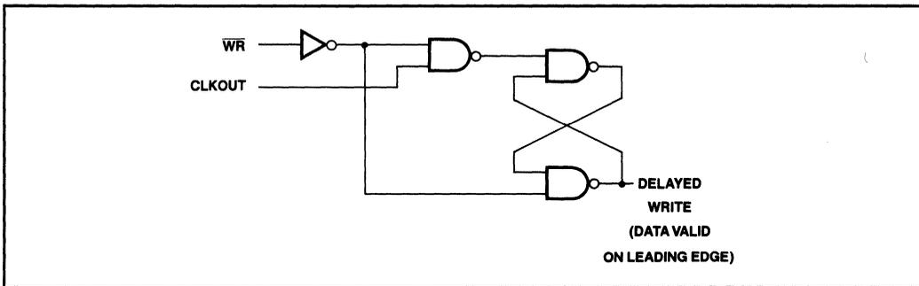
Figure 2-12 Synthesizing Delayed Write from the 80186
