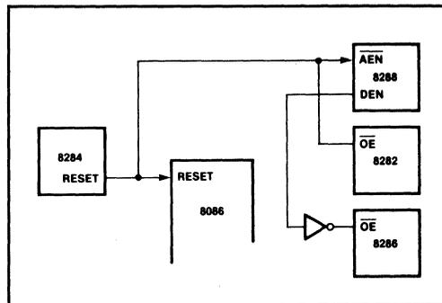
Figure 1-103 Reset Disable for Max Mode 8086/8088 Bus Interface
