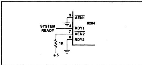
Figure 1-90 Using RDY1/RDY2 to Generate Ready
