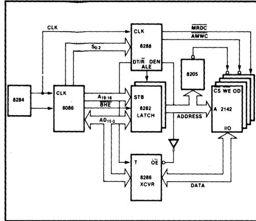
Figure 1-50 Sample Compatibility Analysis Configuration
