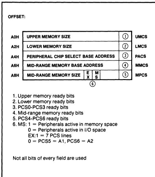
Figure 2-68 80186 Chip Select Control Registers
