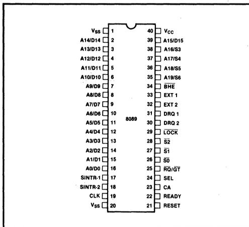
Figure 4-7 8089 I/O Processor Pinout Diagram
