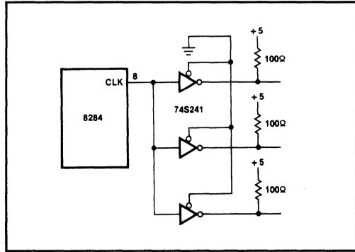
Figure 1-119 Buffering the 8284 CLK Output
