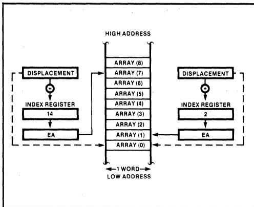
Figure 1-23 Accessing an Array With Indexed Addressing
