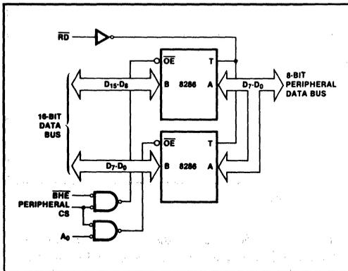
Figure 1-55 16-bit to 8-bit Bus Conversion
