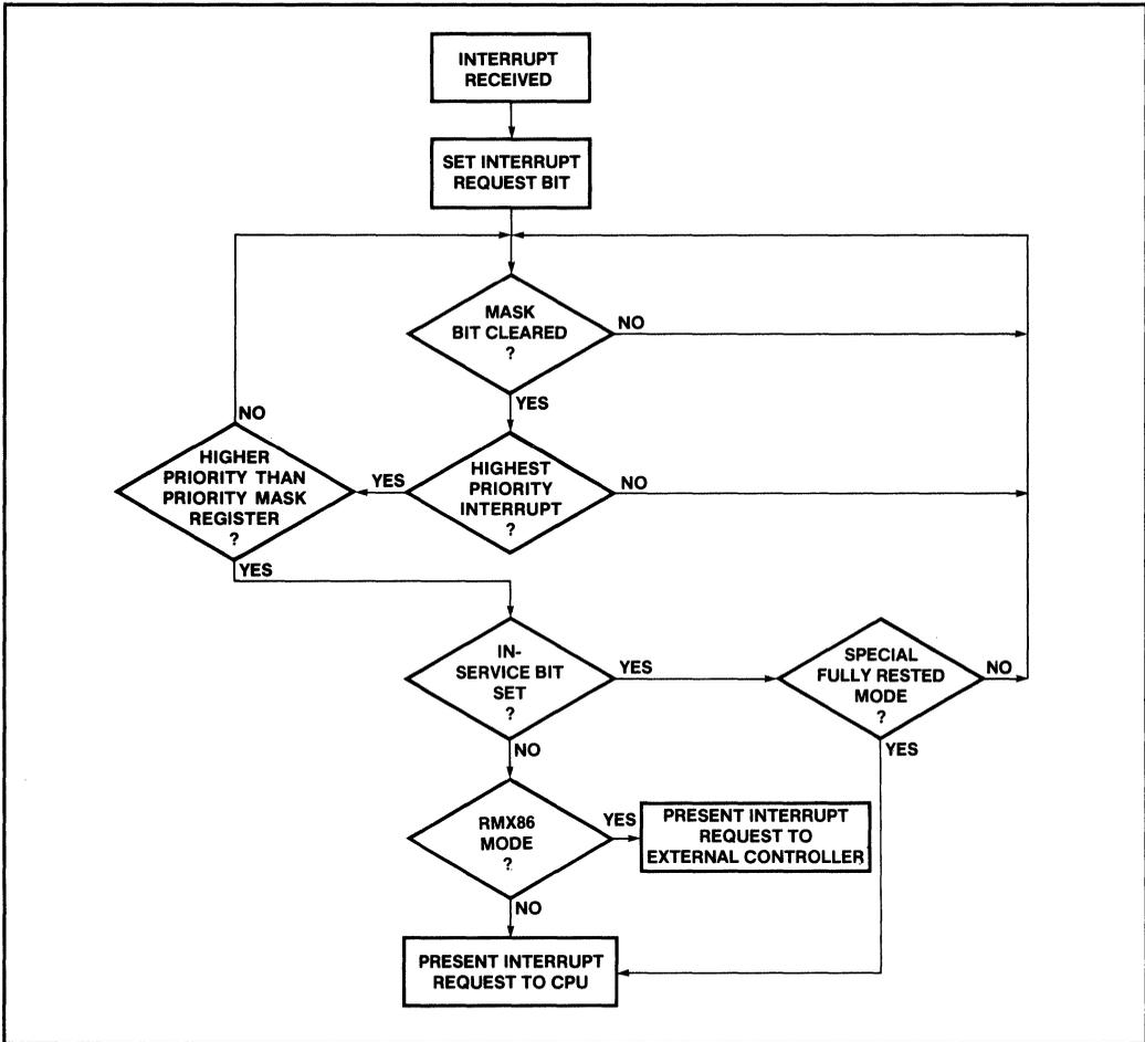
Figure 2-57 80186 Interrupt Sequencing
