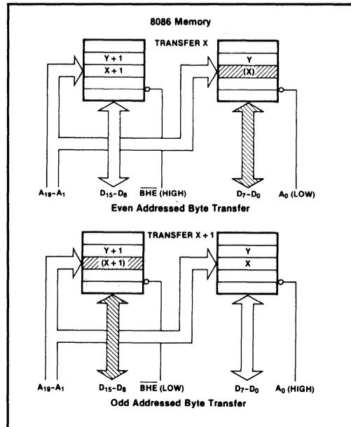
Figure 1-42 Memory Even and Odd Data Byte Transfers
