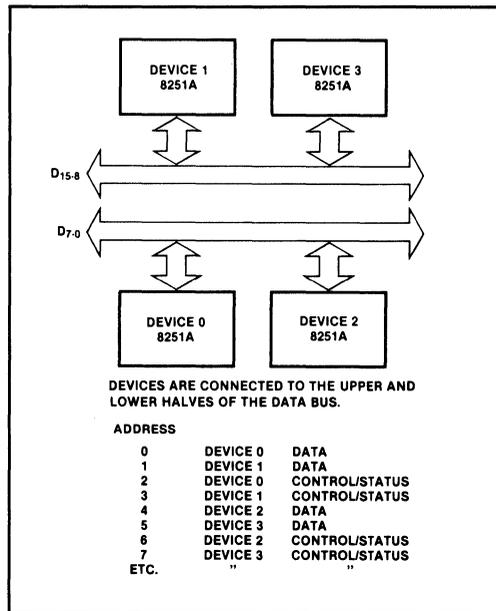
**Figure 1-59 Device Assignment**
