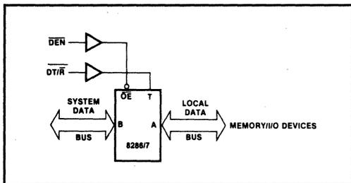
Figure 1-77 Controlling System Transceivers with DEN and DT/R\*
