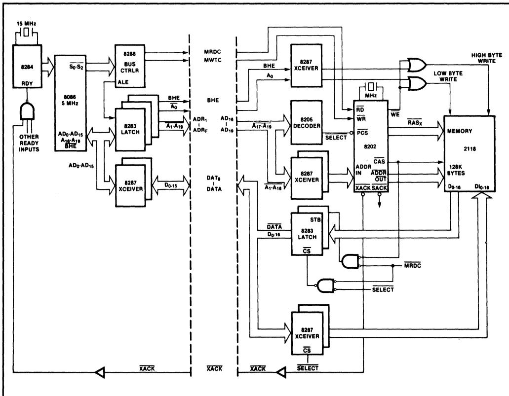
Figure 1-51 5 MHz 8086 System Using an 8202 Dynamic RAM Controller
