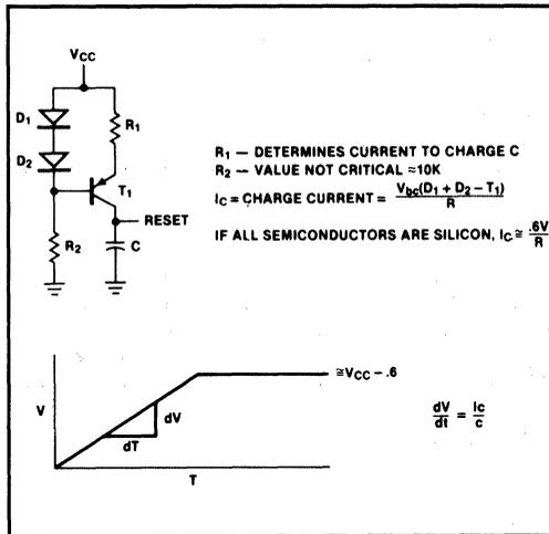
Figure 1-122 Constant Current Power Up Reset Circuit
