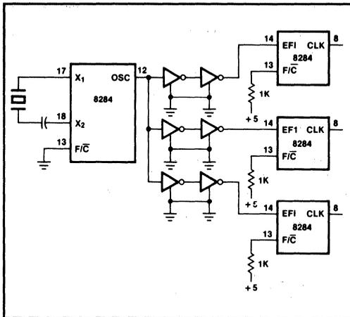
**Figure 1-113 External Frequency for Multiple 8284's**
