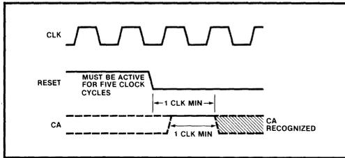
Figure 4-12 RESET-CA Initialization Timing
