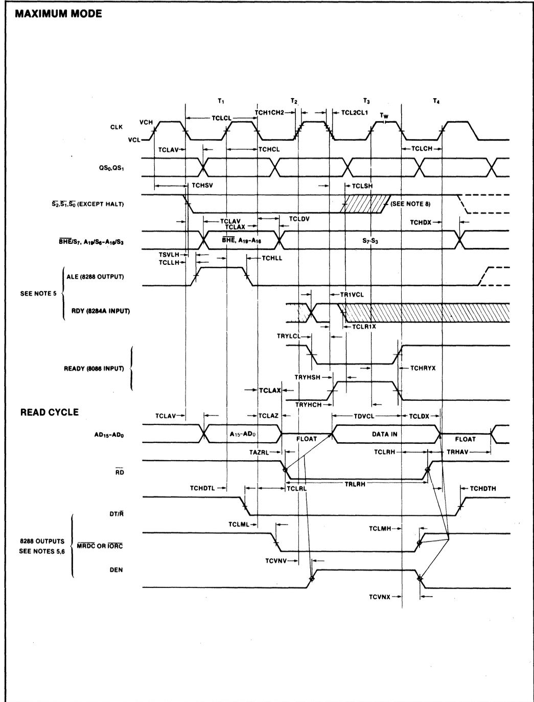
Figure 1-32 Maximum Mode Waveforms
