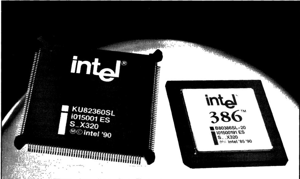
**Figure 1-2. The Intel386™ SL Microprocessor SuperSet Includes Two Highly-Integrated Components**
