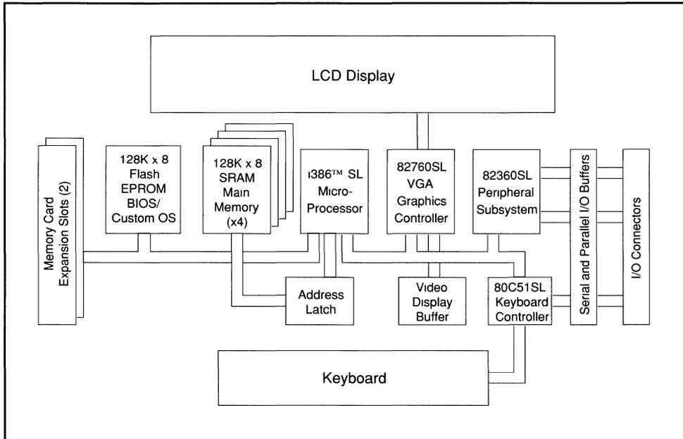
**Figure 5-1. Ten-Chip Palm-Top PC Block Diagram**
