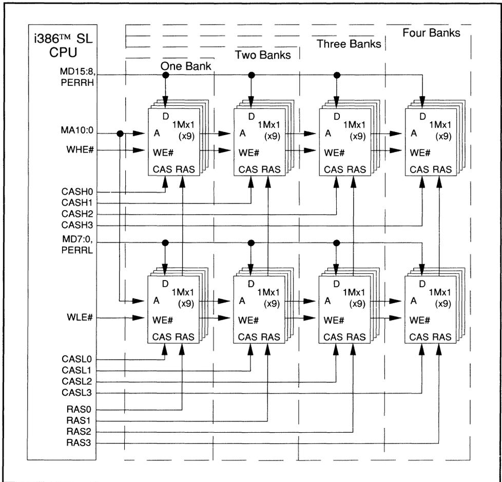
**Figure 2-4. Four-Bank, 32-Megabyte Dynamic RAM Memory Configuration**
