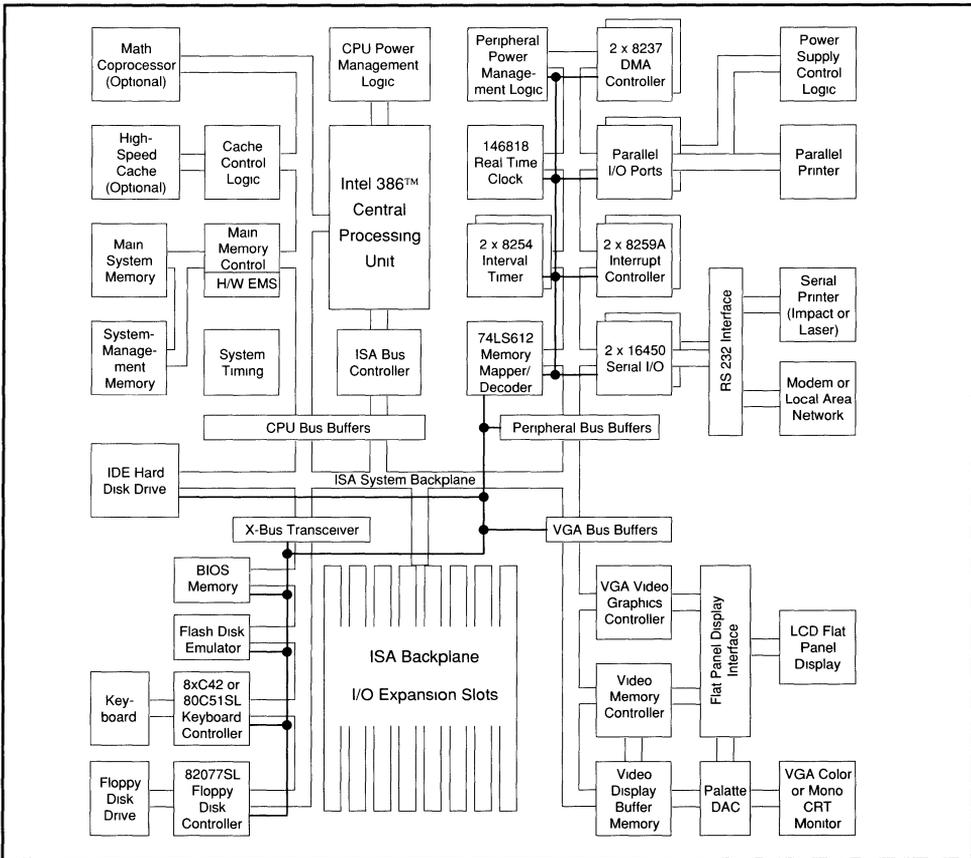
**Figure 1-1. Industry-Standard PCs Contain a Common Set of System Functions and Peripherals**
