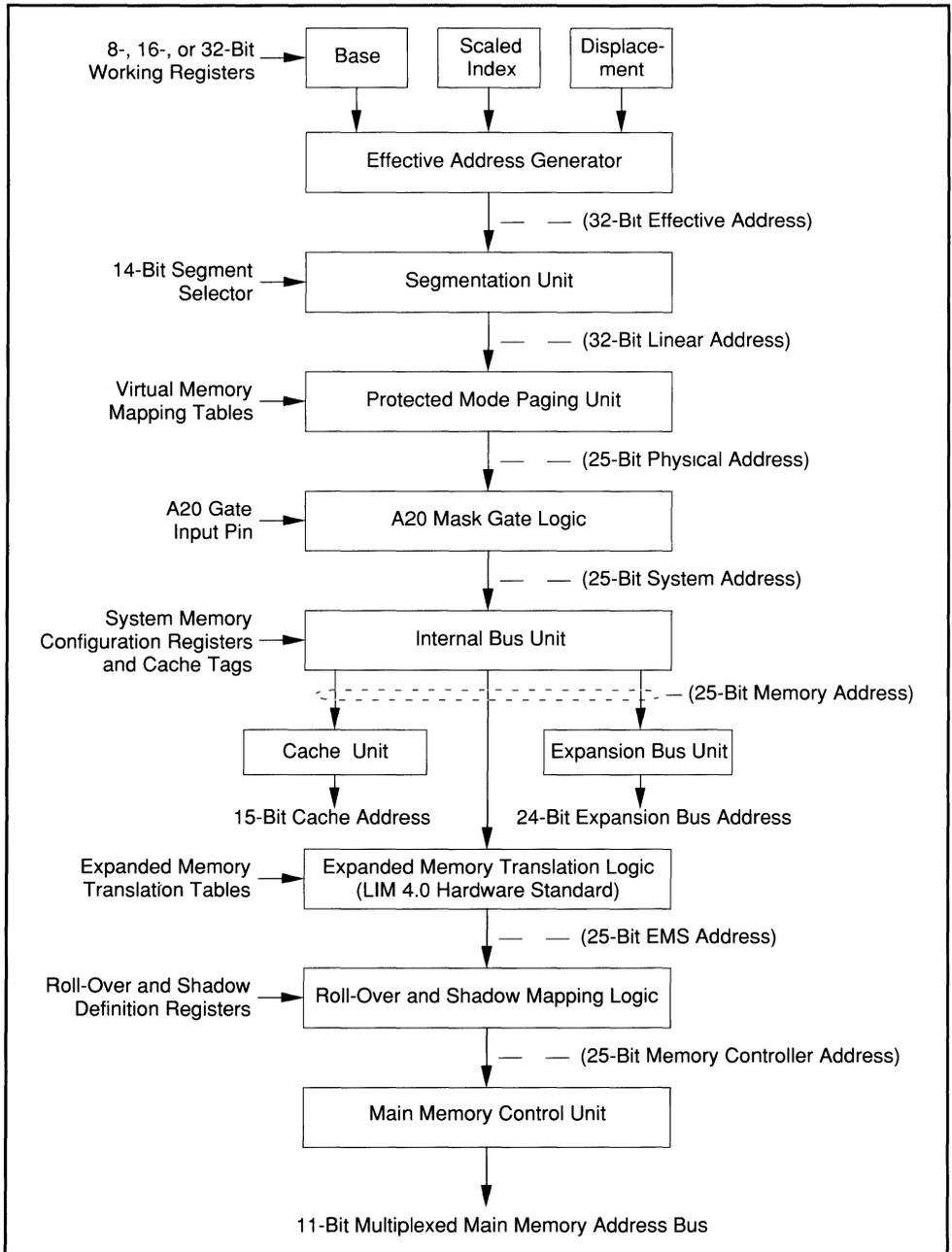
**Figure 3-1. Intel386™ SL Processor Memory Address Translation Logic Eliminates External Propagation Delays**
