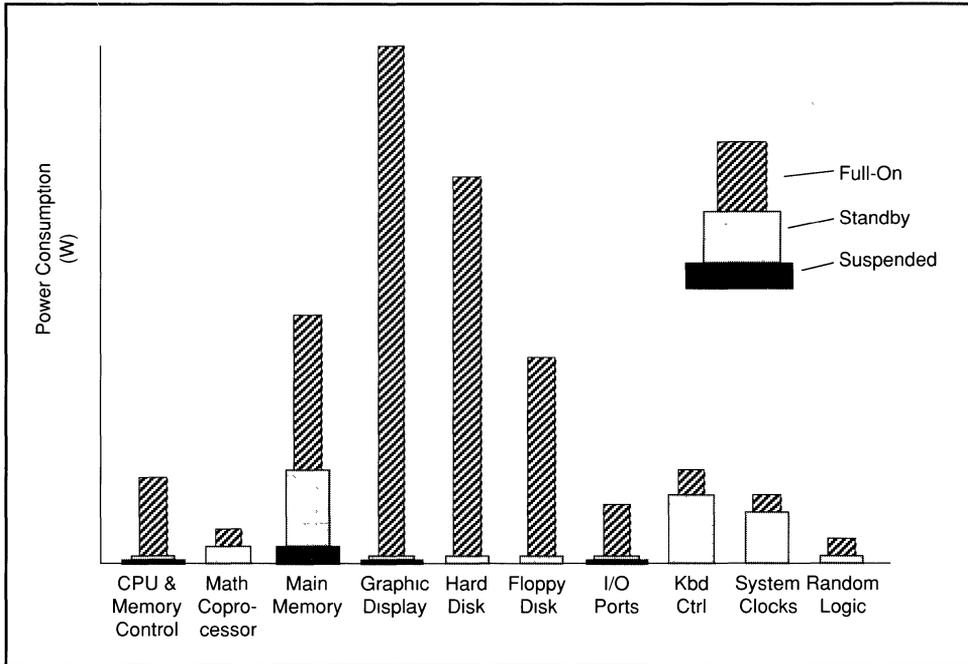
**Figure 4-1. Lap-Top System Power Consumption Varies Greatly Depending on Operating Mode**
