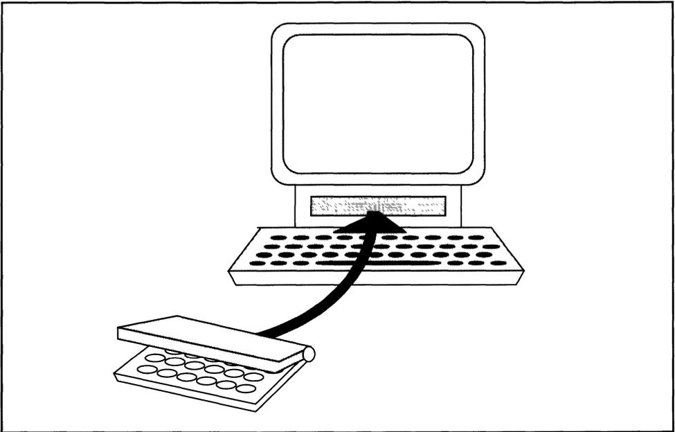
**Figure 1-6. Stand-Alone Portable Module Acts as the Compute Engine of a Hybrid PC Design**
