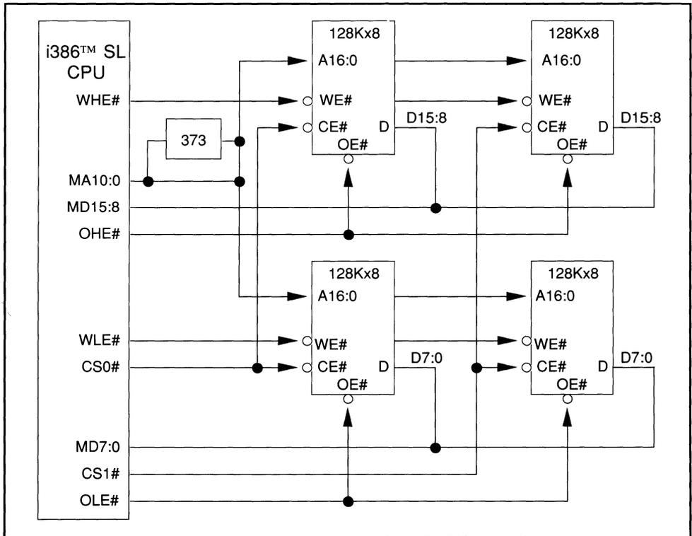
Figure 2-2. 512K-Byte Static RAM Memory Array Connects Directly to the Intel 386™ SL CPU
