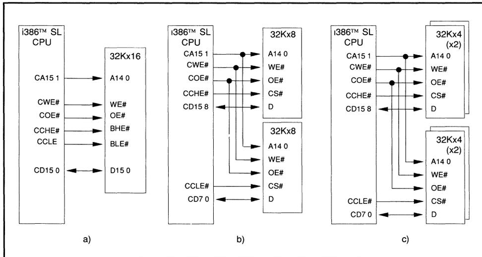
**Figure 2-5. Optional High-Speed Caches Requires (a) One, (b) Two, or (c) Four External Chips**
