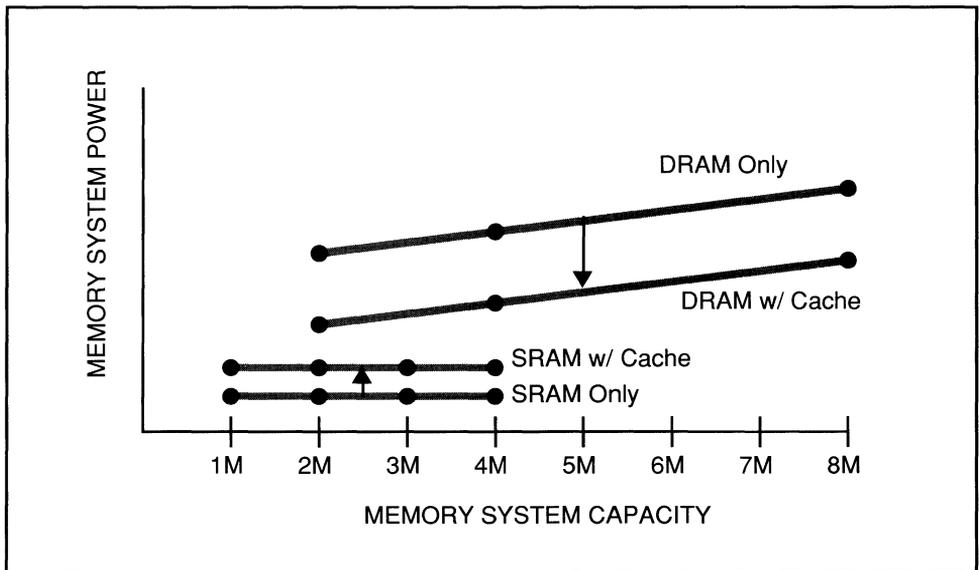
**Figure 2-8. Adding Cache Memory Can Reduce Total System Power Consumption**
