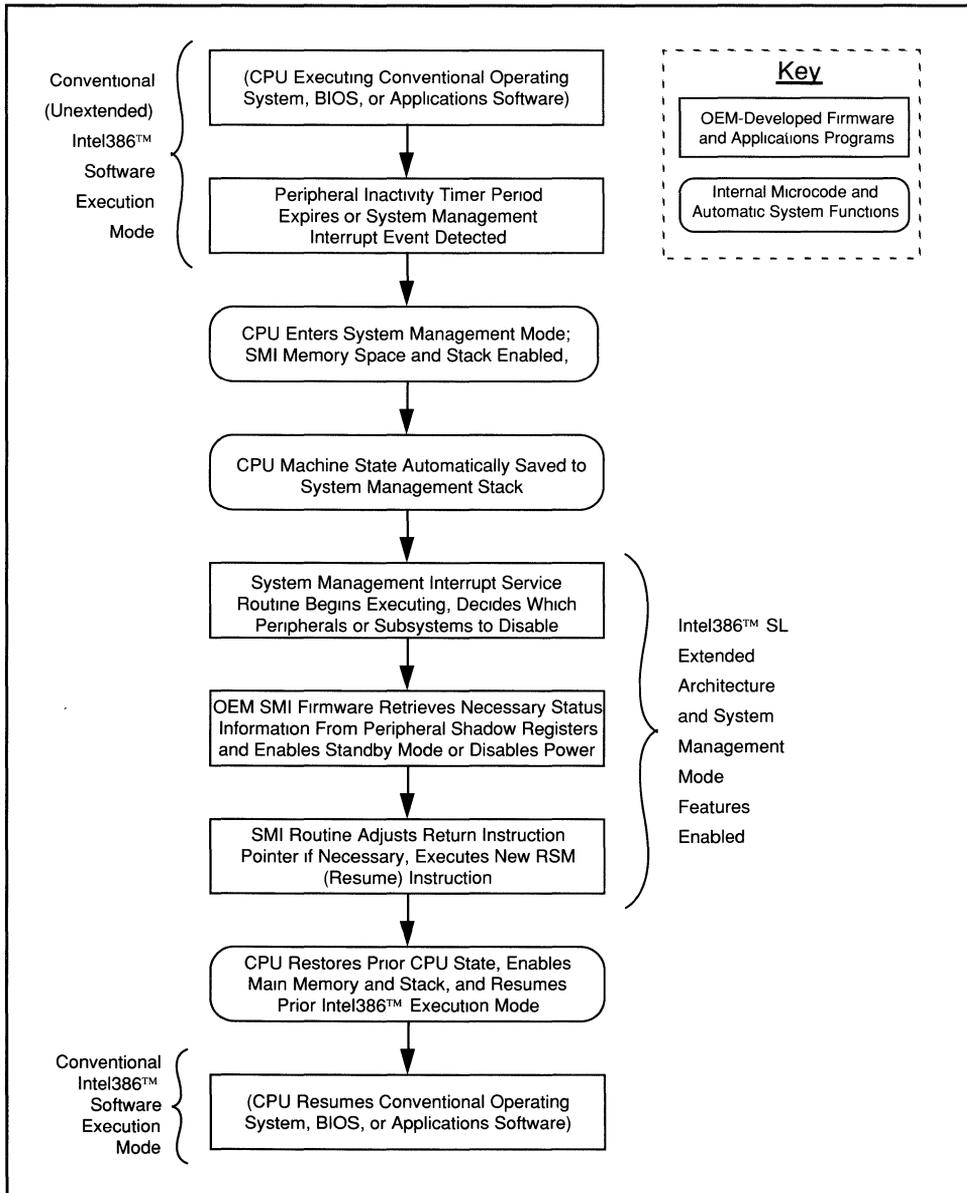
**Figure 4-5. System Management Interrupt Service Routine to Disable Peripheral Power**
