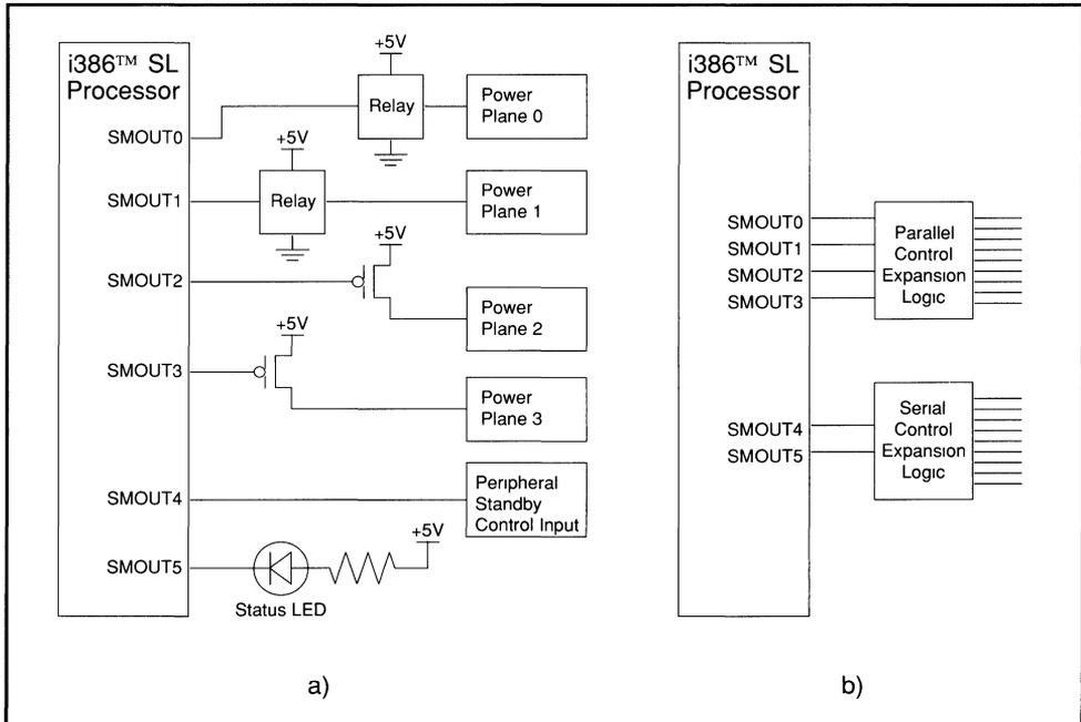
**Figure 4-2. The ideaPort Interface Supports Multiple Power Control Options: a) Direct Peripheral Device Control; b) Parallel and Serial Control Expansion**
