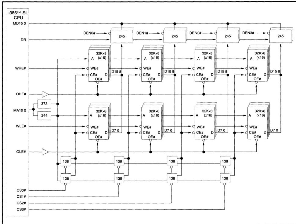
**Figure 2-3. Typical Four-Bank, 4-Megabyte Buffered SRAM Memory Configuration**
