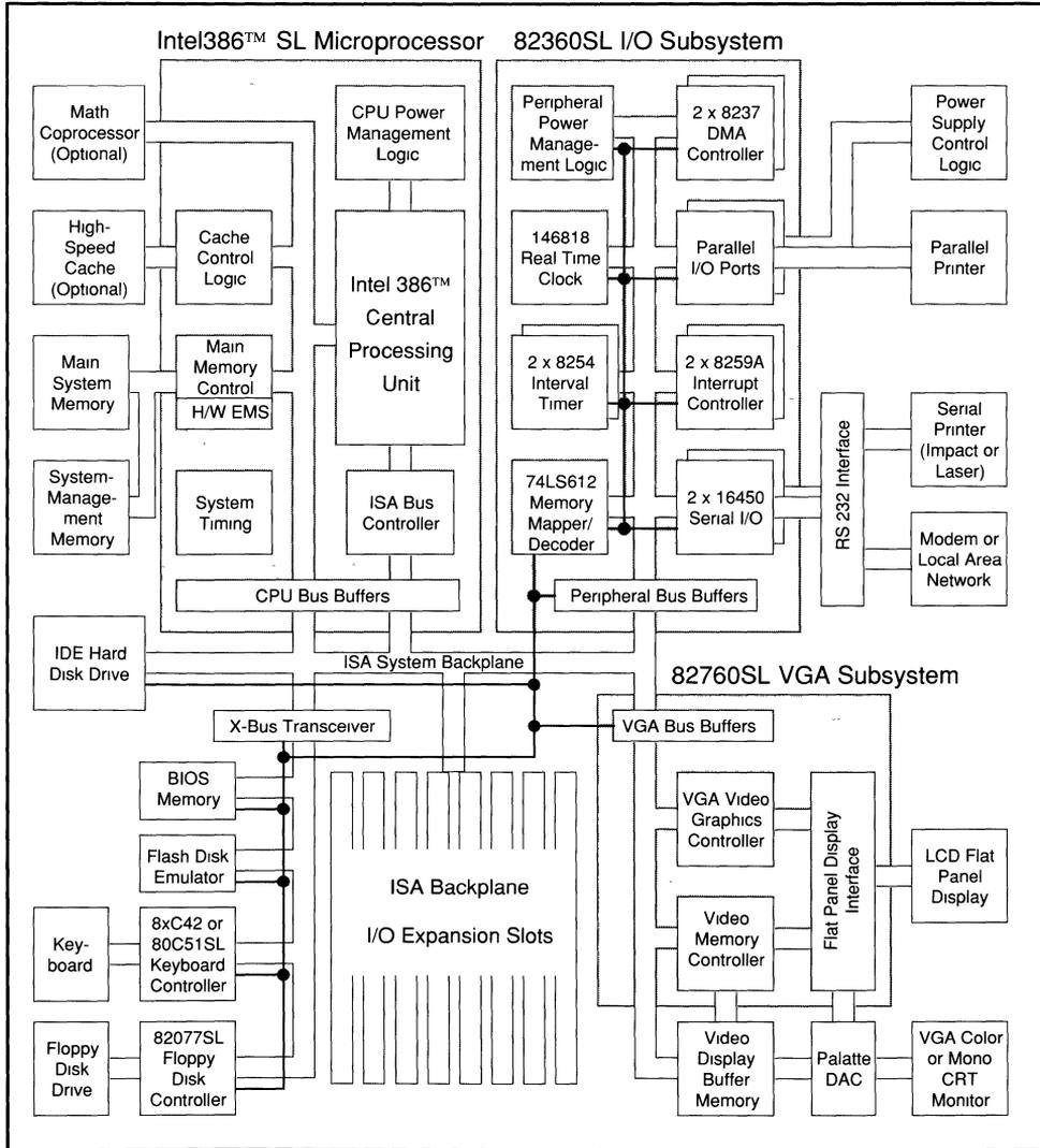
**Figure 2-1. Intel 386™ SL Microprocessor SuperSet Family Components Bring Together All Critical PC Functions**
