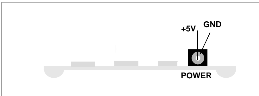
Figure 2-7. Power Supply Polarity
