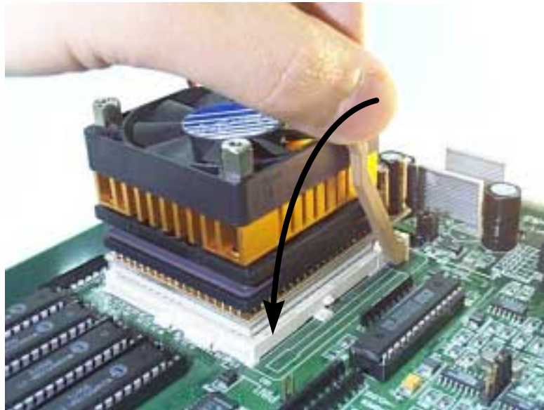
Figure 8. Locking the CPU upgrade board into the ZIF socket
