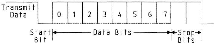
Data bit 0 is the first bit to be transmitted. The interface automatically inserts the start bit, and two stop bits.
