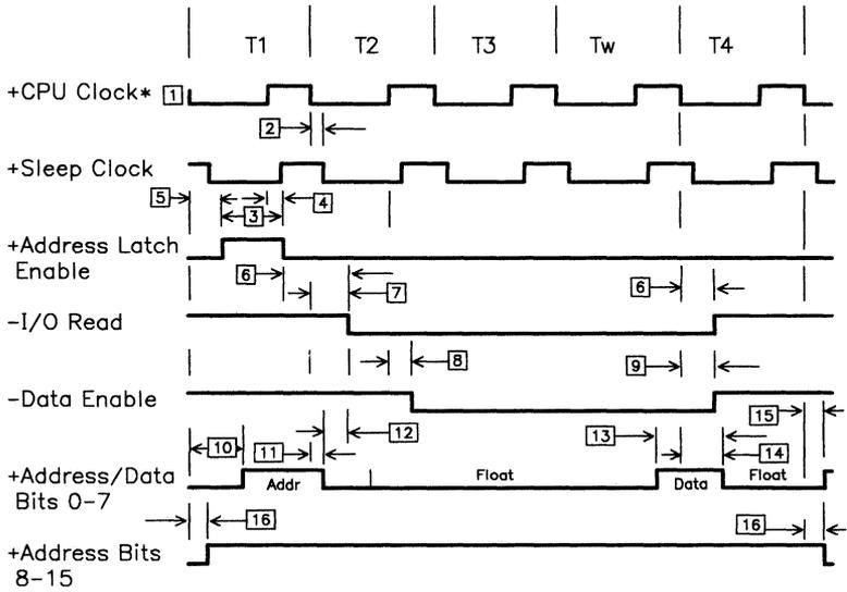
**Figure C-5 (Part 2 of 2). I/O Interface, Processor I/O Read**
