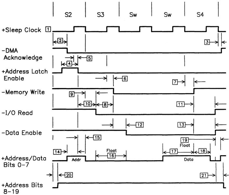
**Figure C-4 (Part 2 of 2). I/O Interface, DMA from I/O to Memory**
