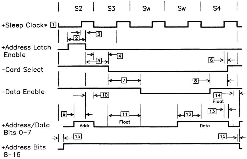
**Figure C-9 (Part 2 of 2). Memory Interface, DMA Read**
