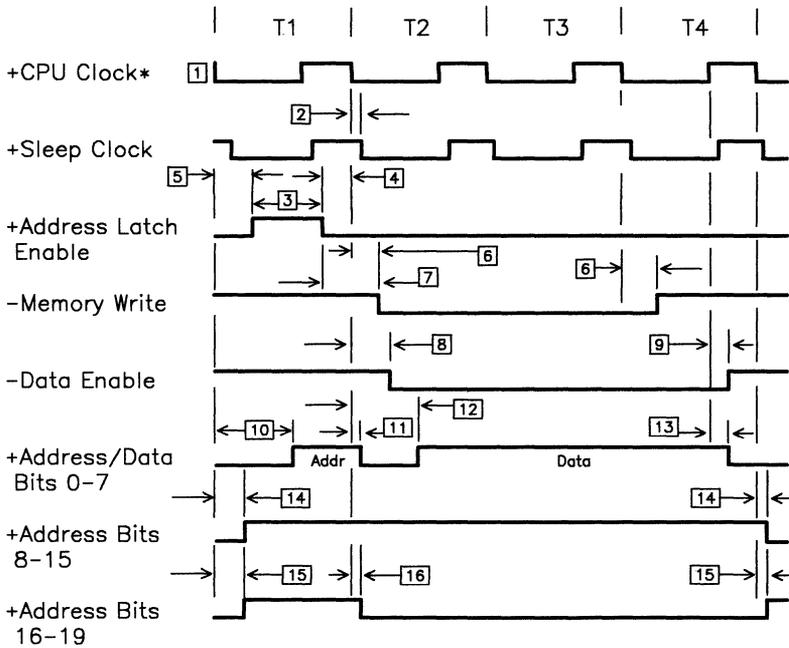
**Figure C-2 (Part 2 of 2). Interface, Processor Memory Write**
