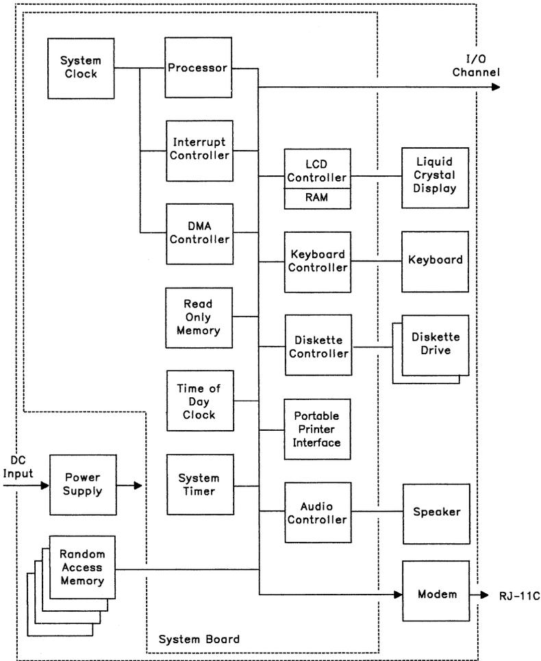
**Figure 2-1. IBM PC Convertible System Unit Functional Units**
