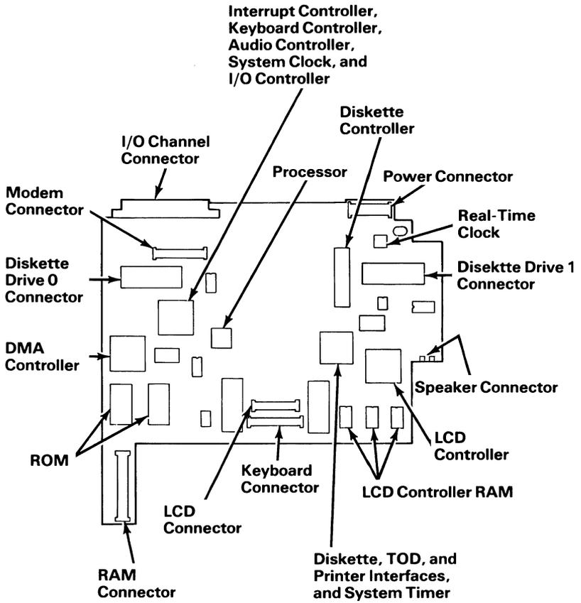
Figure 2-2. System Board Components
