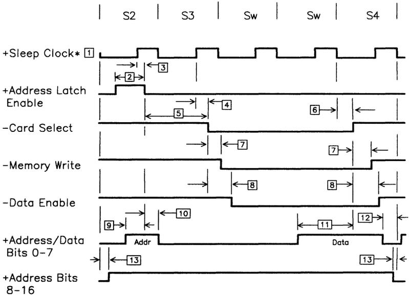
**Figure C-10 (Part 2 of 2). Memory Interface, DMA Write**
