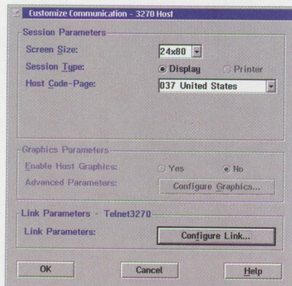
Figure 12. Customize Communication - 3270 Host Window
