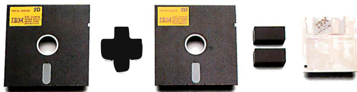
It takes two 360KB 5¼" diskettes to hold as much as one 720KB 3½" diskette.
