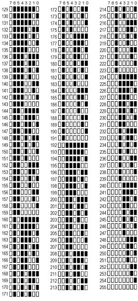
$\blacksquare$  = JUMPER INSTALLED  $\square$  = NO JUMPER
