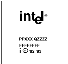
mcB1-Step Engineering Sample TCP Units:
