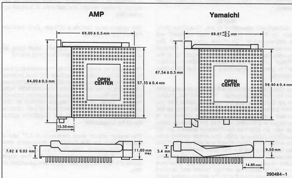
Figure 2-1. OverDrive™ Socket Footprint Dimensions
