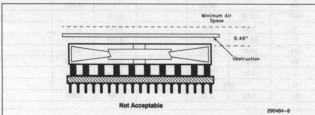
Figure 5-2. Active Heat Sink Top Space Requirements
